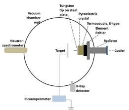
Figure 2. The scheme of the experimental setup.
