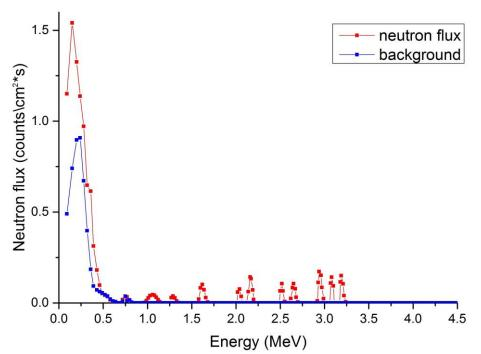
**Figure 3.** The total neutron flux related to energy during the cooling phase within ten thermal cycles (1500 s of total measurement time) vs background neutron flux (1700 s of total measurement time).
