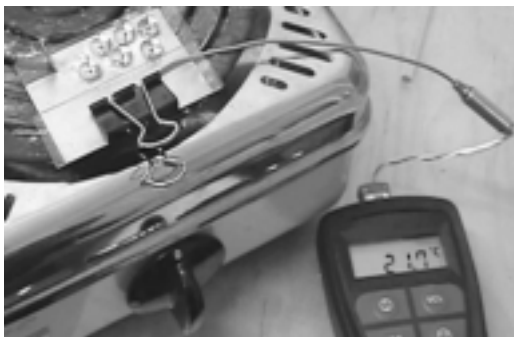
Fig. 5. Assembled experiment before heating. The metal sheet is clamped to the heater between glass slides. The thermocouple is placed below the top slide in contact with the metal sheet. \text{KNO}_3 powder is then distributed onto the metal sheet, and thumbtacks are placed on top of the powder.
