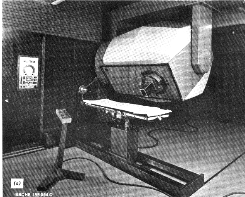
Figure 11.18 Betatron for radiation therapy (45 MeV). (a) Photograph of system: accelerator and treatment table. (b) Cross section of accelerator: gamma ray mode (top) and electron beam mode (bottom). (1) Lead shielding. (2) Transformer yokes. (3) Suspension and rotation mechanisms. (4) X-ray target. (5) Central magnet core. (6) Electron guns. (7) X-ray equalizers. (8) Lead shutter. (9) X-ray monitoring system. (10) Collimator. (11) Movable yoke for servicing. (12) Ten scatterer system for electron beam. (13) Electron radiation monitoring system. (14) Variable localizer. (Courtesy BBC Brown, Boveri and Company.)
