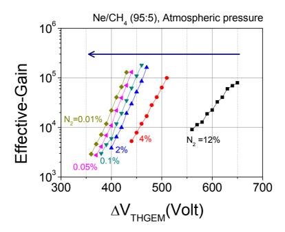
**Figure 16.** Effective-gain in a double-THGEM detector operated with 1 atm. Ne/5%CH<sub>4</sub>, in a vessel containing residual air fraction and being continuously under gas flow; the overall impurity percentage is represented by  $N_2$  percentage in Ne. The time span for the measurement was ~ 20 hours.
