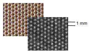
**Figure 22.** Details of the hole-type structure appear in the flat field image when irradiating with low energy X-rays (< 4 keV), where photoelectron ranges are of the order of 0.6 mm.
