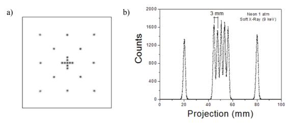
**Figure 21.** Mask image (a) of the THGEM imaging detector of Fig. 3, irradiated with 9 keV X-rays; the 1mm thick mask has 1 mm diameter holes. (b) A projection of the central region of the image.
