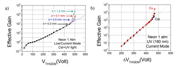
**Figure 12.** a) Single-THGEM gain curves in Ne at atmospheric pressure, measured with electrodes of different holes' diameters. The arrows indicate maximum achievable effective gains. b) Gain-curves measured in Ne with a CsI-coated THGEM and with bare-Cu THGEM at UV flux densities of around  $250 \, \text{s}^{-1} \, \text{mm}^{-2}$ . THGEM geometry:  $t = 0.4 \, \text{mm}$ ,  $d = 0.3-1.2 \, \text{mm}$ ,  $a = 1-2 \, \text{mm}$  and  $b = 0.12 \, \text{mm}$ .
