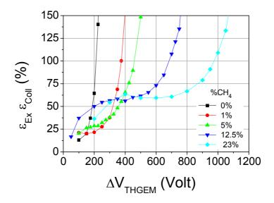
**Figure 19**. Combined photoelectron extraction- and collection-efficiency from a CsI photocathode into THGEM holes  $\epsilon_{Ex} \cdot \epsilon_{Coll} = I_{THGEM}/I_{vac}$ , measured in the setup of Fig. 2b. Data are shown vs  $\Delta V_{THGEM}$  in Ne and Ne-CH<sub>4</sub> mixtures, at atmospheric pressure. The drift field was kept at 0 V/cm. THGEM parameters: t = 0.8 mm, d = 0.5 mm, a = 1 mm and b = 0.1 mm.
