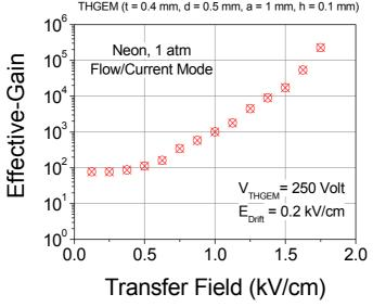
**Figure 7.** Effective-gain variation as function of the transfer field between two THGEMs, with their operation potentials kept at 250 Volt and with  $E_{Drift} = 0.2 \text{ kV/cm}$  (Detector of Fig. 1). THGEM geometry: t = 0.4 mm, d = 0.5 mm, a = 1 mm, b = 0.1 mm.
