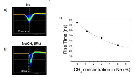
**Figure 9.** Signals from the double-THGEM of Fig. 3 in Ne (a), and in Ne/CH<sub>4</sub> (5%) (b), recorded with ca. 9 keV X-rays. The signal's rise-time as function of  $CH_4$  percentage is shown in c).
