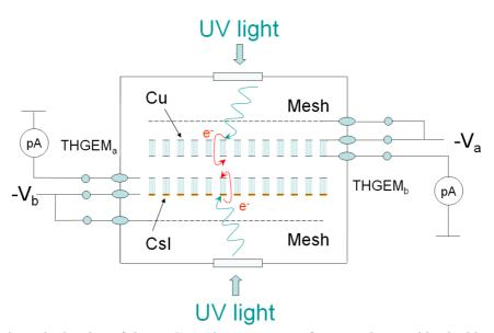
**Figure 2b.** Schematic drawing of the THGEM detectors set-up for extraction combined with collection efficiency measurements.
