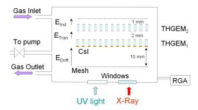
**Figure 1.** Schematic drawing of the THGEM detector investigations set-up (RGA = residual gas analyzer for monitoring the gas composition). The different gap dimensions are given as example and varied according to the experiment.
