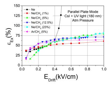
Figure 18. Photoelectron extraction efficiency  $\varepsilon_{Ex}(V_{drift}) = I_{gas}(V_{drift})/I_{vac}$  from the CsI photocathode (Fig. 2a), as function of the drift field; it was measured in parallel-plate mode (no voltage across the THGEM) in Ne, Ne-CH<sub>4</sub> mixtures and in Ar/5%CH<sub>4</sub> at atmospheric pressure. The data were normalized to extraction in vacuum.
