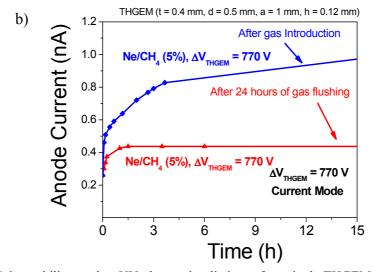
**Figure 10.** Gain stability under UV-photon irradiation of a single-THGEM coated with a CsI photocathode, measured in a): Ne, Ne/5%CH<sub>4</sub> and Ar/5%CH<sub>4</sub> after 24 hours of gas flow prior to measurements; b) Ne/5%CH<sub>4</sub> after 24 hours of gas flow compared to measurements taken immediately after gas introduction. Effective gain:  $\sim 10^4$ ; counting-rate of  $\sim 10^4$  photoelectrons per second and per mm<sup>2</sup>.
