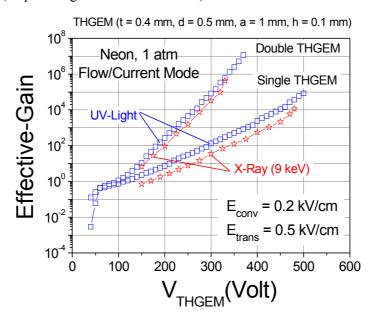
**Figure 6.** Effective-gain curves in Ne of single- and double-THGEM detectors, measured with single UV photons and with soft X-rays. THGEM geometry: t = 0.4 mm, d = 0.5 mm, a = 1 mm and b = 0.1 mm.
