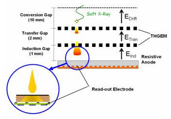
Figure 3. The THGEM-based imaging detector set-up.
