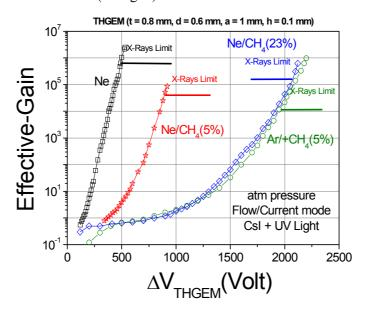
**Figure 4.** Effective-gain curves obtained in the single-THGEM detector of Fig. 1, with single UV photons (CsI photocathode;  $E_{drift} = 0$ ) in Ne, Ne/CH<sub>4</sub> mixtures and in Ar/CH<sub>4</sub> (95:5). The maximum effective gain reached in each gas, in the same detector, with 9 keV (Cu-K<sub> $\alpha$ </sub>) X-rays is also shown ( $E_{drift} = 0.2 \text{ kV/cm}$ ). THGEM geometry: t = 0.8 mm, d = 0.6 mm, a = 1 mm, b = 0.1 mm.
