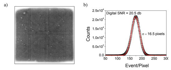
**Figure 20.** a) Grey-level flat-field image of the double-THGEM imaging detector of Fig. 3. b) Histogram of the flat-field image depicted in fig. a); the Gaussian fit of the histogram is shown (red line).
