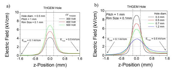
**Figure 13.** a) depicts the electric field calculated on the hole's axis for various voltage differences applied across the THGEM while b) depicts the electric field strength along the hole's axis for different hole's diameters.
