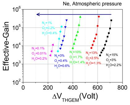
**Figure 15.** Gain curves in a double-THGEM detector, measured in a vessel containing residual air fraction, and being continuously under Ne gas flow; the impurity percentage is indicated for  $N_2$ ,  $O_2$  and  $H_2O$ . The time span for the measurement was  $\sim 20$  hours.
