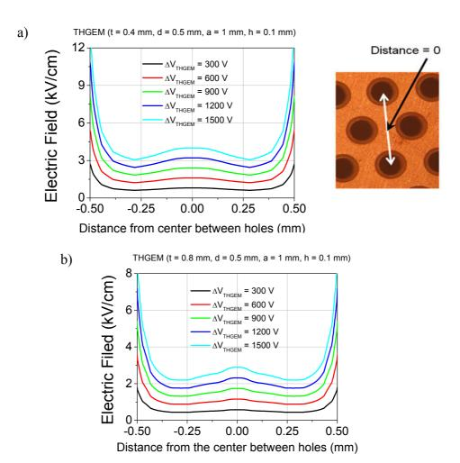
**Figure 17.** Calculated electric field strength on the top-surface of the THGEM along a line between two neighboring holes (scheme on the right); the fields are calculated for different  $\Delta V_{THGEM}$  values. Drift and induction fields were 0 kV/cm. a) THGEM parameters: t=0.4 mm, d=0.5 mm, a=1 mm and h=0.1 mm; b) THGEM parameters: t=0.8 mm, d=0.5 mm, a=1 mm, b=0.1 mm.
