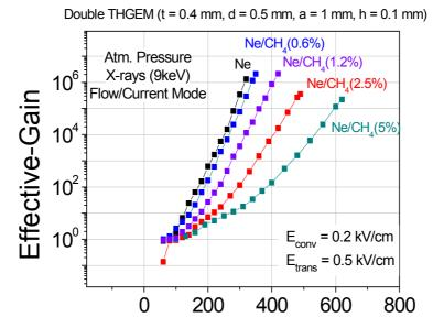
**Figure 5.** Effective-gain curves in the double-THGEM imaging detector of Fig. 3; data measured in Ne and Ne-CH<sub>4</sub> mixtures, in gas flow-mode, with 9 keV X-rays. THGEM geometry: t = 0.4 mm, d = 0.5 mm, a = 1 mm, h = 0.1 mm.
