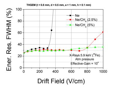
**Figure 8.** Energy resolution of 5.9 keV X-rays, measured in a single-THGEM at an effective gain of  $\sim 10^4$ , as function of the drift field, in Ne and Ne/CH<sub>4</sub> mixtures. THGEM geometry: t = 0.8 mm, d = 0.5 mm, a = 1 mm, b = 0.2 mm.
