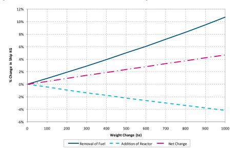
Figure 2:Ship KG Vs Weight Change
