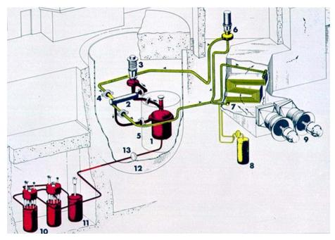
Figure 1: The Molten Salt Reactor Experiment
