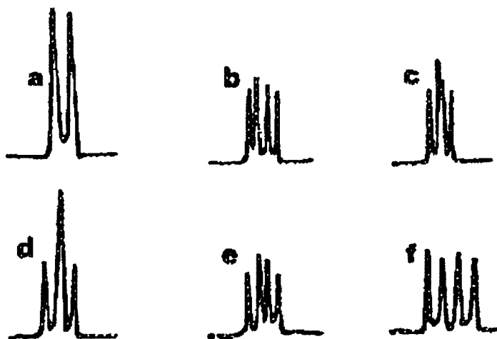
Fig. 10.27. Changes in the propylenediamine methyl resonance of a racemic mixture of 4 ( M = \text{Ni} , R = \text{CH}_3 , R' = \text{CH}_3 , X = \text{H} ) on addition of \text{Eu}(++)\text{fpc}_3 : (a) original methyl doublet; (b-f) changes on addition of LSR.
