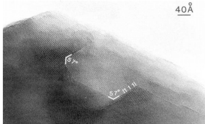
Figure 3-30. A leach pit developed at the dislocation site. The fast reaction generates {111}-surface steps as pit walls.
