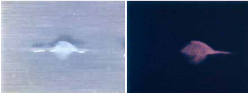
Figure 9-39. Infusion mass viewed in visible light (left). Infusion mass viewed during UV excitation at 254 nm (right). (Reprinted with permission from ref 78. Copyright 2002 IOP Publishing Ltd.)
