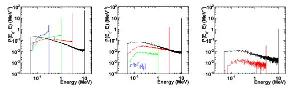
Figure 9. Photon spectra at the observatory derived from Monte Carlo simulations. Three panels correspond to d = 300 m (left), 1000 m (middle), and 2000 m (right). Different colors denote incident photon energies,  $E_0 = 0.3$  (blue), 1 (green), 3 (red), and 10 MeV (black) in all panels. Abscissa shows the photon energy at the observatory, while ordinate represents probability density function.
