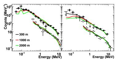
**Figure 10.** The photon spectra observed by the NaI (filled circles) and CsI (open circles) scintillators of Detector-B, compared with calculations for assumed source distances of 300 m (black), 1000 m (red), and 2000 m (green). Left panel shows 071213, while right one indicates 081225. For clarity, the CsI data and the corresponding model spectra are multiplied by 0.1. The horizontal and vertical axes show the photon energy in MeV and counts in each bin, respectively.
