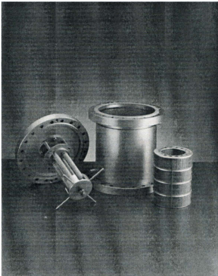
A nonevaporable getter pump (NEG). The getter cartridge, consisting of four rows of accordion-pleated getter strips is on the right. The cartridge support and heater is on the left. Reprinted with permission from SAES Getters/USA., Inc.
