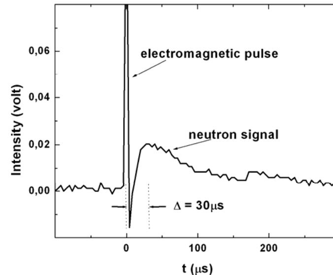
In addition as the neutron signal is preceded by the electromagnetic pulse of the plasma focus discharge, the neutron signal is coincident with the discharge and it is possible secure that the signal is from the plasma focus event. In discharges in hydrogen in which neutrons are not emitted only the electrical noise is register in the signal, background radiation is not detected in that small temporal windows of hundreds of microseconds.
