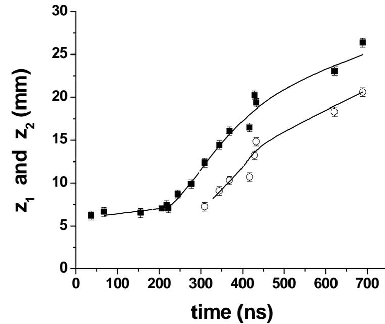
**Fig. 5. Radial plasma motion  $a(t)$  and motion of the frontal and rear axial plasma edge,  $z_1(t)$  and  $z_2(t)$**
