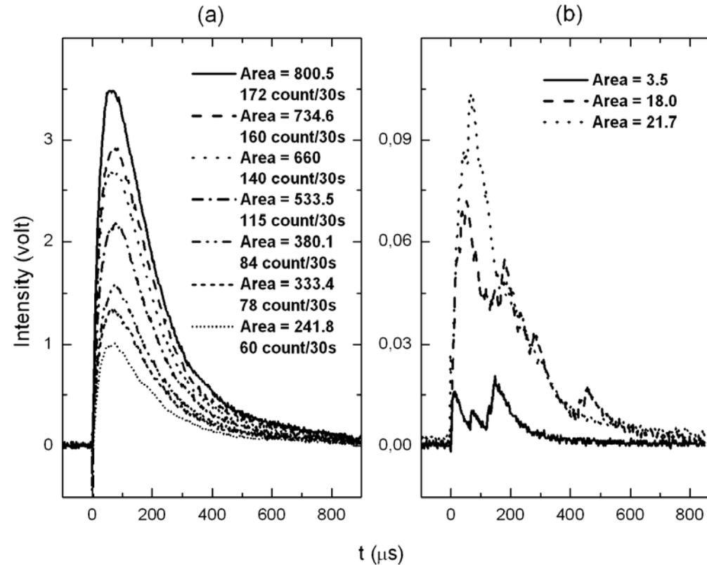
Count rate vs. area under the curve of the signal and the count rate vs. the maximum intensity of the signal, show that a linear relation exists in both cases.
