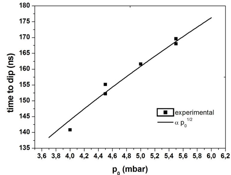
Time to dip vs filling pressure for discharges in hydrogen. The time to dip dependence on pressure,  $\propto \sqrt{p_0}$ , shows that the device is working as plasma focus.
