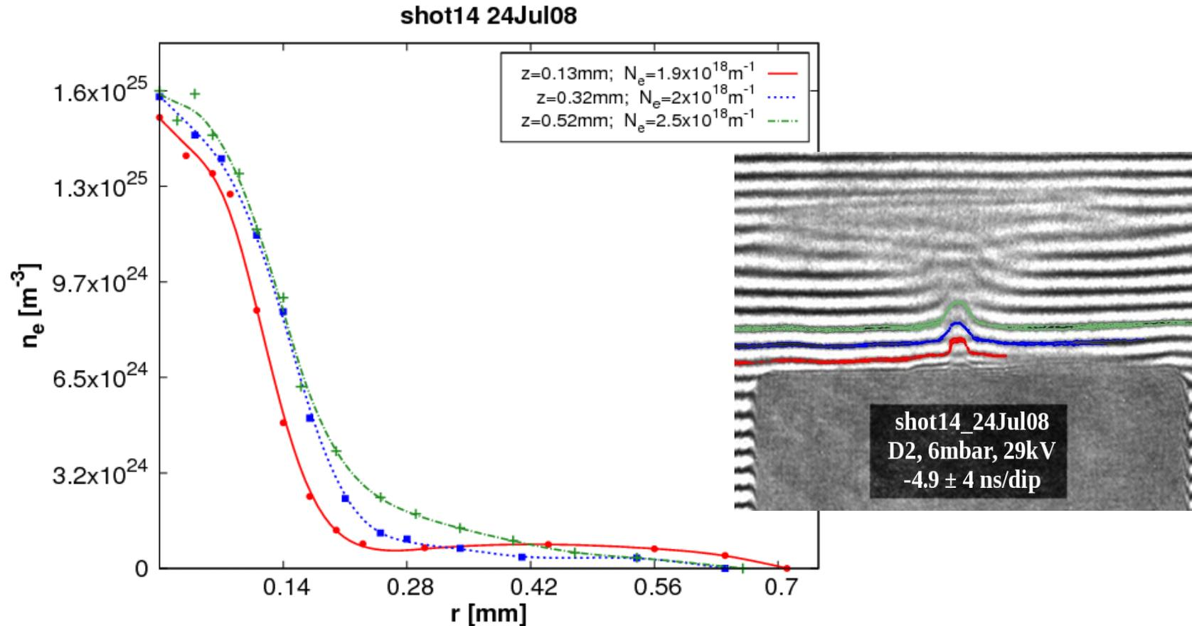
**For Deuterium, it has been found that densities as high as  $10^{25} \text{ m}^{-3}$  are reached in the axis, while the line density is of the order of  $10^{18} \text{ m}^{-1}$ .**
