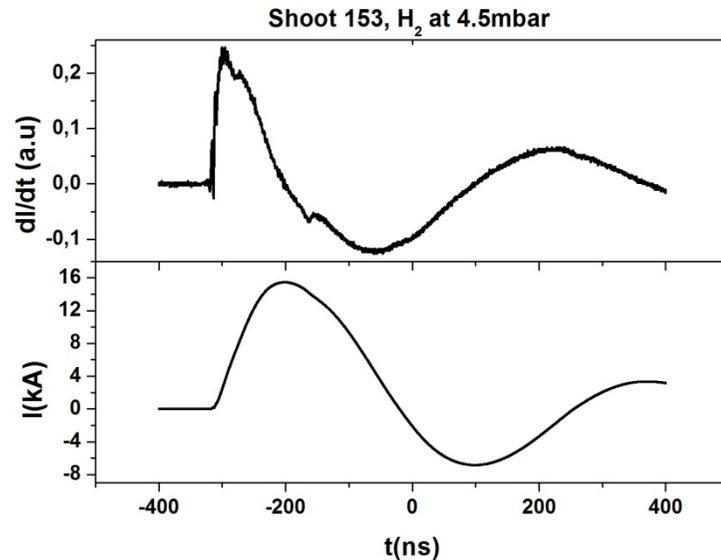
Electrical signals of the current derivative  $dI/dt$  and current  $I$ . The typical dip in the  $dI/dt$  and the drop in  $I$ , that correspond to the pinch effect is observed.
