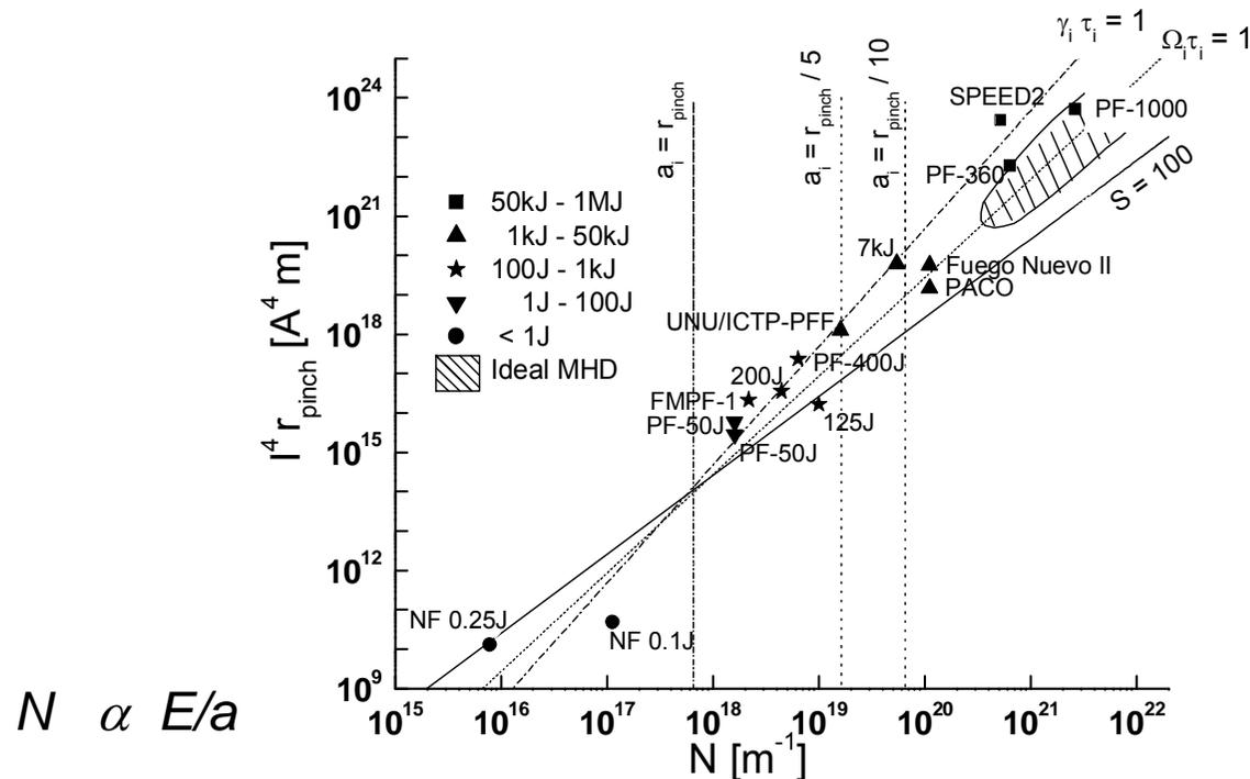
Different plasma foci that work with stored energy ranging from 0.1 J to 1MJ are plotted in the diagram for Z-pinch stability given by Haines and Coppins
