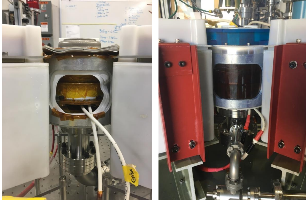
Figure 4. (left) Last year's Mylar-based high-voltage insulator. (right) Improved 3d-printed acrylic insulators. The red beams are fiberglass struts to secure the pulsed power system to the test stand frame.
