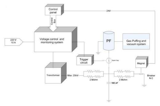
Fig. 2: Schematic of the electrical and mechanical systems of SORENA-1.
