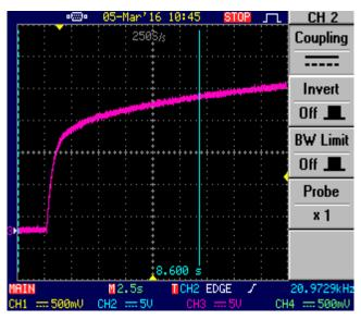
Fig. 13: Charging of capacitor by DC power supply
