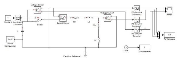
Fig. 6: Equivalent Circuit diagram of plasma and spark gap in MATLAB/Simulink
