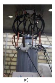
Fig. 4: a) General view of SORENA-1 b) power supply box c) transformer d) charge and discharge resistances and damper e) capacitor and its connections to spark gap
