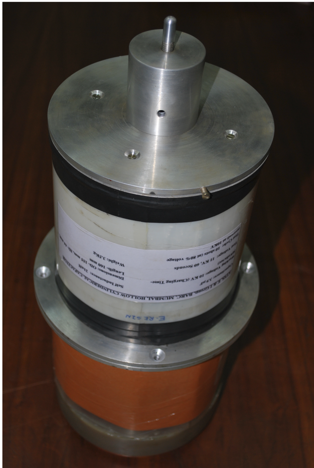
FIG. 6. Compact pulsed power system (20 kV, 400 J).
