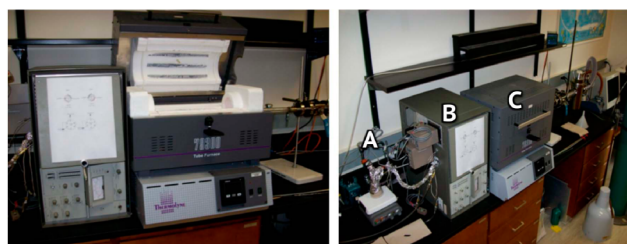
Figure 2. Photos of the horizontal hot-walled ALD system, composed of the (A) coreactant ( \text{H}_2\text{O}/^i\text{PrOH} ) injection system, (B) precursor oven–injection system, and (C) deposition chamber. The sand bath used to heat the coreactant flask (A) is not shown in the image.
