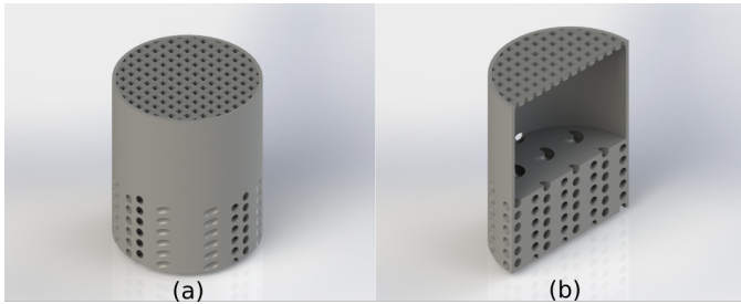
Figure 3: Micro-helix cavity design printed as an acoustic cylinder: (a) Overall view, (b) Cross section
