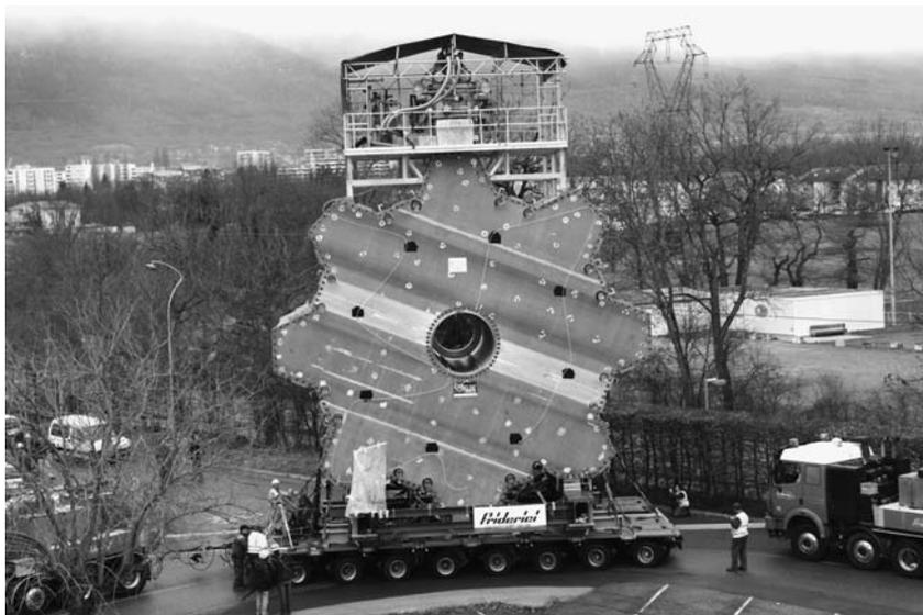
**Figure 7.11** Transport of the ATLAS end-cap toroid magnet, weighing 240 tonnes, on a special trailer with 128 wheels, on 6 February 2007.
