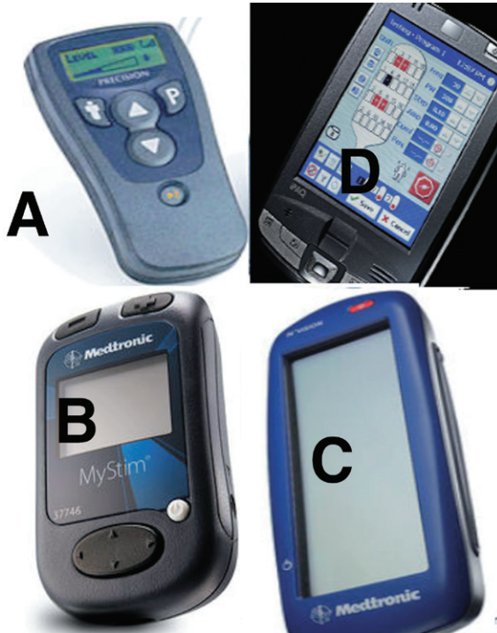
Figure 18.4 Some of the non-implantable components of spinal cord stimulation. A and B, Examples of patient controllers; C and D, examples of physician programmers.
