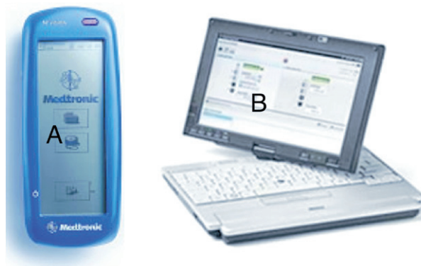
Figure 2.4 Photograph of the two most commonly used physician programmers in deep brain stimulation. (A) N'Vision from Medtronic; (B) Athena from St. Jude Medical.
