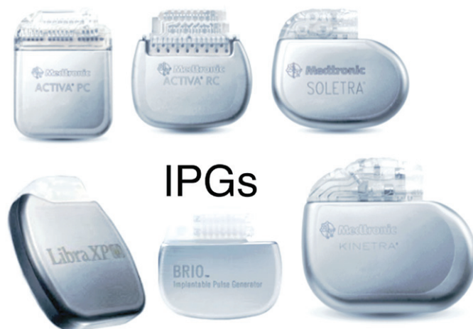
Figure 2.1 Photograph of different implantable pulse generators for deep brain stimulation: Activa PC, RC, Soletra and Kinetra from Medtronic [1] (Soletra and Kinetra discontinued), LibraXP and Brio from St. Jude Medical [2]. Activa RC and Brio are rechargeable. Other vendors are coming on the market, e.g., Boston Scientific [3]. Please check licenses for specific indications before using devices in patients.
