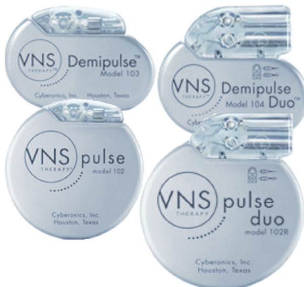
Figure 13.1 Photograph of four models of NCPs: Demipulse™ Model 103 (top left) with single pin, Demipulse™ Model 104 Duo™ (top right) with dual pins, pulse model 102 and pulse duo model 102R (bottom left and right) older models.
