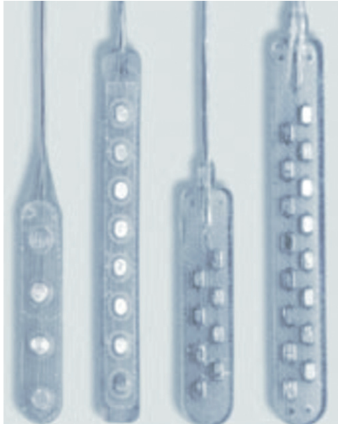
Figure 16.1 Paddle leads used in spinal cord stimulation and were used off label in motor cortex stimulation.
