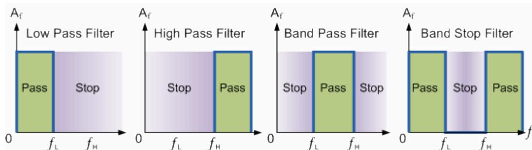
Filters can be divided into two distinct types: active filters and passive filters. Active filters contain amplifying devices to increase signal strength while passive do not contain amplifying devices to strengthen the signal. As there are two passive components within a passive filter design the output signal has a smaller amplitude than its corresponding input signal, therefore passive RC filters attenuate the signal and have a gain of less than one, (unity).
