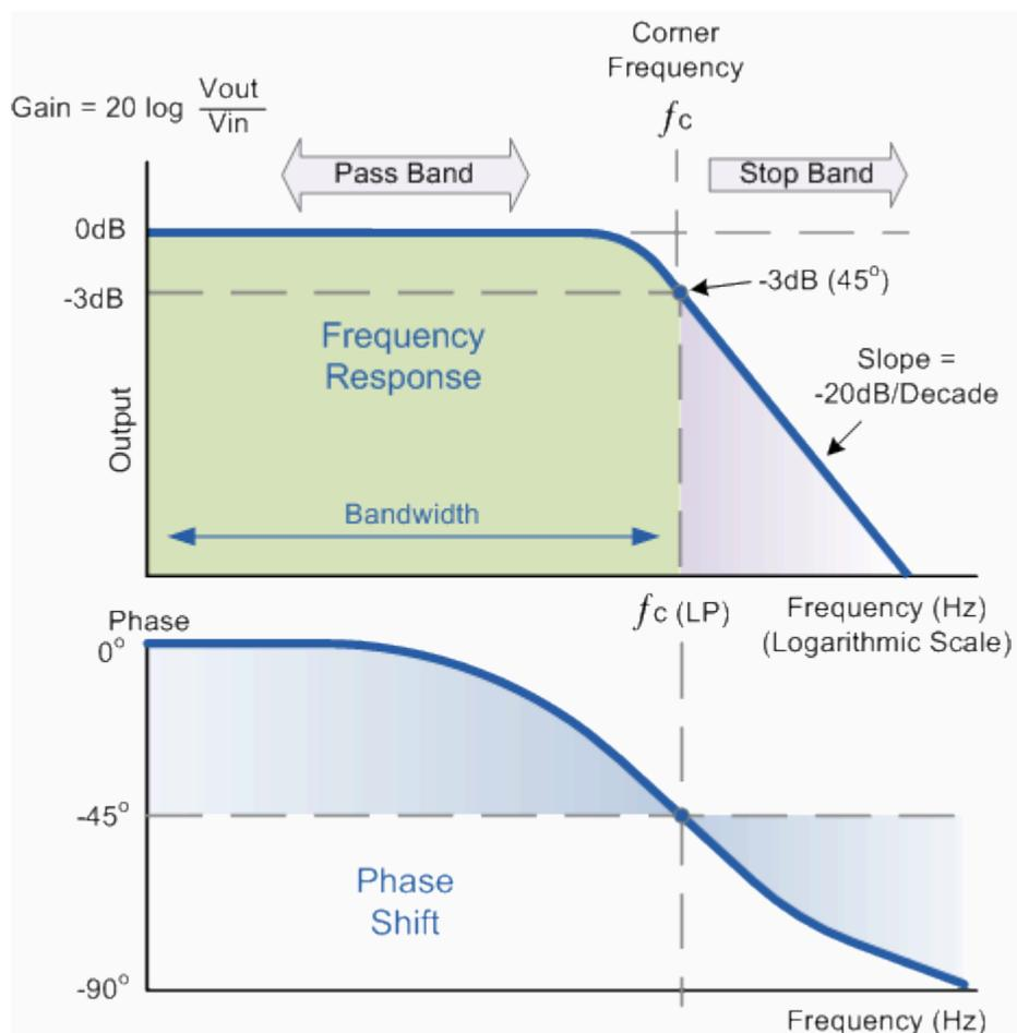
The Bode Plot shows the **Frequency Response** of the filter to be nearly flat for low frequencies and all of the input signal is passed directly to the output, resulting in a gain of nearly 1, called unity, until it reaches its **Cut-off Frequency** point ( $f_c$ ). This is because the reactance of the capacitor is high at low
