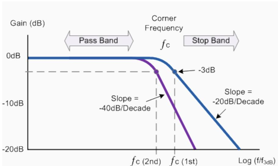
In practice, cascading passive filters together to produce larger-order filters is difficult to implement accurately as the dynamic impedance of each filter order affects its neighbouring network. However, to
