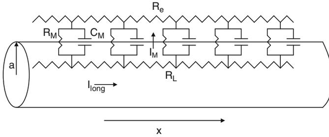
**Fig. 1.5** Equivalent circuit for a uniform passive cable.  $I_{\text{long}}$  is the current along the inside of the cable,  $I_M$  is the current across the membrane,  $R_L$  is the resistance of the cytoplasm,  $R_e$  is the resistance of the extracellular space,  $R_M$  is the membrane resistance, and  $C_M$  is the membrane capacitance
