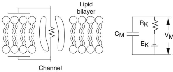
**Fig. 1.2** The cell membrane showing the insulating lipid bilayer and a K<sup>+</sup> channel, which allows current to flow. The equivalent electrical circuit is shown on the *right*
