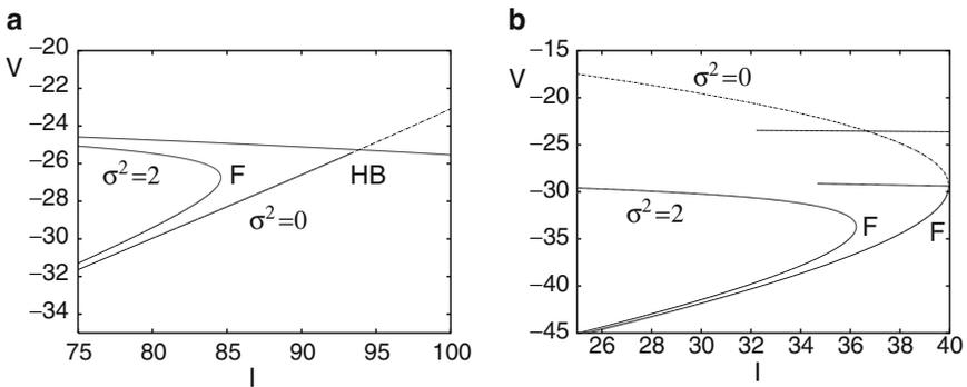
**Fig. 10.6** Bifurcation diagram for Morris–Lecar moment expansion for (a) class II and (b) class I excitability as the current varies at zero noise and with large noise ( $\sigma^2 = 2$ ). In each case, the addition of noise shifts the loss of the stable fixed point to a lower value of  $I$
