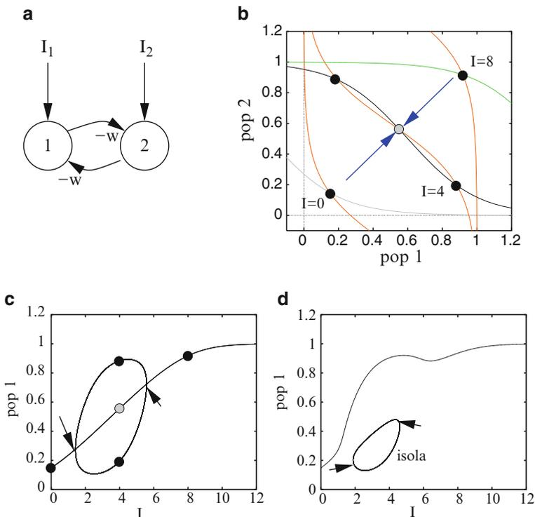
**Fig. 11.3** The simplest model for competition between two populations: (a) the circuit, (b) null-clines for identical inputs at three different strengths, (c) bifurcation diagram when the inputs are identical, and (d) same as (c) but there is a small bias in favor of population 1
