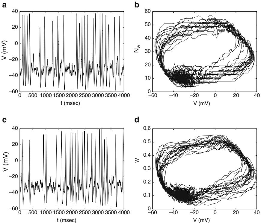
**Fig. 10.7** Stochastic simulation of the Morris–Lecar model with 100 potassium and 100 calcium channels.  $I = 80 \mu\text{A}/\text{cm}^2$  injected is subthreshold for repetitive firing. (a) Time series of the voltage. (b) Projection onto the  $(V, W)$  plane showing the stochastic limit cycle. (c, d) Langevin approximations to the channel dynamics
