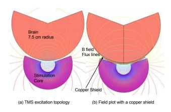
Fig. 4 Transcrannial magnetic stimulation B field plot without (a) and with (b) a passive copper shield.
