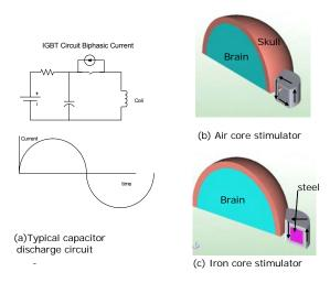
Fig. 1 (a) Typical magnetic stimulation circuit, (b) ½ of an air core stimulator for TMS, and (c) an iron core stimulator showing a winding wrapped around a tape wound laminated core..
