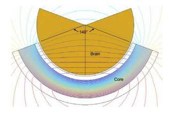
Fig. 12 Core opened to 140°, 3790 AT excitation at 5280 Hz.
