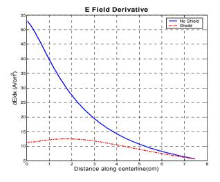
Fig. 7 E field gradient along a radial line centered at the core.
