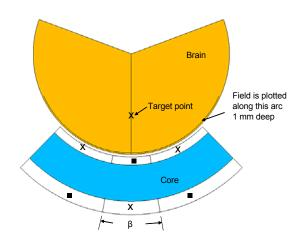
Fig. 10 Opening the angle of the core yields deeper field penetration.
