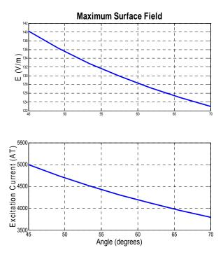
Fig. 13 Peak surface field and amp-turn excitation with increasing core angle.
