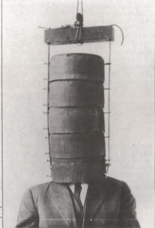
**Figure 4.** The magnetic coils of Magnusson and Stevens reported in 1911 and 1914.<sup>17,18</sup> Additional sections of coils could be energized to increase the magnetic field.
