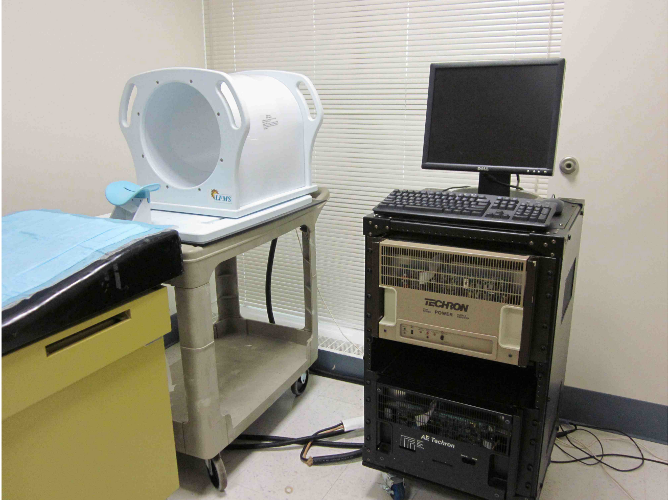
Figure S1. LFMS Device. The LFMS includes a coil, power source and computer with control card. The treatment volume is at the end of the coil, so the patient's head is not inserted far into the device. Fields inside the device were calculated and measured to be on the order of 0.7 V/m and 20 Gauss. These fields replicate the features first observed to produce an antidepressant effect in a magnetic resonance imaging (MRI) setting, using a magnetic resonance spectroscopic imaging procedure, as previously reported (1).
