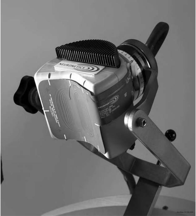
**Figure 5-2.** E-shield system used to make active transcranial magnetic stimulation (TMS) feel like sham TMS.
