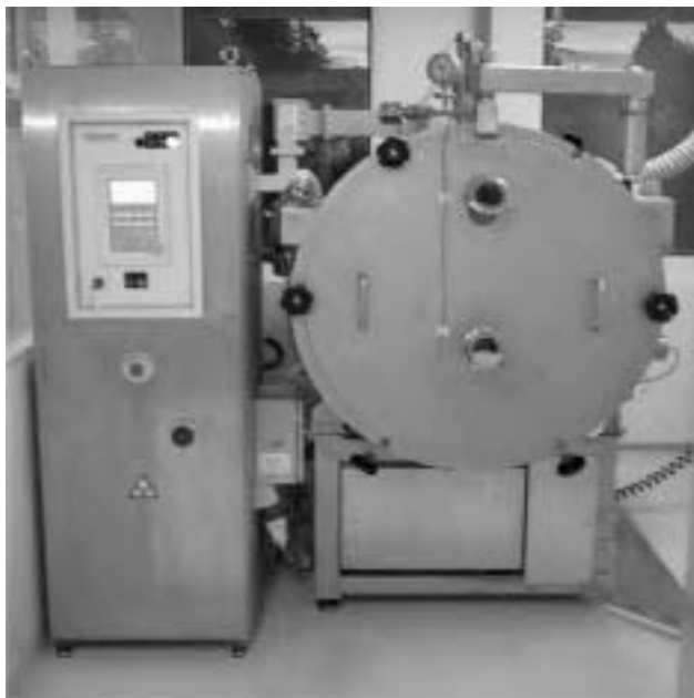
Fig. 14.28 Microwave disk dryer for combined air circulation and vacuum mode under explosion protection.
