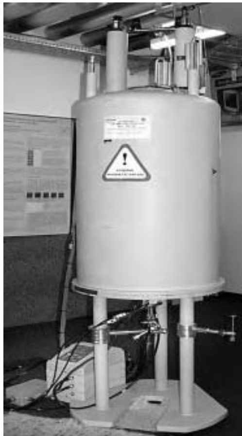
Fig. 13.15 Tomograph used for temperature mapping experiments.
