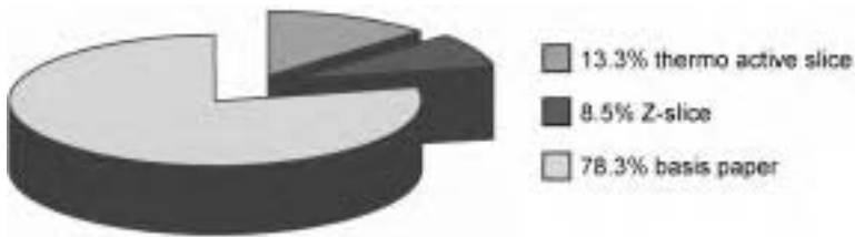
Fig. 13.10 Composition of thermo paper (percentage referred to the thickness of the thermo paper) (Umweltberatung Bayern, 1997).
