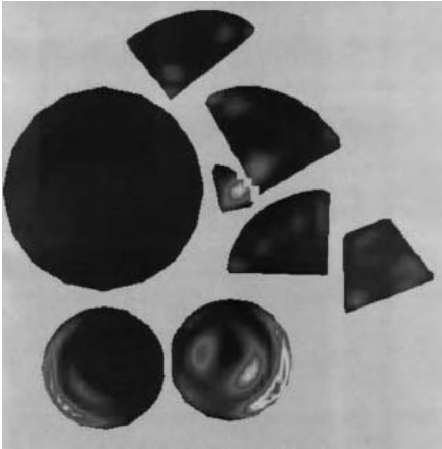
Fig. 15.7 Predicted dissipated power in a multi-component ready meal. The meal is heated from frozen, and consists of mashed potato (the larger component), two meat patties (at the bottom), and pieces of parsnip (upper left), and Swedish turnip (middle right). The heating uniformity would be more levelled out if the product were designed in a way which would allow a quicker thawing of several of the components and a more levelled out heating distribution between the components.
