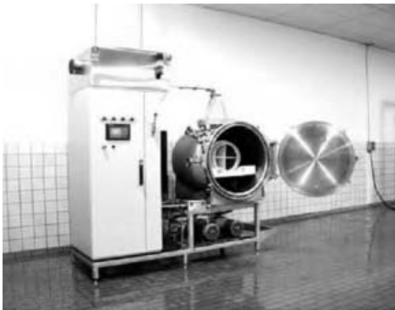
Fig. 6.3 EnWave VM Model 15, 15 kW, 2450 MHz, fully variable microwave power with vacuum to 30 torr (Enwave Corporation, BC, Canada).
