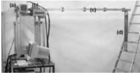
Fig. 13.17 (a) Absorbing units; (b) microwave generator; (c) rectangular waveguide; (d) circular waveguide (for introducing microwaves in tomography).
