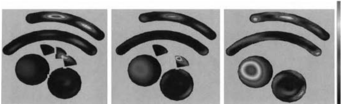
Fig. 15.8 Predicted microwave heating pattern in a multi-component ready meal, consisting of two sausages, two components of mashed potato and pieces of blanched vegetables. From left to right: three different planes through the ready meal, lower, middle and upper planes, located 5 mm from each other. The lower plane is located 5 mm above the bottom of the meal. The overheated areas and the non-uniformity between different components indicate the need for optimisation of the product, similar to the solutions for the previous cases (see Fig. 15.7 and compare with Figs 15.5 and 15.6).
