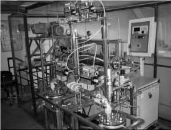
Fig. 14.32 2 \times 2 \text{ kW}/2450 \text{ MHz} pilot plant at the TU-Berlin, Institute of Biotechnology.
