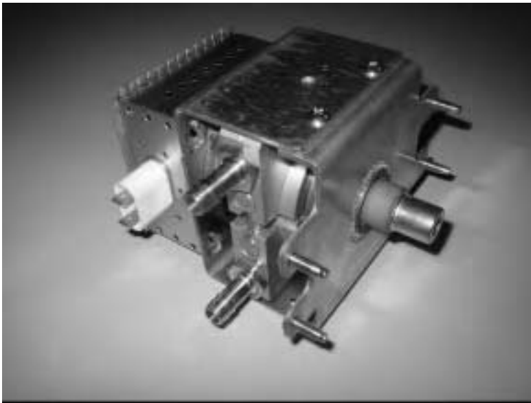
Fig. 14.3 1.2 kW/2450 MHz magnetron 2M137 type with a water-cooling jacket. 1
