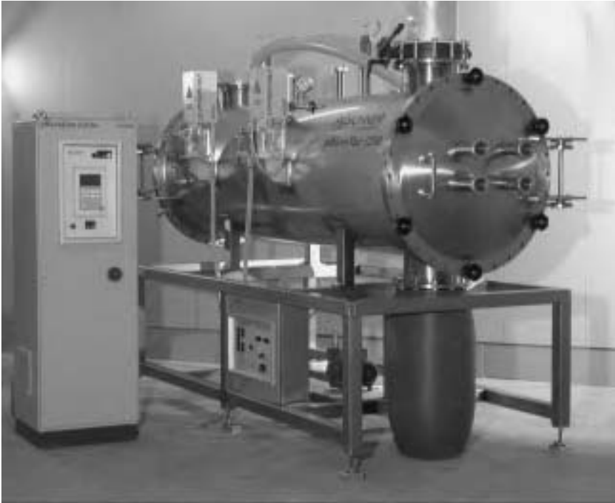
Fig. 14.27 12 kW/2450 MHz double stage continuous belt dryer.
