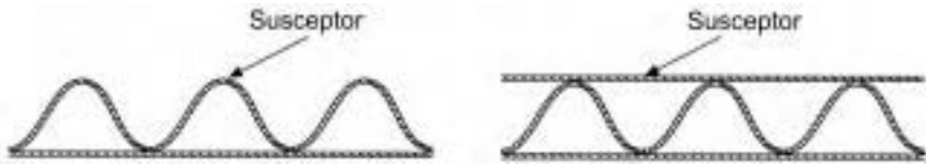
Fig. 11.6 Two types of fluted or corrugated susceptor. On the left, the fluted surface is coated with the metalized susceptor and provides channels for evolved moisture to escape. On the right, the metalized susceptor is on the flat top surface – the fluted corrugations insulate the susceptor from the floor.
