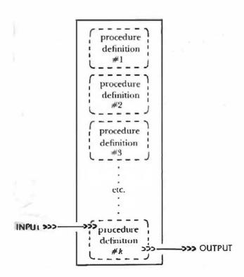
FIGURE 72. The structure of a call-less BlooP program. For this program to be self-contained, each procedure definition may only call procedures defined above it.
