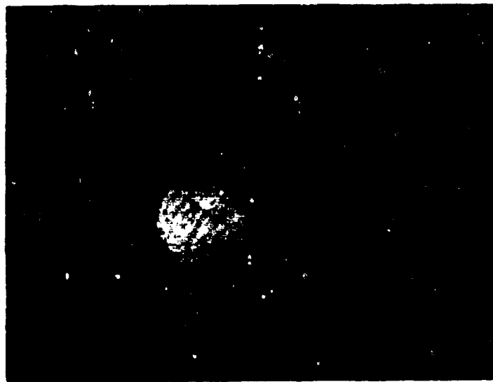
Figure A7: Imprint of TEA laser beam at focus of a mirror of focal length 1.5 m. The 1.5 cm diameter of the imprint implies 10 mradian beam divergence.
