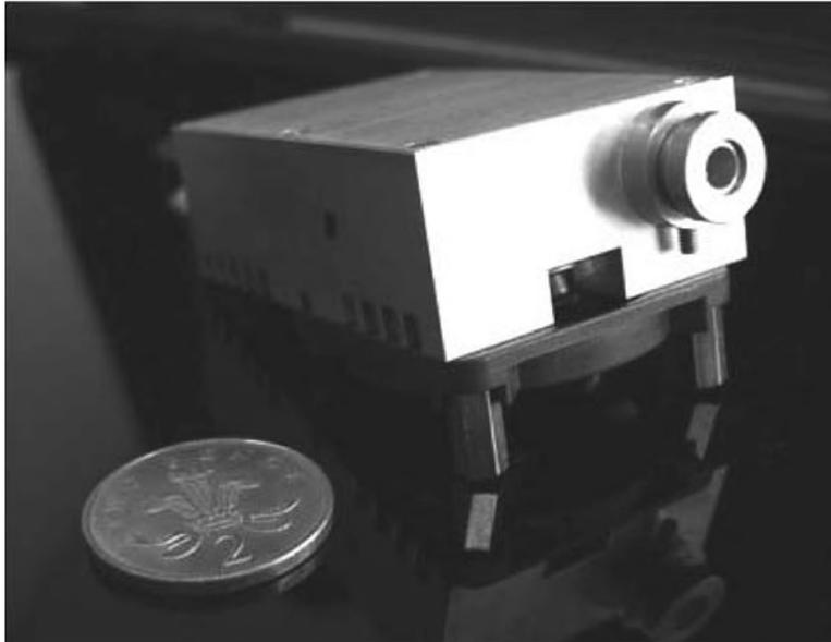
Since such a projector generates a diffracted image in the far field, there is no need for an objective lens and/or a zoom lens, and thus the size of the projector can remain very small. However, due to small diffraction angles generated by dynamical diffractives, an additional optical setup is usually necessary to increase these angles.
