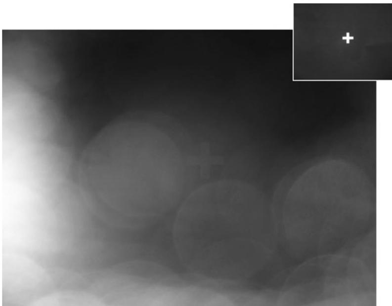
priority. In such systems small dust particles may be a significant portion of the diameter of the pupil. The depth of field is large in a slow system, so several optical surfaces may contribute particle obscurations to any given field point. This may cause obscurations to occur in the image. The dust particles in slow systems are often likened to being “rocks in the image.”
