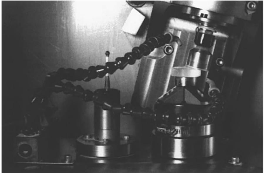
CNC polishing machine (Fig. 18.6). Determining which polishing method is most appropriate depends on geometry of the lens as well as the quantity being produced. For example, if the lens has a relatively long radius of curvature, then conventional polishing of a multiple block may be most cost effective.
