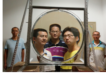
Figure 2: Virtual image formation using the water lens as a magnifying glass.
