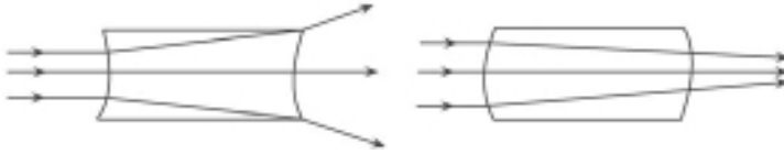
Fig. 4.4-6 The phenomenon of thermal distortion
