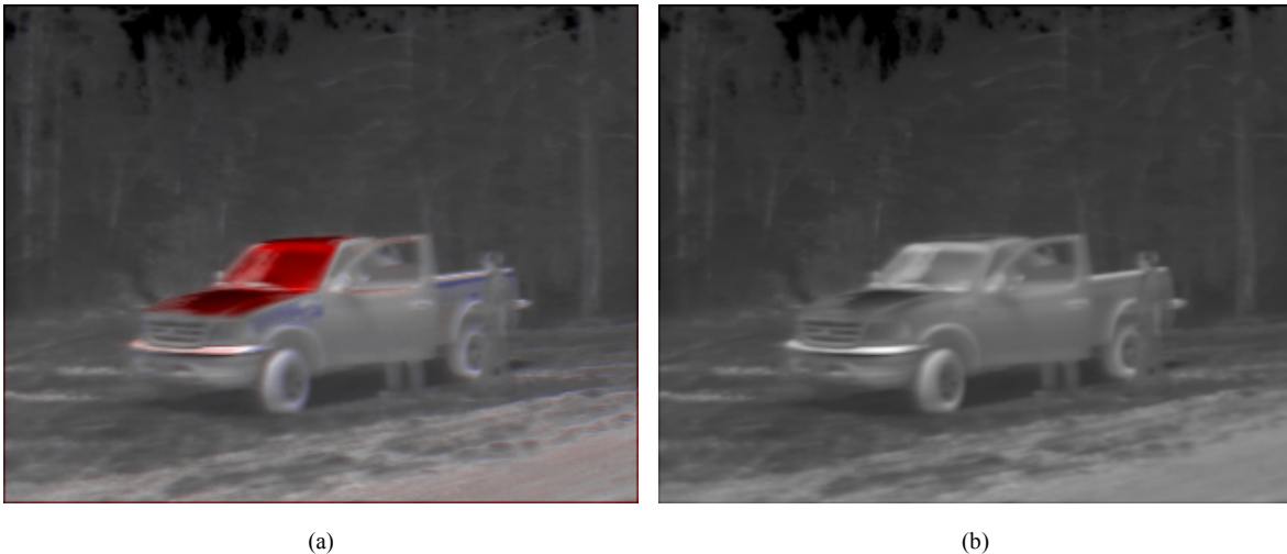
Fig. 11. (a) Color-fusion of an S_1 Stokes parameter image taken from a moving vehicle that was driving past a pickup truck. (b) Intensity image ( S_0 ). Full color saturation occurs at a value of 0.06. Red and blue denote vertical and horizontal polarizations, respectively.
