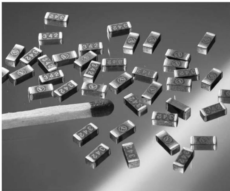
Fig. 16.18. Marking of surface mounted devices (SMDs) [7]
