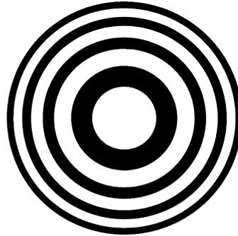
Fig. 4.27 Two dimensional Fresnel zone plate
