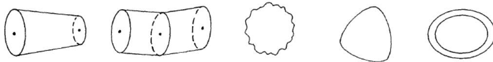
Fig. 8 Examples of non-cylindricity
