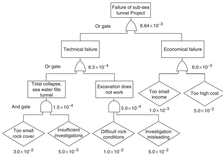
Fig. 26.5 Example of a fault tree with “and gates” and “or gates” and evaluated probabilities for an under-sea tunnel (Eskesen et al., 2004).
