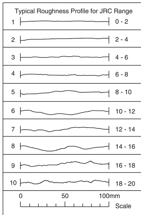
Fig. 7.1 Standard profiles for visual estimation of JRC (Barton & Choubey, 1977).
