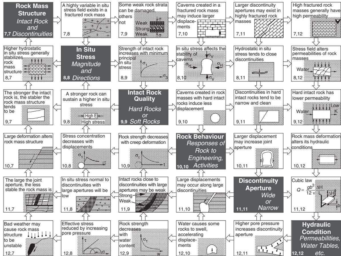
Fig. 13.2b Interaction of rock parameters in the underground excavations (Hudson, 1991).
