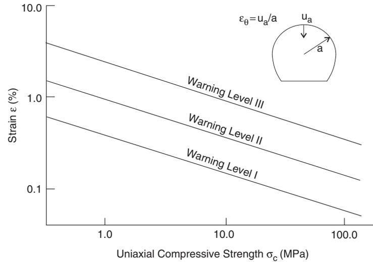
Fig. 8.2 Hazard warning levels for assessing the stability of tunnels (Sakurai, 1997).
