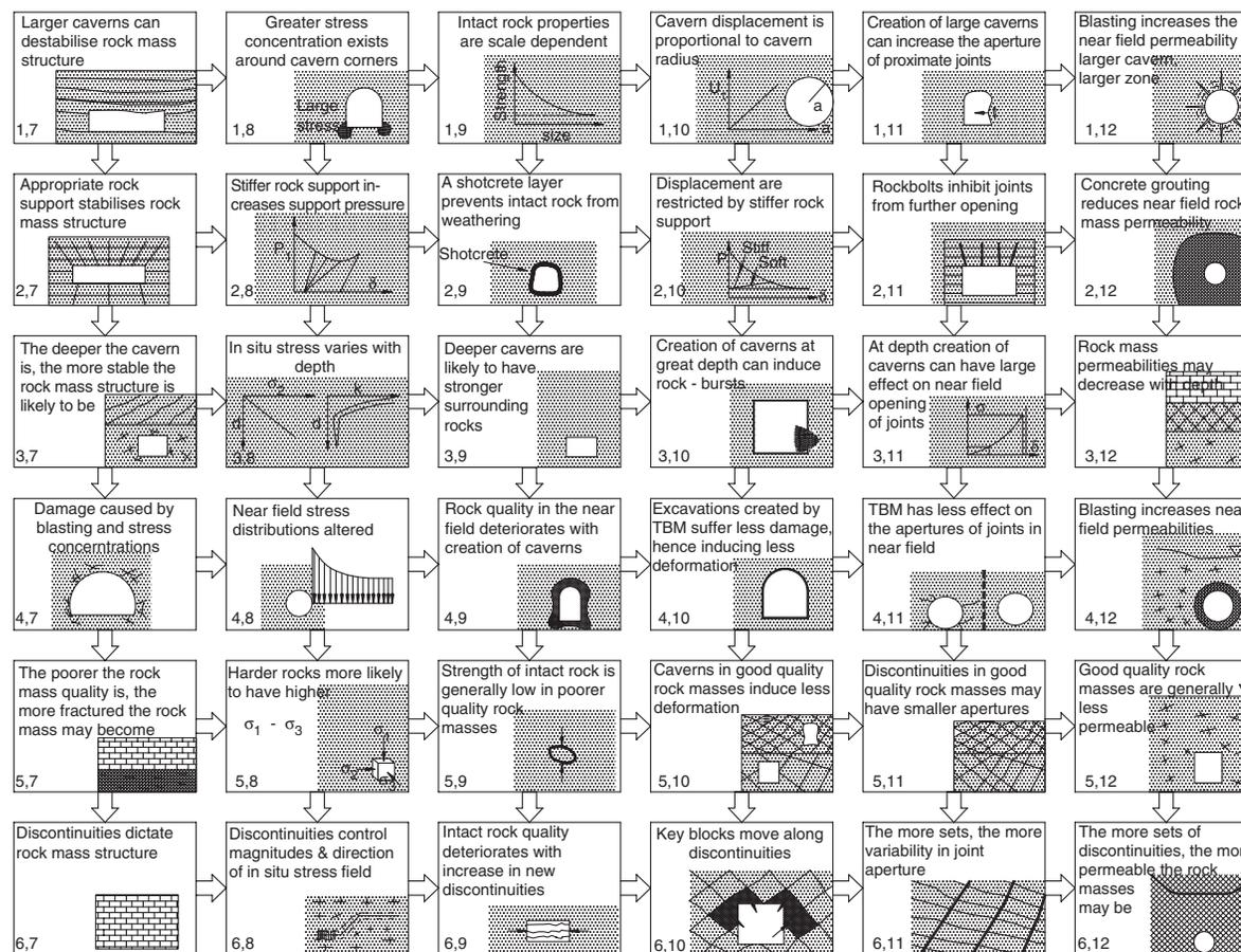
Fig. 13.2c Interaction of rock parameters in the underground excavations (Hudson, 1991).
