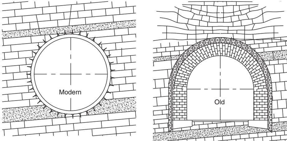
Fig. 9.3 Loosening must be prevented as it reduces strength.
