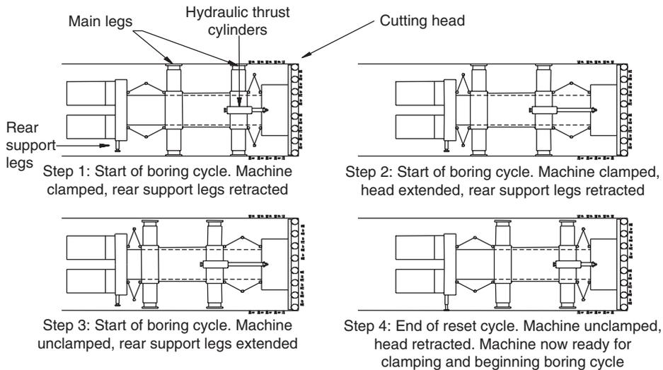
Fig. 15.5 Method of advance of a rock tunnelling machine (Bickel & Kuesel, 1982).
