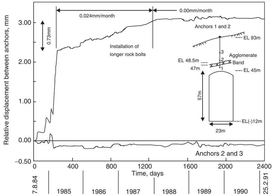
Fig. 14.10 Monitoring agglomerate band behavior with the multi-point borehole extensometer in the roof of a large underground cavity, India (Goel, 2001).
