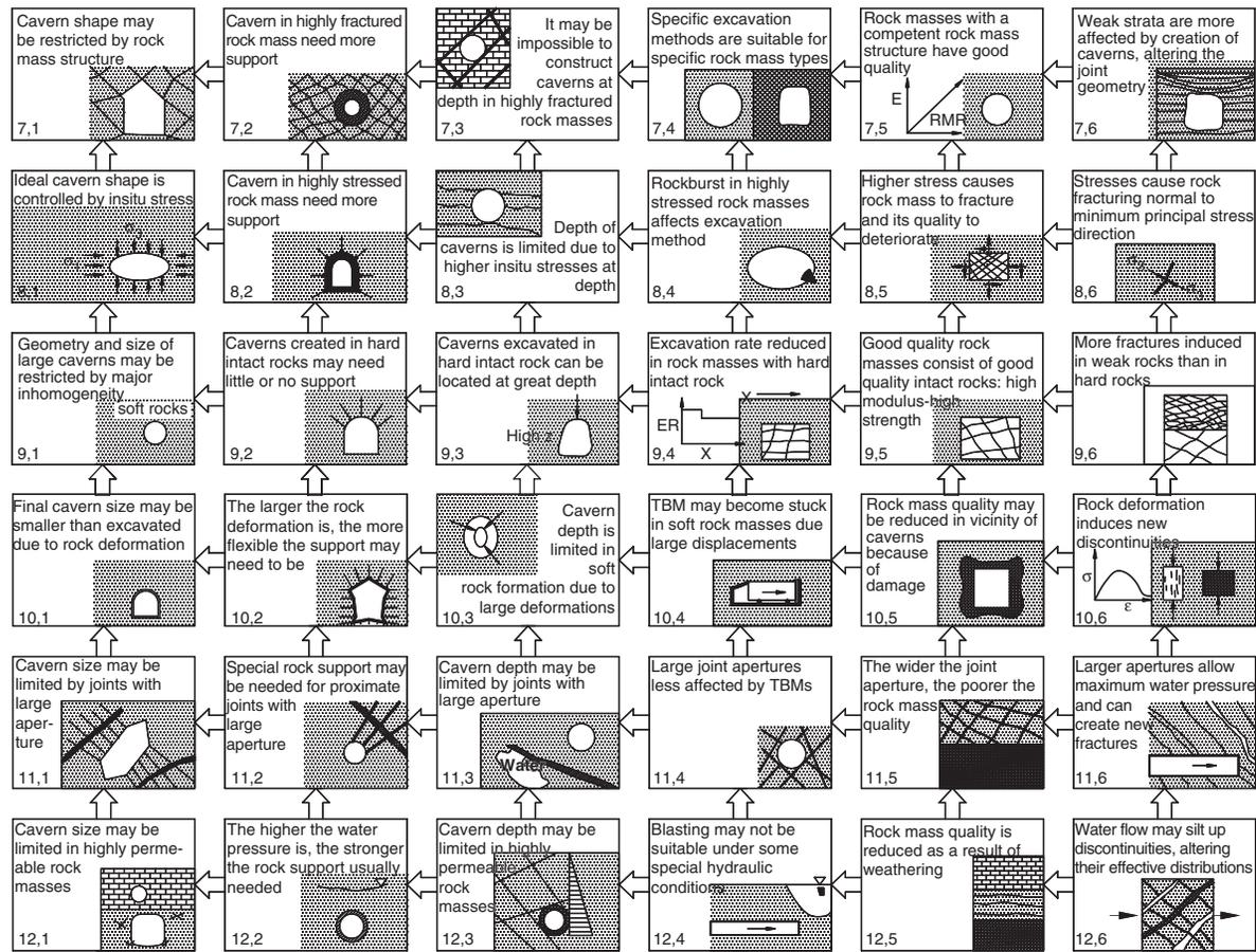
Fig. 13.2d Interaction of rock parameters in the underground excavations (Hudson, 1991).
