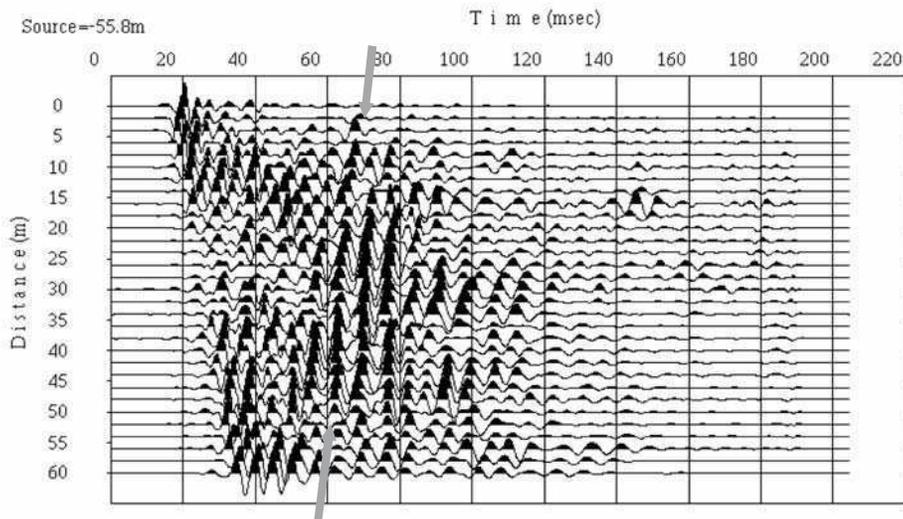
Fig. 2.12 A shot gather after applying a band-pass and F-K filter. Big arrows indicate reflected waves from a reflector ahead of the tunnel face.
