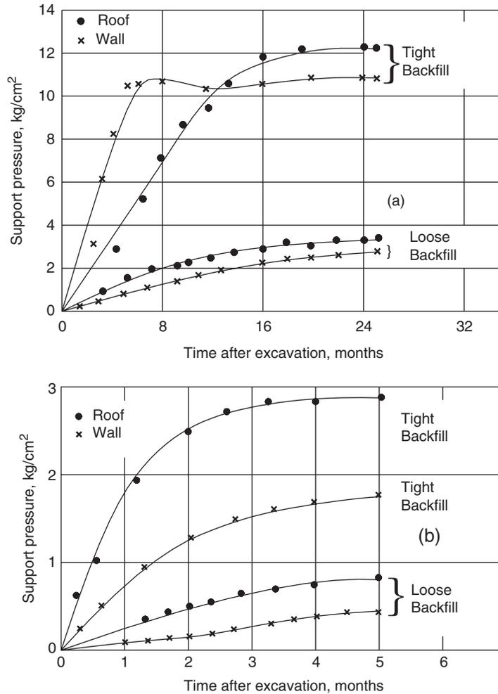
Fig. 20.15 Effect of type of backfill on support pressure in (a) black clays; (b) red shales.
