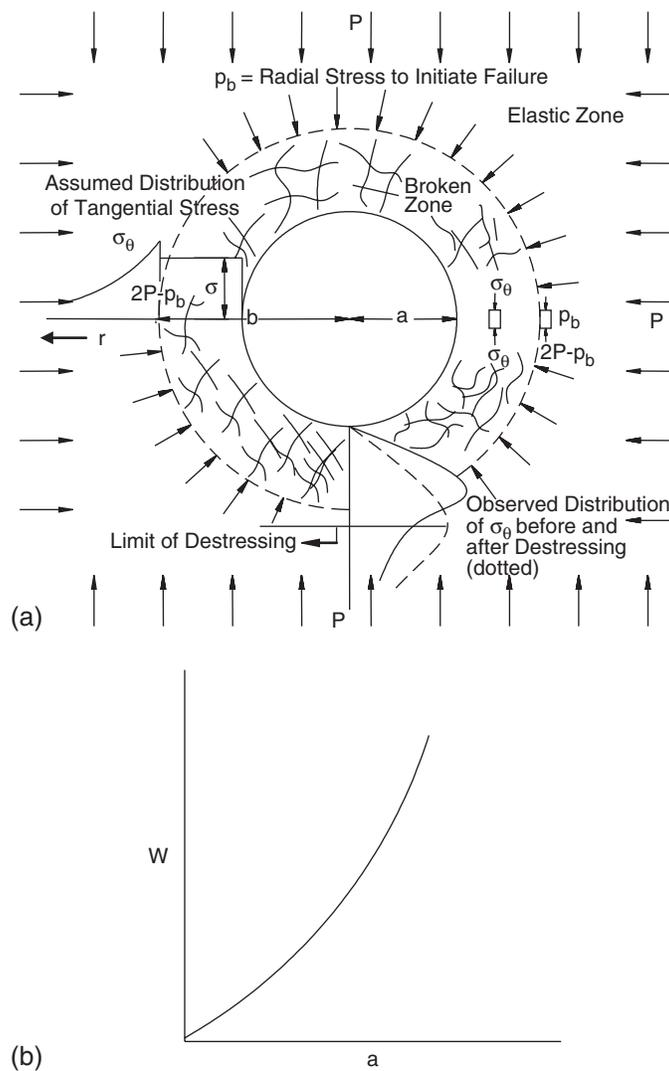
Fig. 22.2 Energy released in a rock burst;  $W$  is the difference in energy released by elastic zone and that absorbed by broken zone.
