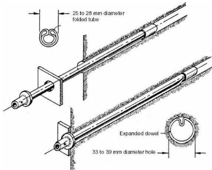
Fig. 12.6 Swellex tube bolt (Hoek, 2004).
