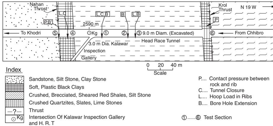
Fig. 20.8 Locations of test sections and details of instrumentation in the intra-thrust zone at Kalawar.
