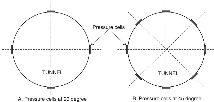
Fig. 14.4 Typical installation arrangements of pressure cells.
