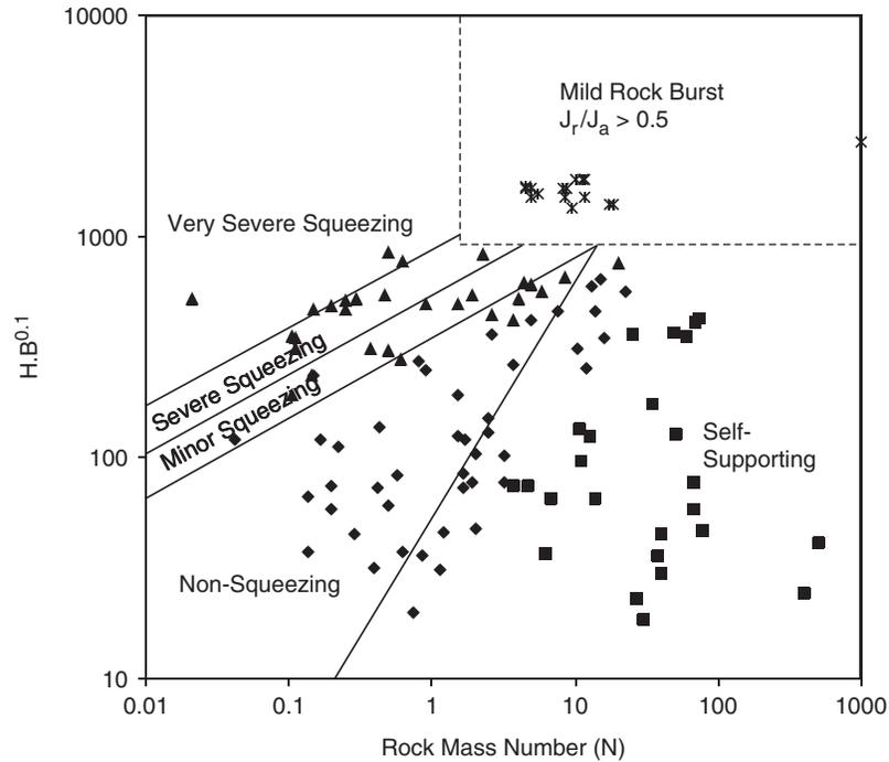
Fig. 13.1 Plot between rock mass number  $N$  and  $HB^{0.1}$  for predicting ground conditions (Goel, 1994).
