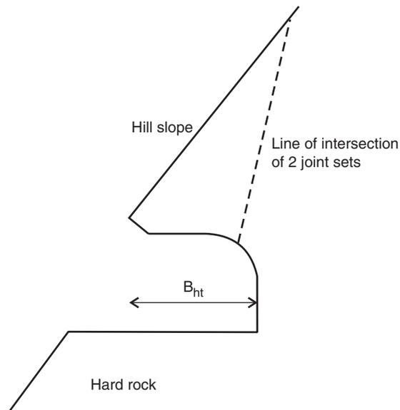
Fig. 25.3 Half tunnel along hill roads in hard rocks.
