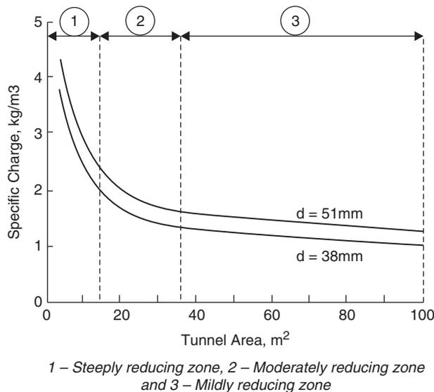
Fig. 11.7 Specific charge vs. tunnel area (Olofsson, 1988) [ $d$  = blast hole diameter].
