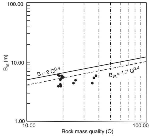
Fig. 25.2 Plot of rock mass quality  $Q$  vs span of half tunnel  $B_{ht}$ .
