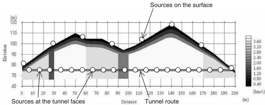
Fig. 2.6 A velocity model used in numerical tests and source location.
