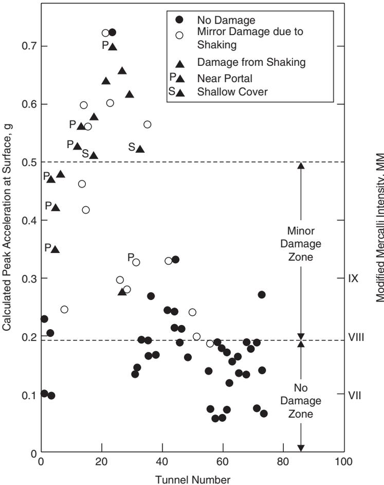
Fig. 21.1 Calculated peak acceleration at the surface and associated tunnel damage (Dowding & Rozen, 1978).
