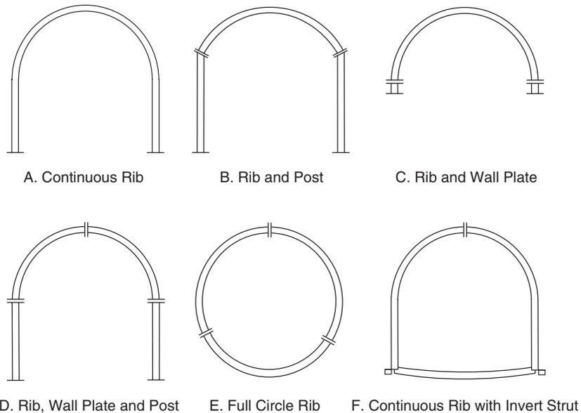
Fig. 28.9 Types of steel support system.
