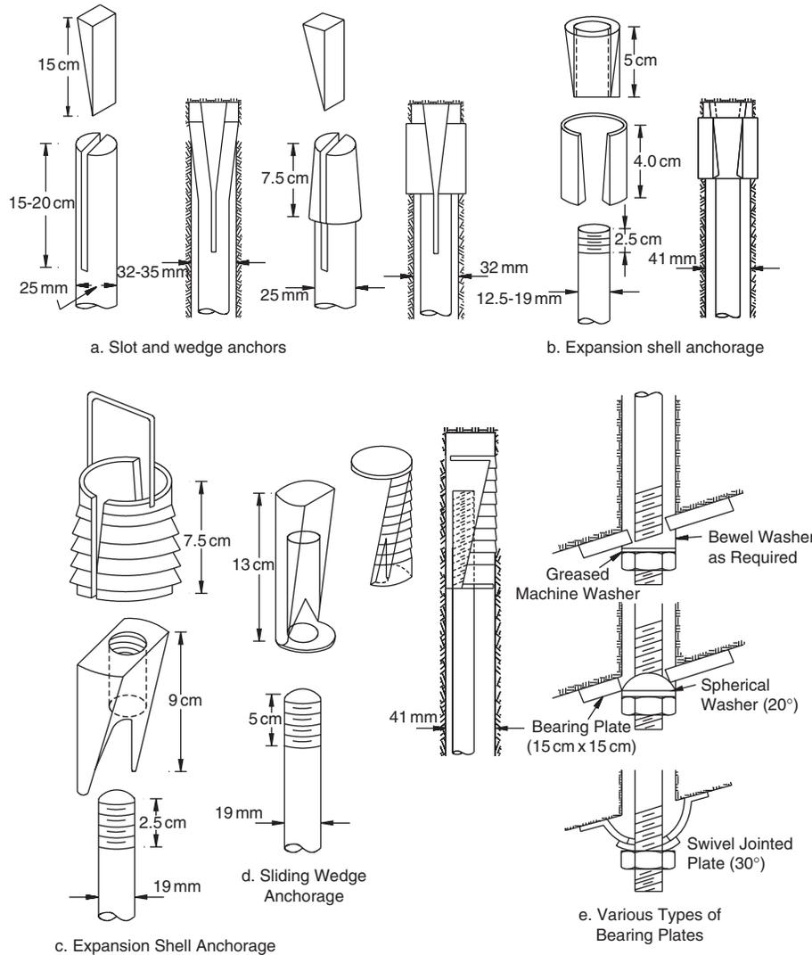
Fig. 12.3 Components of point-anchored bolts.
