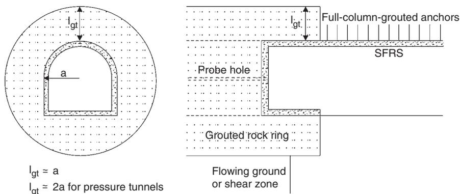
Fig. 28.20 Grouting ahead of flowing ground.
