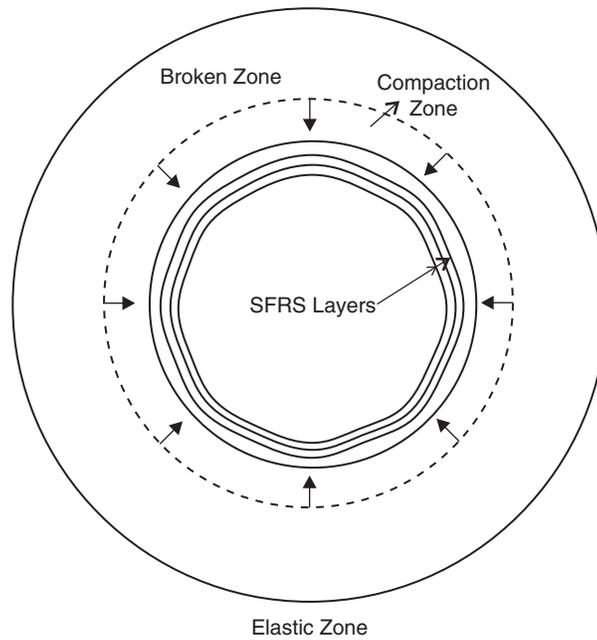
Fig. 28.4 Stabilization of broken zone in squeezing ground condition.
