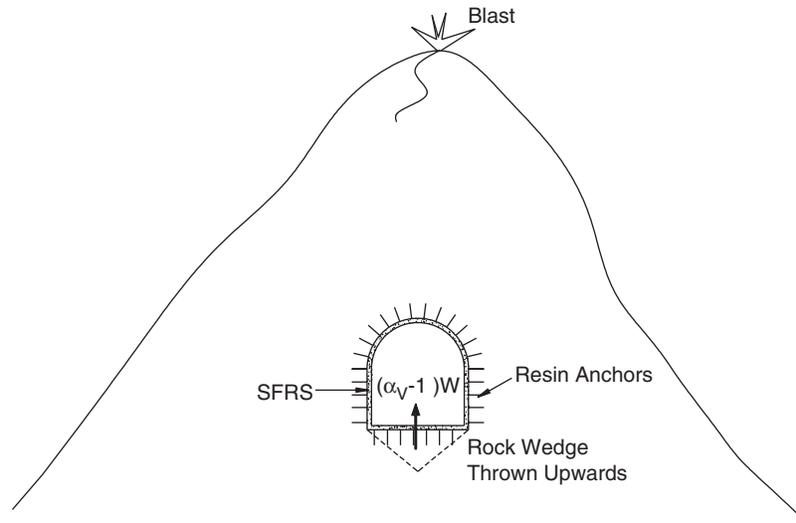
Fig. 21.3 Support system for blast loading.
