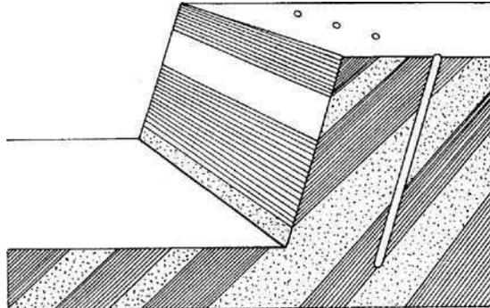
Fig. 11.5 Bench blasting with joints dipping towards the free face (Johansen, 1998). Advantages: Good forward movement of muck and reduced toe; Disadvantages: Large backbreak, poor contour and slope control problems.
