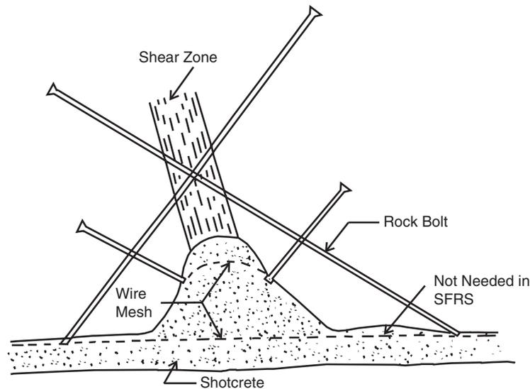
Fig. 28.5 Typical treatment of a narrow shear zone.
