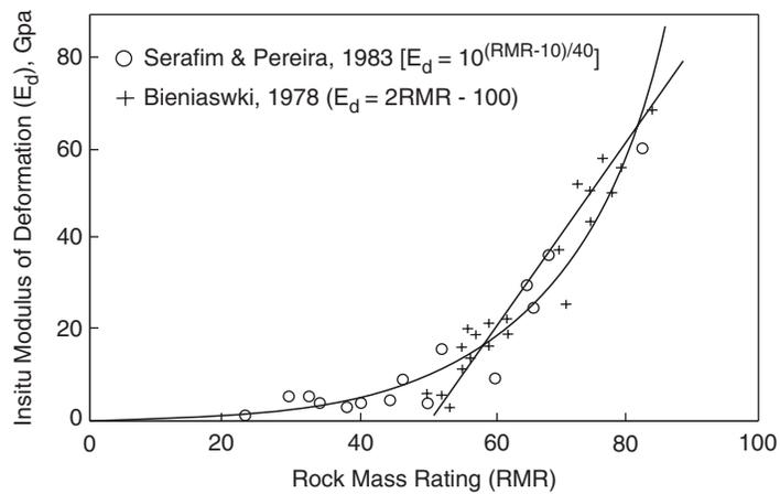
Fig. 4.3 Correlation between modulus of deformation of rock masses and RMR (Bieniawski, 1984).
