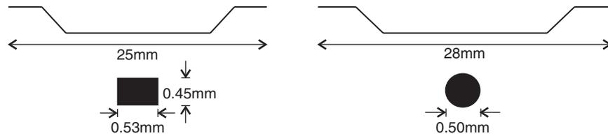
Fig. 28.2 Typical fibers used in shotcrete work.
