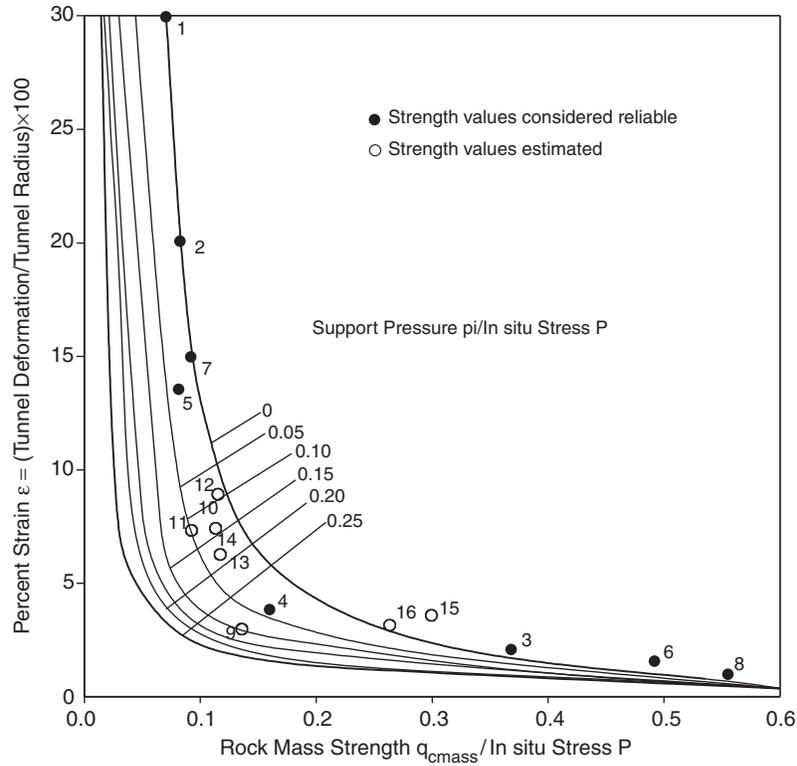
Fig. 19.8 Influence of internal support pressure  $p_i$  upon deformation of tunnels in weak ground (Numbered points are from case histories) (Hoek, 2001).
