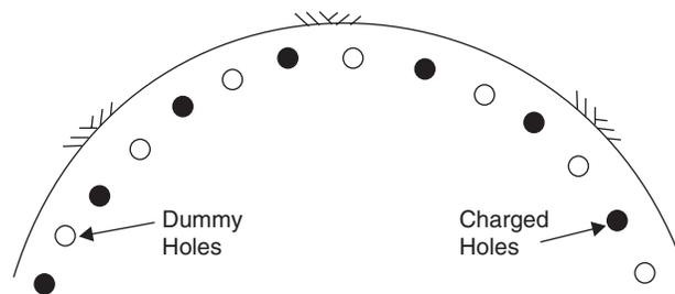
Fig. 11.11 Smooth blasting pattern with dummy holes.
