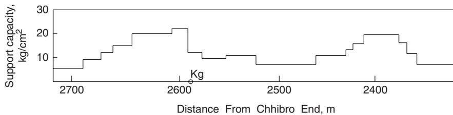
Fig. 20.9 Support density in the intra-thrust zone at Kalawar.
