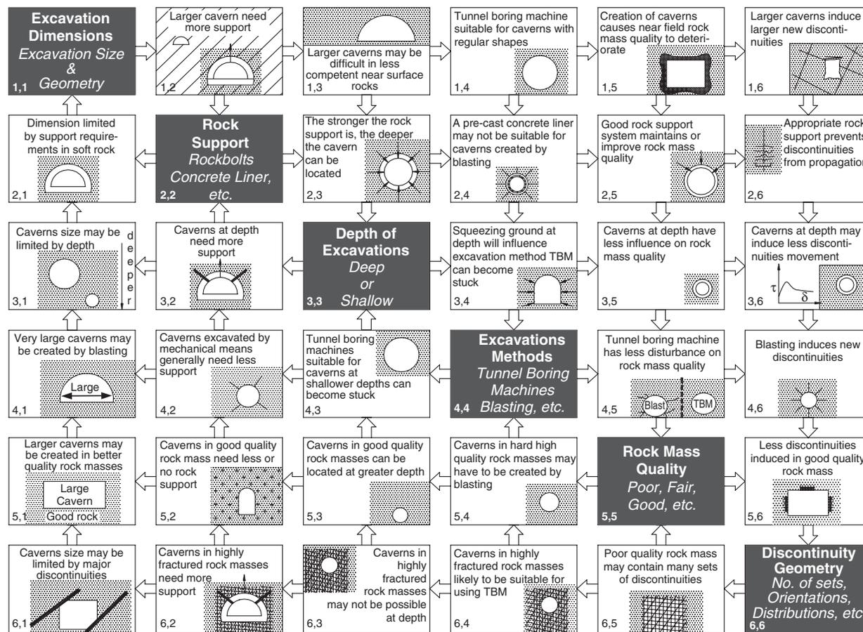
Fig. 13.2a Interaction of rock parameters in the underground excavations (Hudson, 1991).
