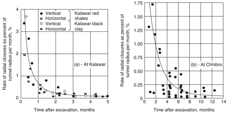
Fig. 20.16 Rate of radial tunnel closure vs. time.
