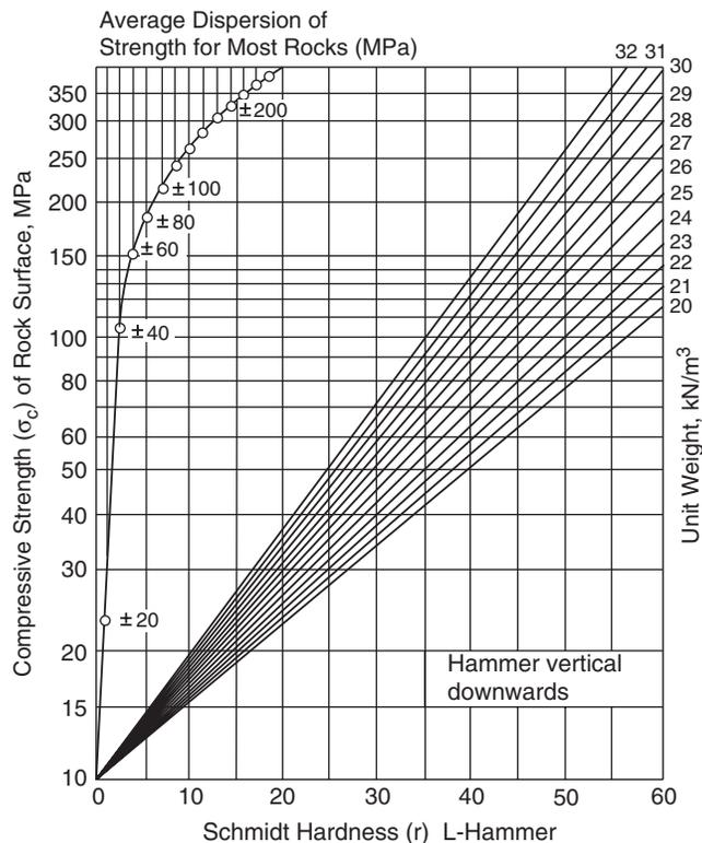
Fig. 7.4 Correlation chart for compressive strength with rock density and Schmidt hammer rebound number on smooth surfaces (Miller, 1965).
