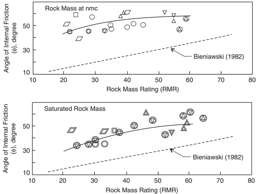
Fig. 29.5 Relationship between rock mass rating (RMR) and angle of internal friction ( $\phi_p$ ) (Mehrotra, 1992) [nmc: natural moisture content].
