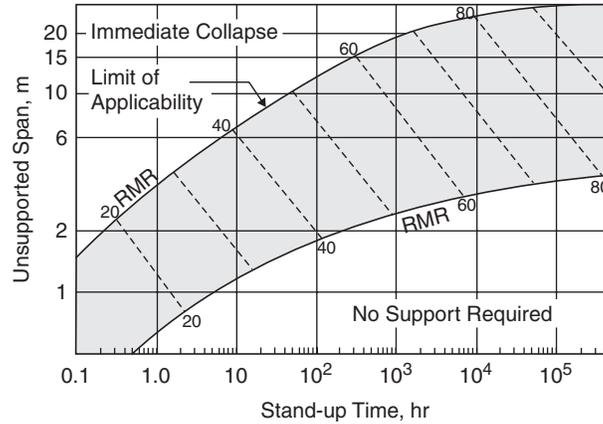
Fig. 4.1 Stand-up time vs. unsupported span for various rock mass classes as per RMR.
