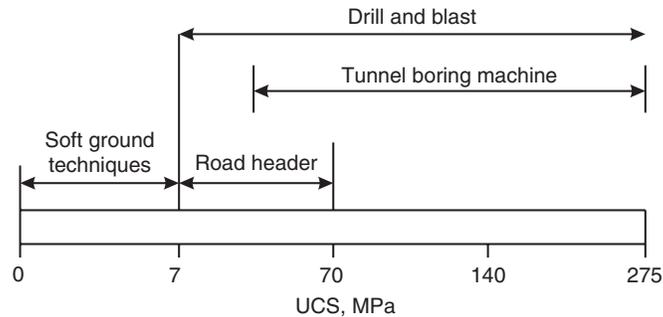
Fig. 15.1 Tunnel excavation methods as a function of rock strength (Jethwa, 2001).
