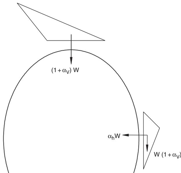
Fig. 21.2 Peak acceleration experienced by rock wedges during earthquakes.
