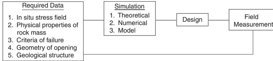
Fig. 14.1 Basic requirements for design of a structure in rock.
