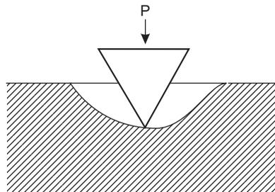
Fig. 15.3 Mechanism of failure of rock by cutter (Bickel & Kuesel, 1982).
