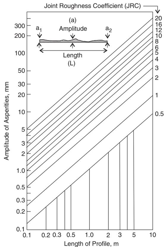
Fig. 7.2 Assessment of JRC from amplitude of asperities and length of joint profile (Barton, 1982).
