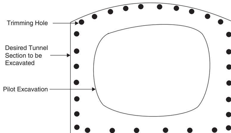
Fig. 11.12 Trimming after elimination of stress by making a pilot excavation (Calder & Bauer, 1983).
