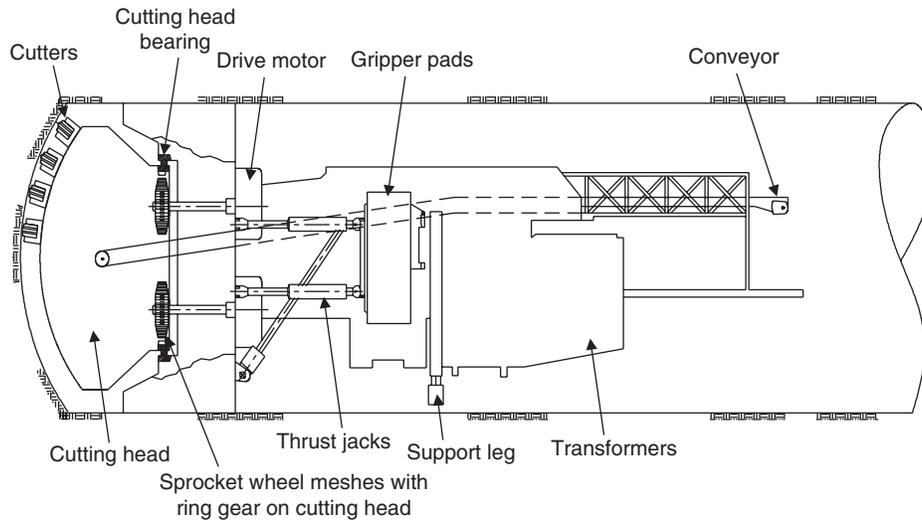
Fig. 15.4 Tunnel boring machine and ancillary equipment (Bickel & Kuesel, 1982).
