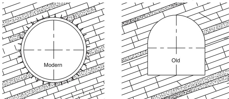
Fig. 9.2 Maintenance of original rock mass strength.
