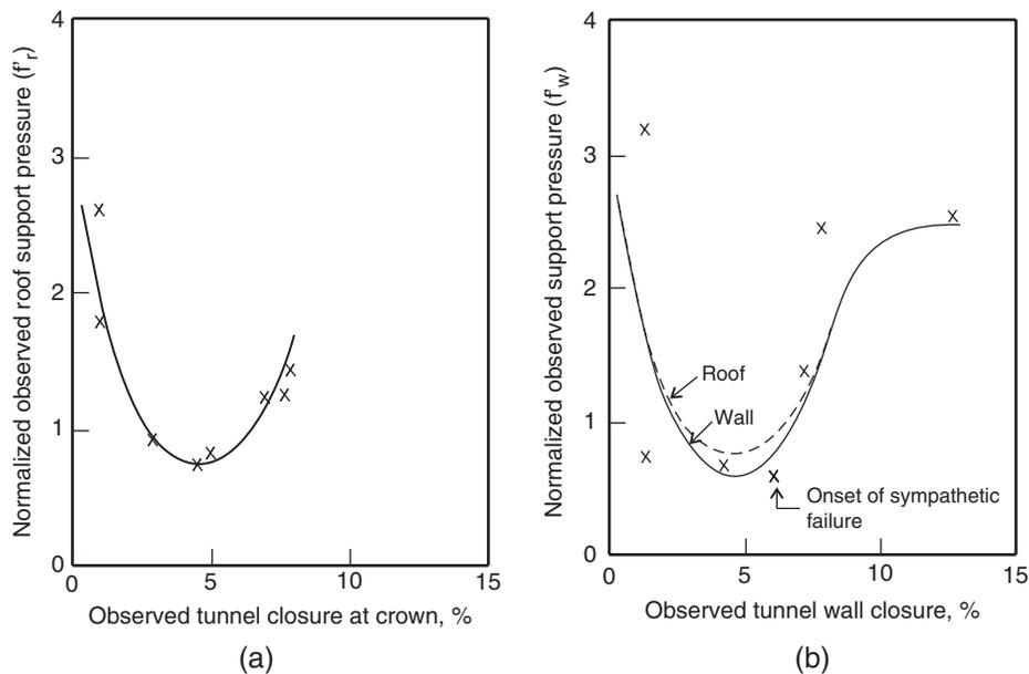
Fig. 5.4 Correction factor for (a) roof closure and (b) wall closure under squeezing ground condition (Singh et al., 1992).
