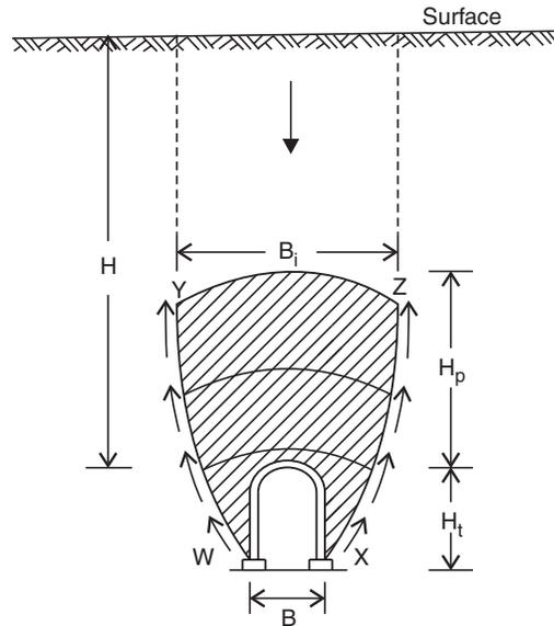
Fig. 3.1 Terzaghi's (1946) rock-load concept in tunnels.
