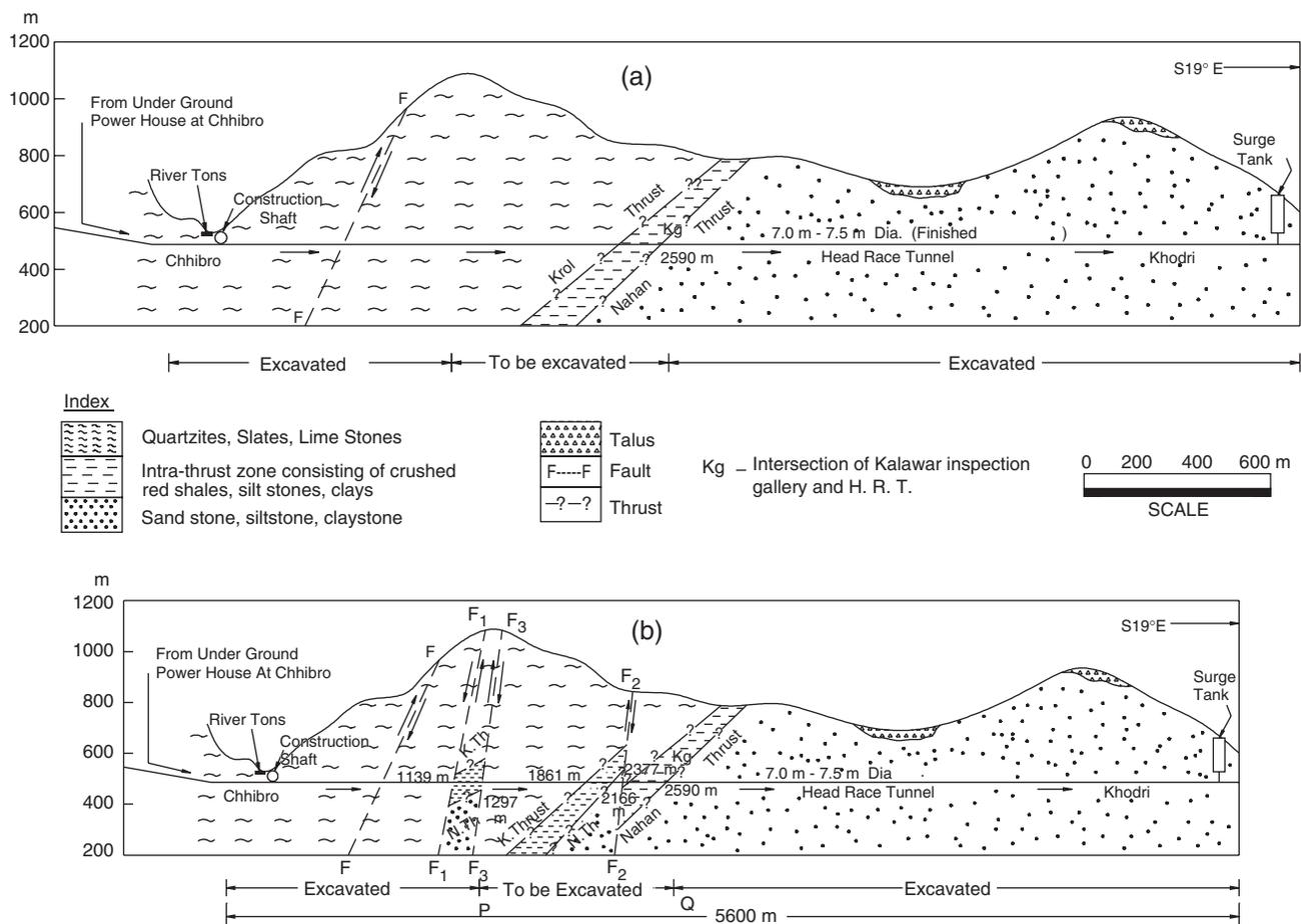
Fig. 20.2 (a) Original geological section along the Chhibro-Khodri tunnel (Auden, 1942); (b) Revised geological section along the Chhibro-Khodri tunnel (Jain et al., 1975).
