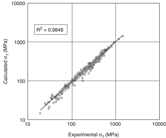
Fig. 29.2 Comparison of experimental  $\sigma_1$  values with those calculated through the proposed criterion (equation (29.1)) (Singh & Singh, 2005).
