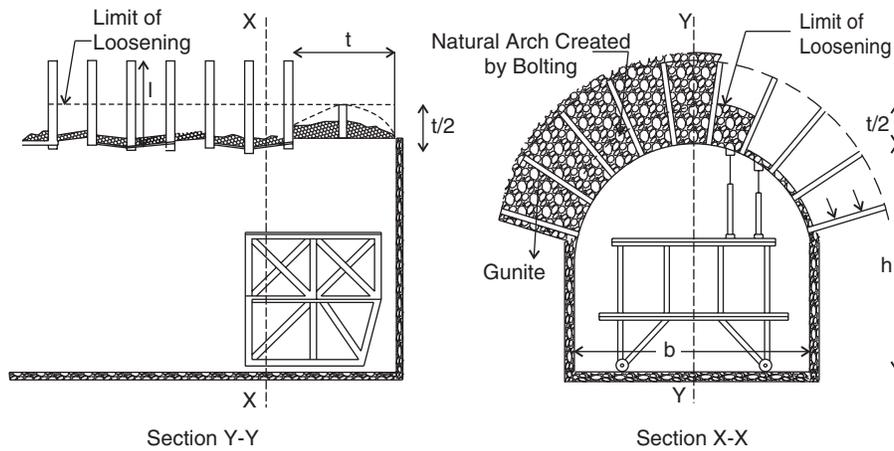
Fig. 12.13 Diagrammatic sections demonstrating principles of roof bolting.
