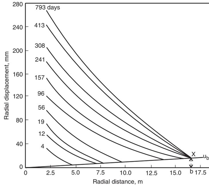
Fig. 19.1 Variation of radial displacement with radial distance within slates/phyllites of Giri Tunnel, India (Dube et al., 1986).
