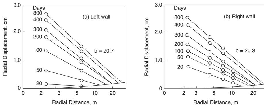
Fig. 14.9 Variation of radial displacement with radial distance within phyllites in Giri Hydeltunnel ( $a = 2.12$  m and  $b =$  radius of broken zone in squeezing ground).
