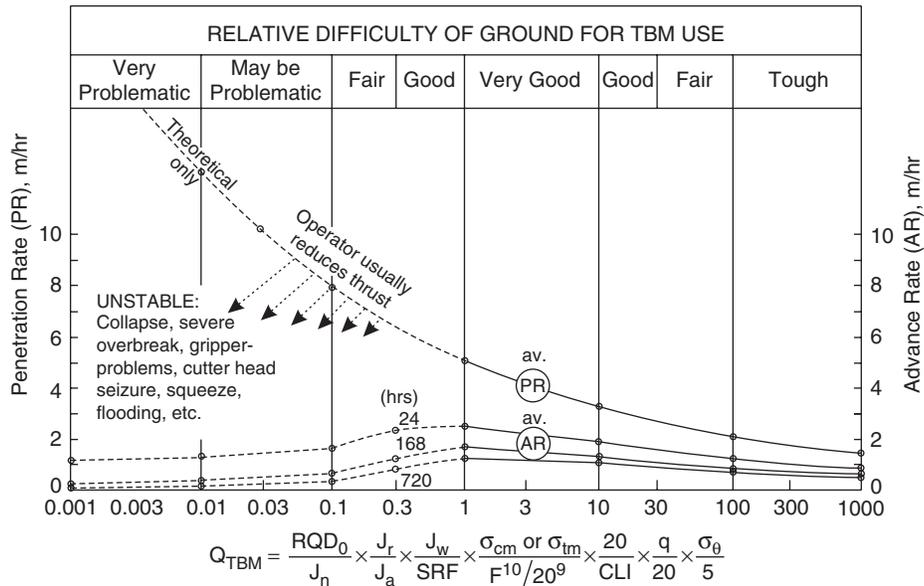
Fig. 16.2 Suggested relation between PR, AR and  $Q_{TBM}$ .
