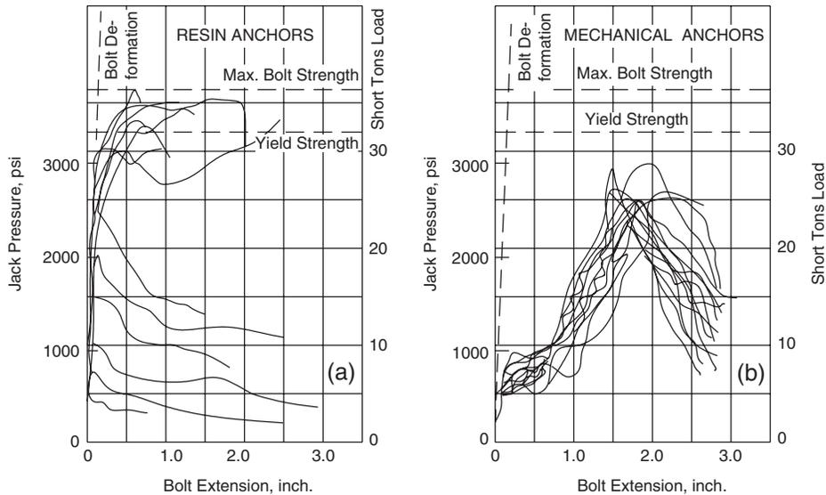
Fig. 12.7b Pull-out curves for granites (a) resin-anchored bolts, (b) mechanically anchored bolts.
