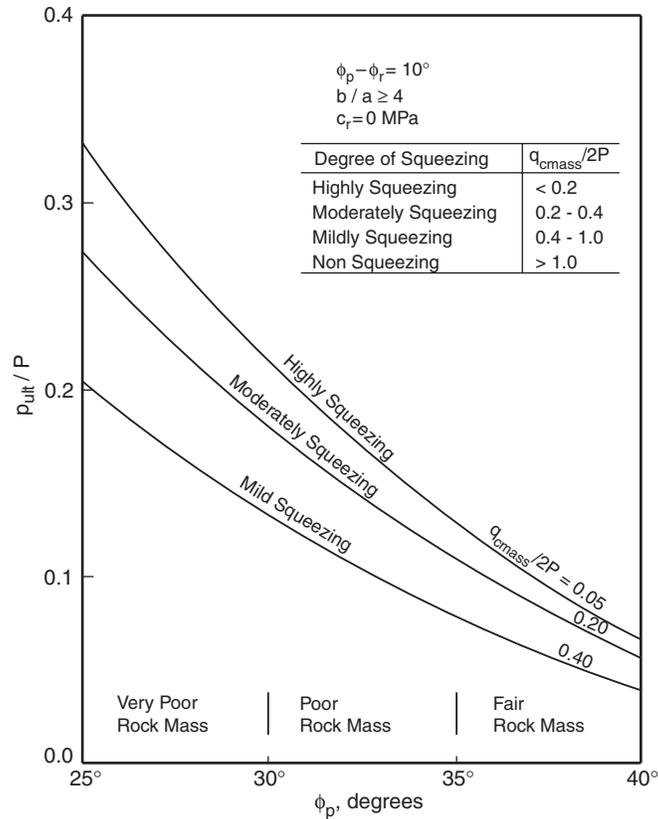
Fig. 18.1 Chart for ultimate support pressure ( $p_{\text{ult}}$ ) in squeezing ground conditions ( $P$  = overburden pressure).
