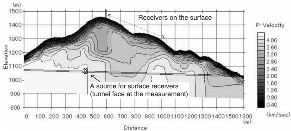
Fig. 2.13 Result of an analysis of seismic refraction data with an in-tunnel source  $\odot$ . The velocity ahead of tunnel face at distances of 500 to 900 m and elevation of 1000 to 1200 m decreases clearly, compared to results of analysis before construction (Fig. 2.10).
