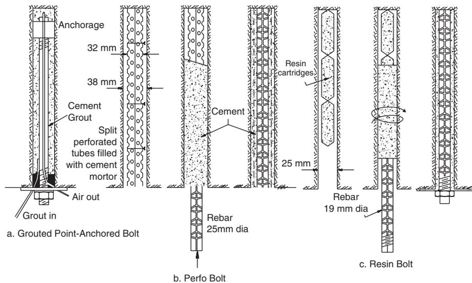
Fig. 12.4 Process of installation of grouted bolts.
