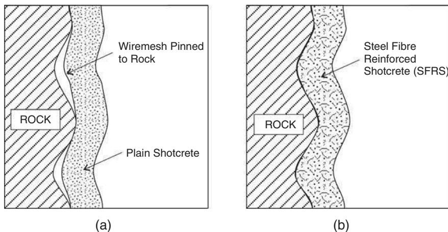
Fig. 28.1 Difference in application of shotcrete with (a) wire mesh and (b) steel fiber.
