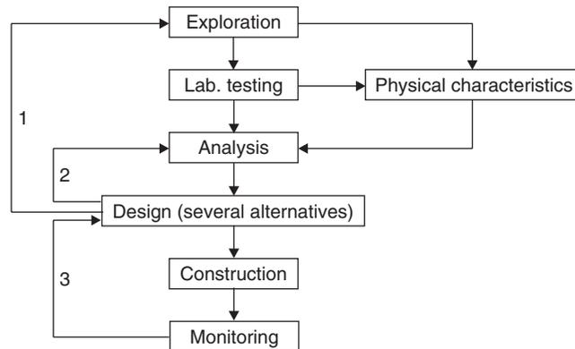
Fig. 18.4 Integrated analysis-design approach for rock structure (ISRM, 1994).
