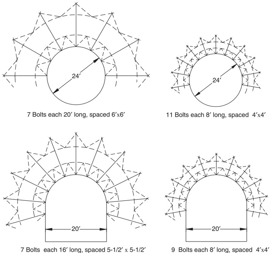
Fig. 12.11 Arch concept of rock reinforcement in circular and horse-shoe shaped tunnels (Lang, 1961).
