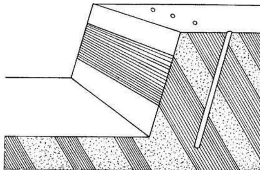
Fig. 11.6 Bench blasting with joints dipping away from the free face (Johansen, 1998). Advantages: Small backbreak; Disadvantages: Restricted forward movement, tight muck pile and increased toe.
