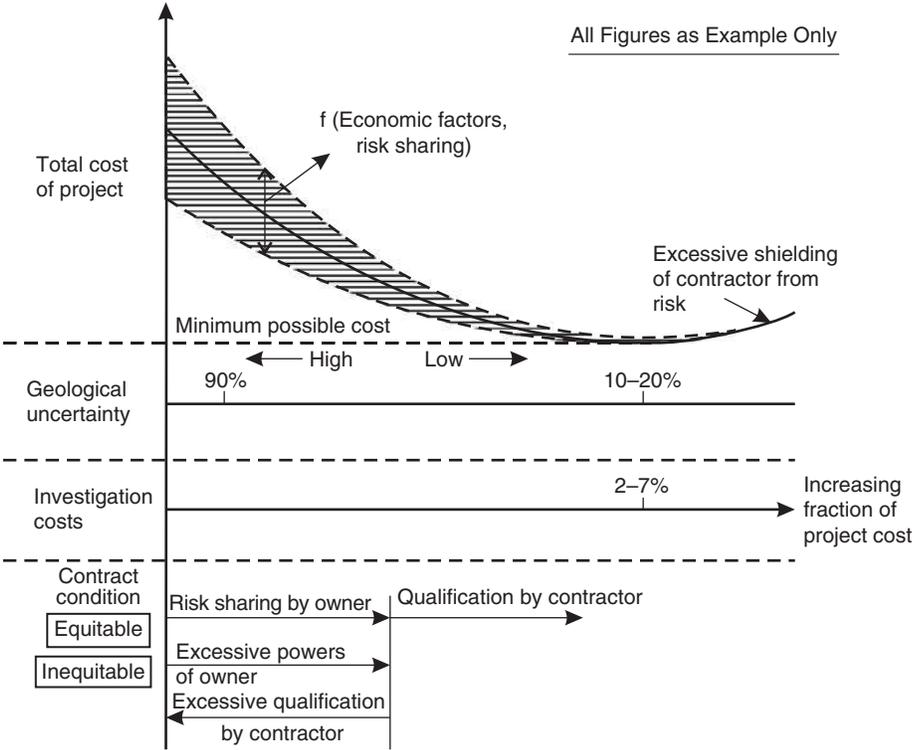
Fig. 26.4 Features of minimizing project cost (Sutcliffe, 1972).
