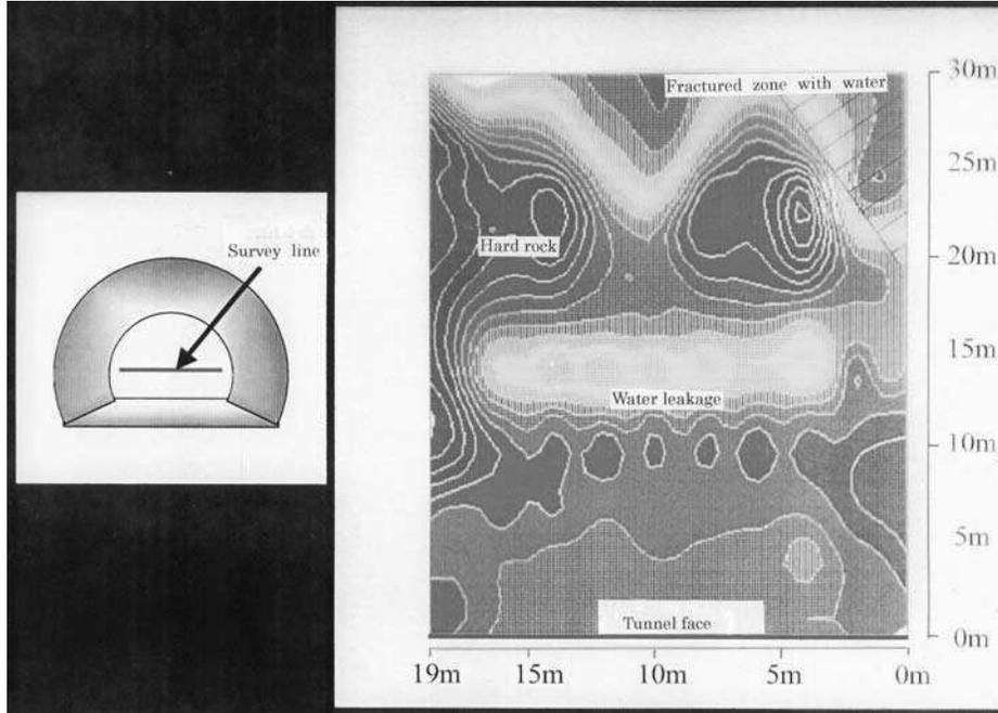
Fig. 2.3 Inversion result of electromagnetic survey for looking ahead of tunnel face.
