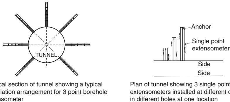
Fig. 14.5 Typical installation arrangements of multi-point (3 points shown) and single point borehole extensometers.
