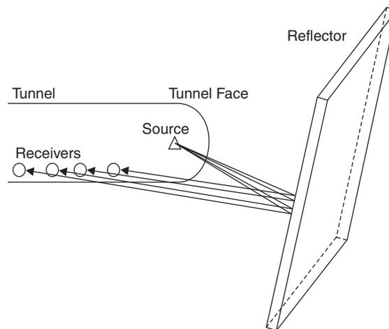
Fig. 2.2 Schematic map of data acquisition ahead of a tunnel face.
