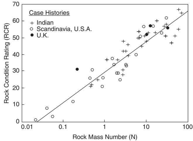
Fig. 6.2 Correlations between  $N$  and RCR (Goel et al., 1995b).
