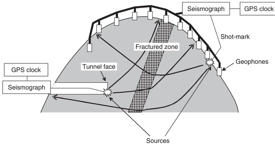
Fig. 2.5 Schematic diagram of data acquisition. Sources are placed not only on the ground surface but also within a tunnel under construction (Hayashi & Saito, 2001).
