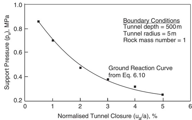
Fig. 6.3 Ground reaction curve obtained from equation (6.10).
