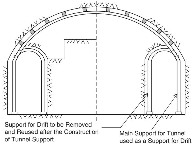
Fig. 28.10 Side drift method.
