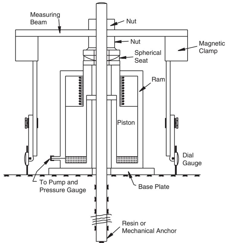
Fig. 12.7a Rock bolt testing equipment (Franklin and Woodfield, 1971).
