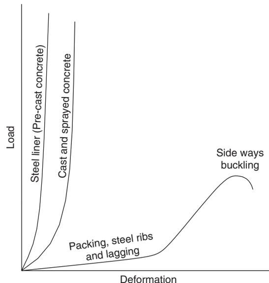
Fig. 20.14 Load-deformation characteristics of some support system (Ward, 1978).
