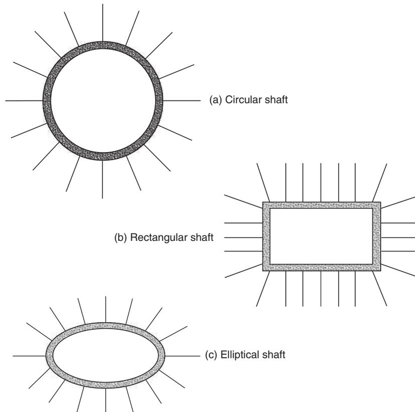
Fig. 24.1 Shapes of shafts in rock masses.
