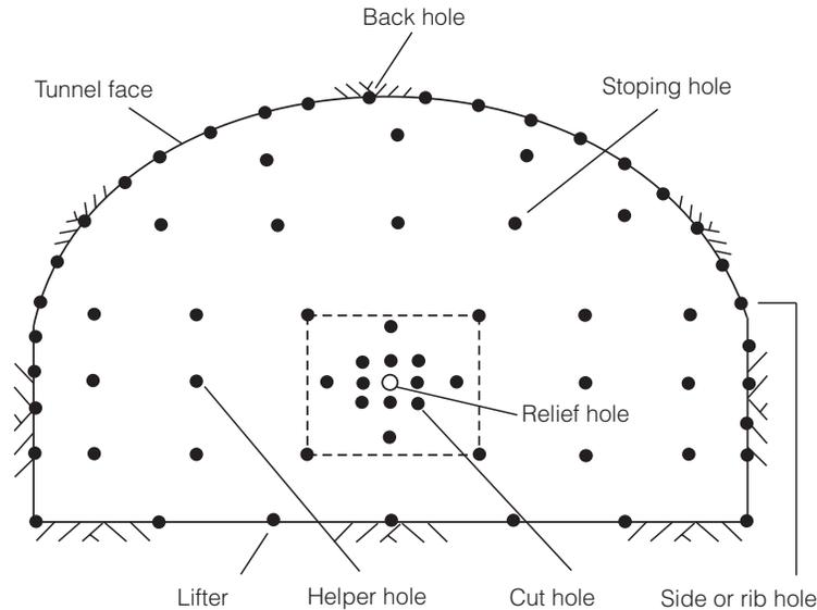
Fig. 11.1 Nomenclature of blast holes in different parts of a tunnel section (Rustan, 1998).
