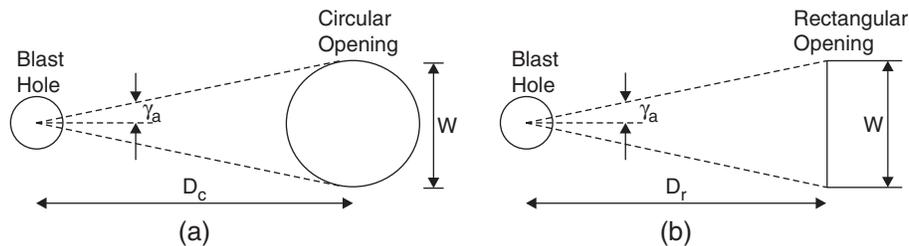
Fig. 11.10 Plan view of blasting towards narrow opening (a) circular and (b) rectangular (Langefors & Kihlstrom, 1973).
