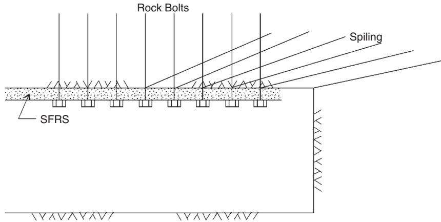
Fig. 28.3 Arrangement of spiling dowel with the advancement of tunnel face.
