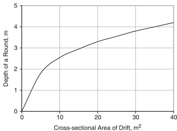
Fig. 11.9 Depth of a blast round vs. tunnel size in Germany (Ziegler, 1985).
