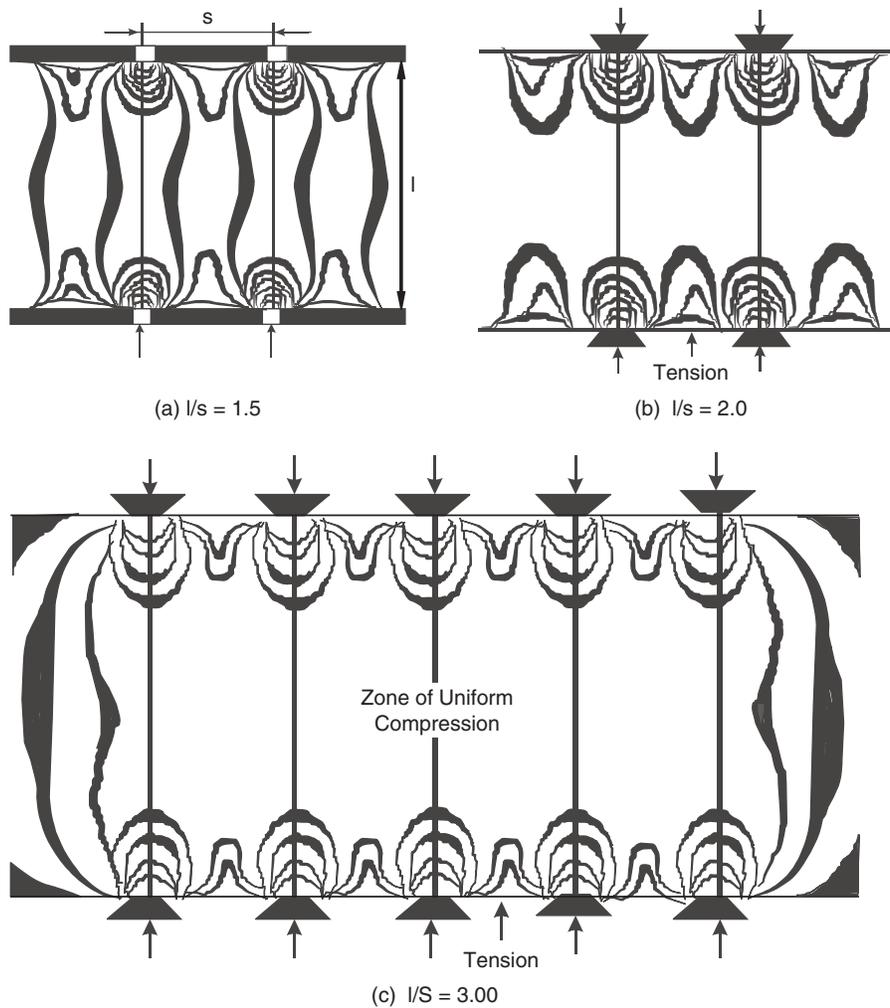
Fig. 12.9 Rock bolt – photoelastic stress pattern (Lang, 1961).
