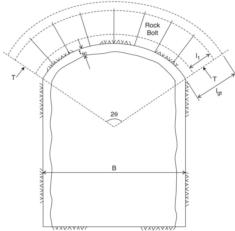
Fig. 28.17 Capacity of reinforced rock arch.
