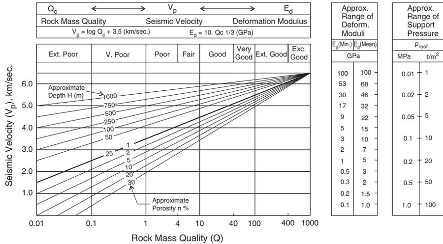
Fig. 5.5 An integration of  $V_p$ ,  $Q$ ,  $q_c$ , depth, porosity and static deformation modulus  $E_d$  which was developed stage by stage by trial and error fitting to field data (Barton, 2002).
