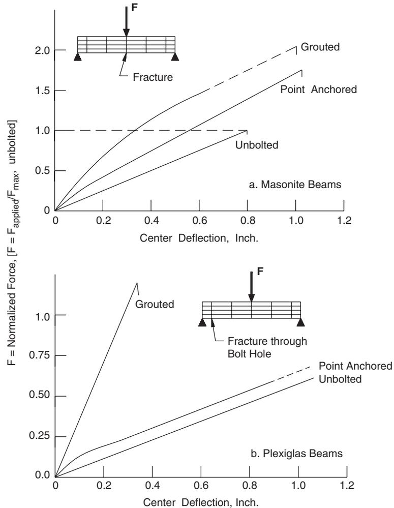
Fig. 12.8 Load deflection results from model rock bolting tests (Fairhurst and Singh, 1974).
