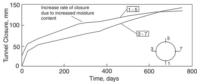
Fig. 14.6 Tunnel closure as a function of time.
