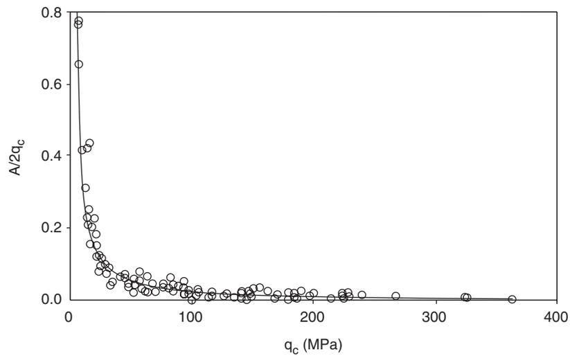
Fig. 29.4 Variation of parameter  $A/2q_c$  with UCS of the intact rocks ( $q_c$ ).
