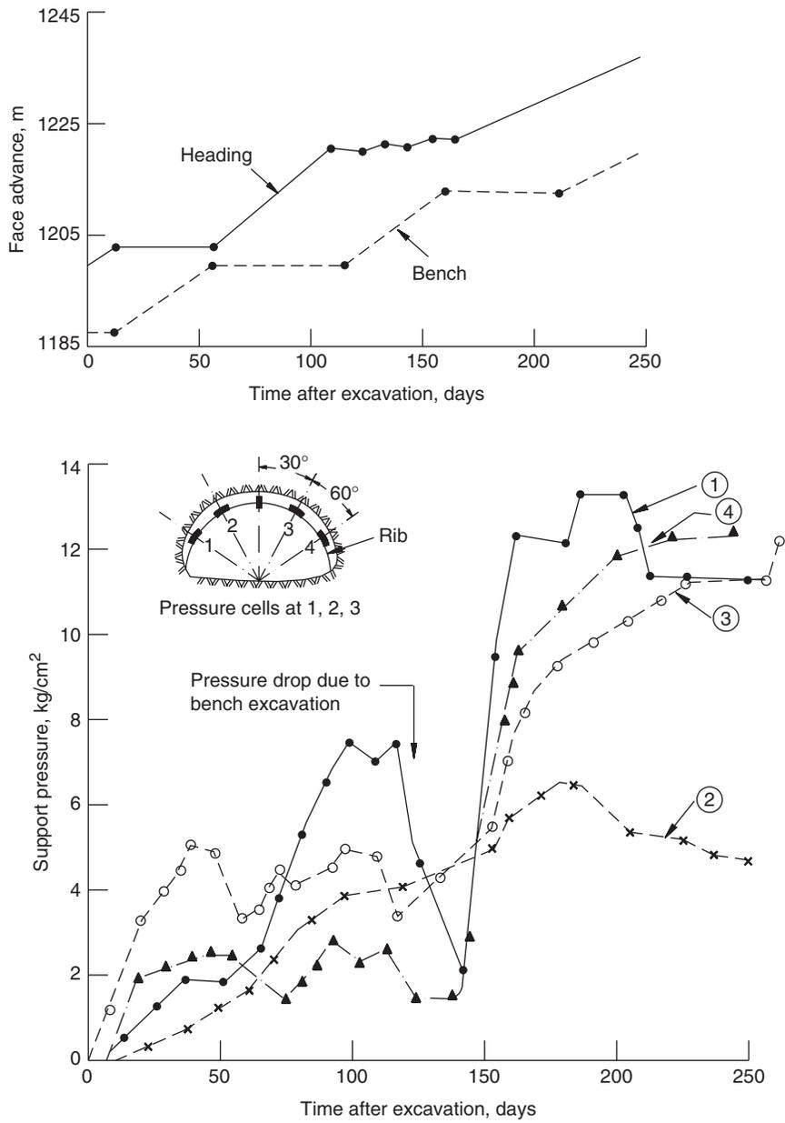
Fig. 20.12 Support pressure vs. time in red shales at Chhibro.
