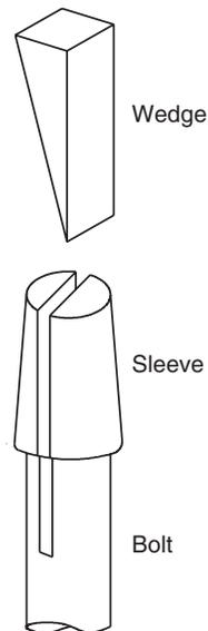
Fig. 28.7 Wedge and sleeve bolt.
