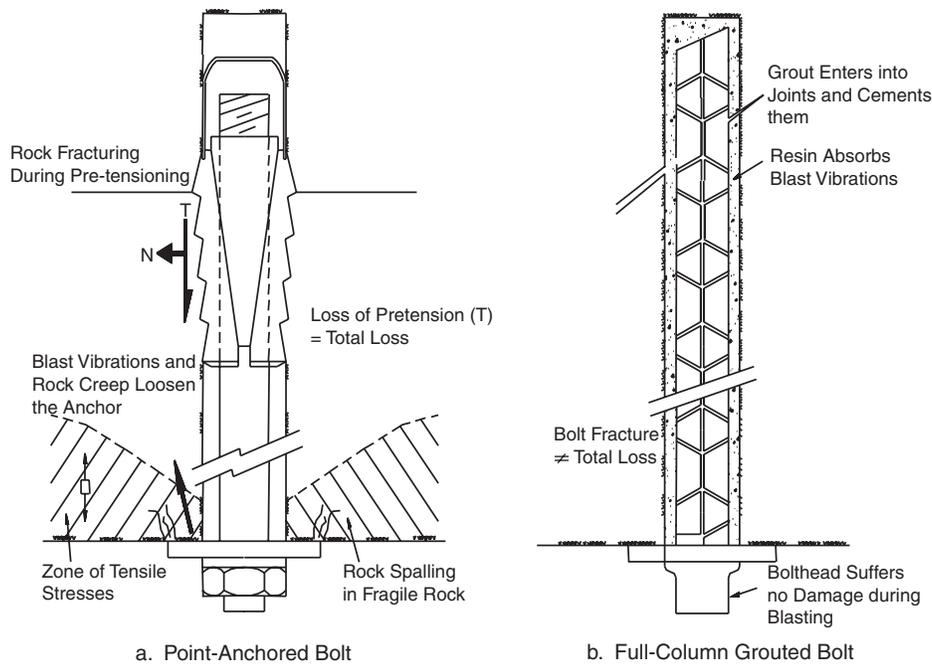
Fig. 12.1 Comparison of point-anchored and grouted bolts.
