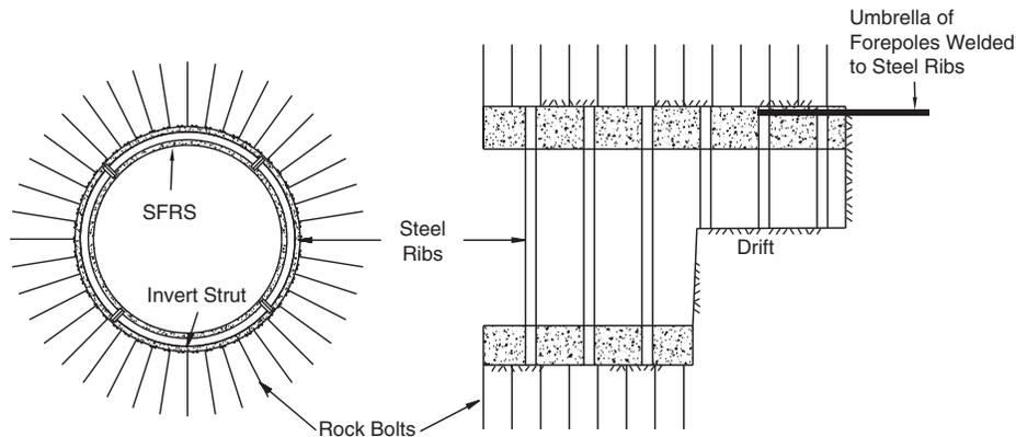
Fig. 19.9 Support system in severe squeezing ground condition.
