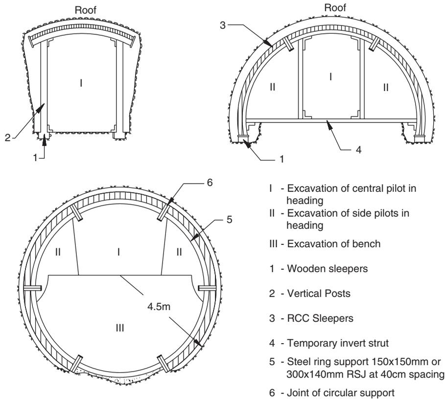
Fig. 20.7 Sequence of excavation and support for the main tunnel through the intra-thrust zone at Kalawar.
