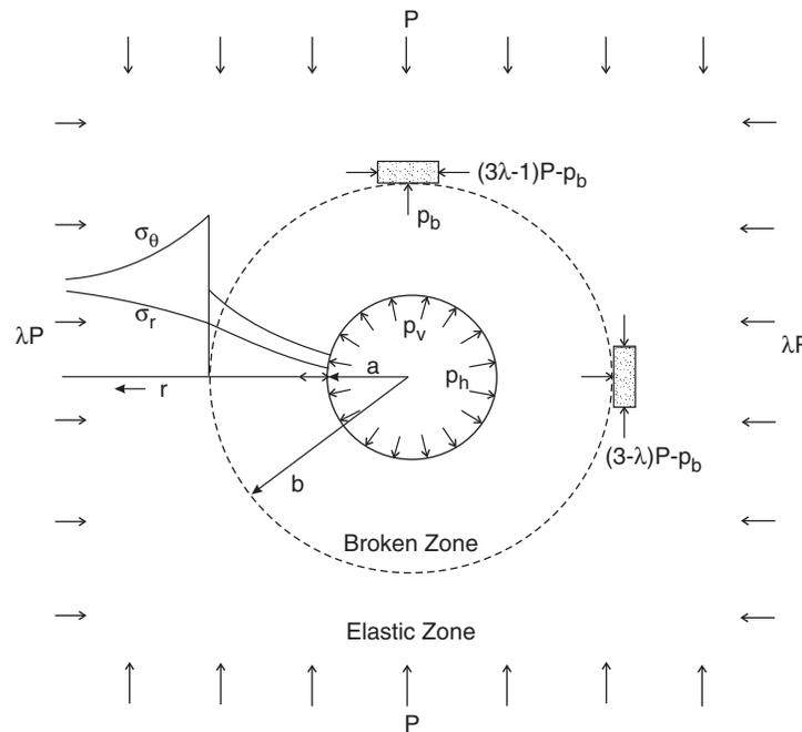
Fig. AI.3 Stress distribution in squeezing ground.
