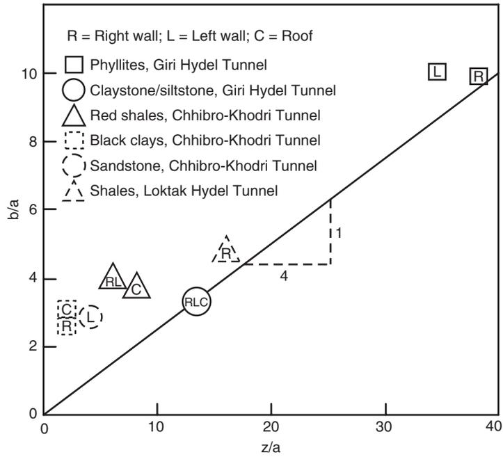
Fig. 19.4 Face advance ( $z$ ) for stabilization of broken zone ( $b$ ).
