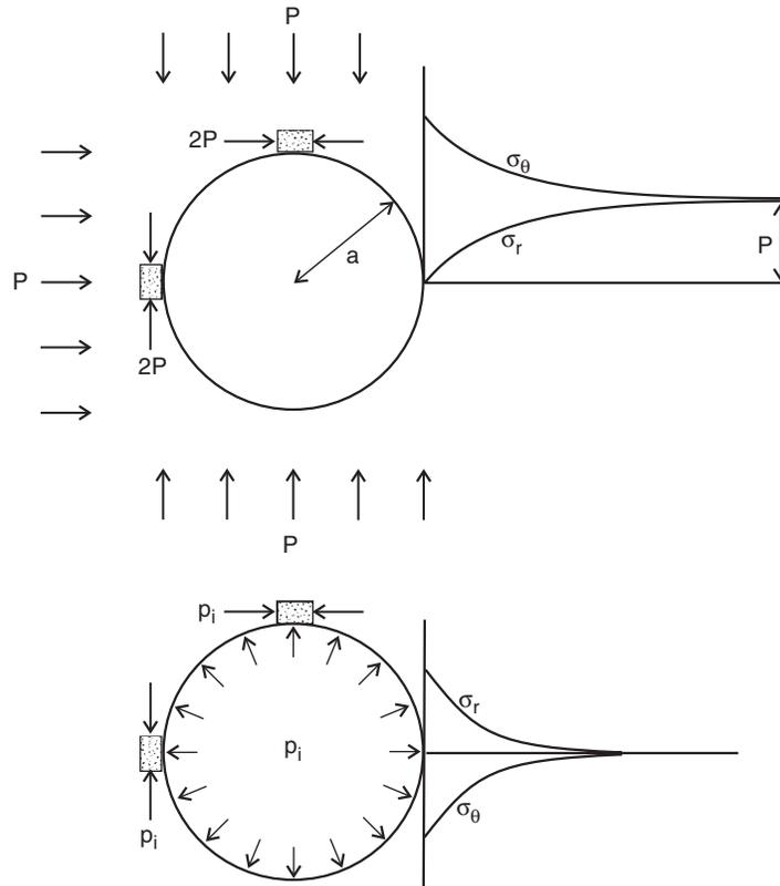
Fig. AI.2 The stress distribution around circular tunnel in hydrostatic stress condition and plain strain condition.
