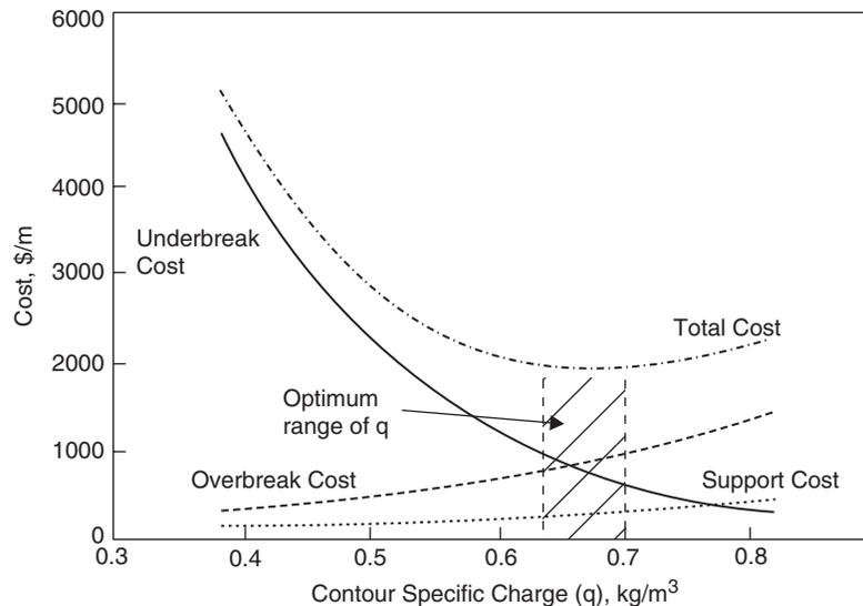
Fig. 11.13 Optimization of contour specific charge in terms of cost (Ibarra et al., 1996).
