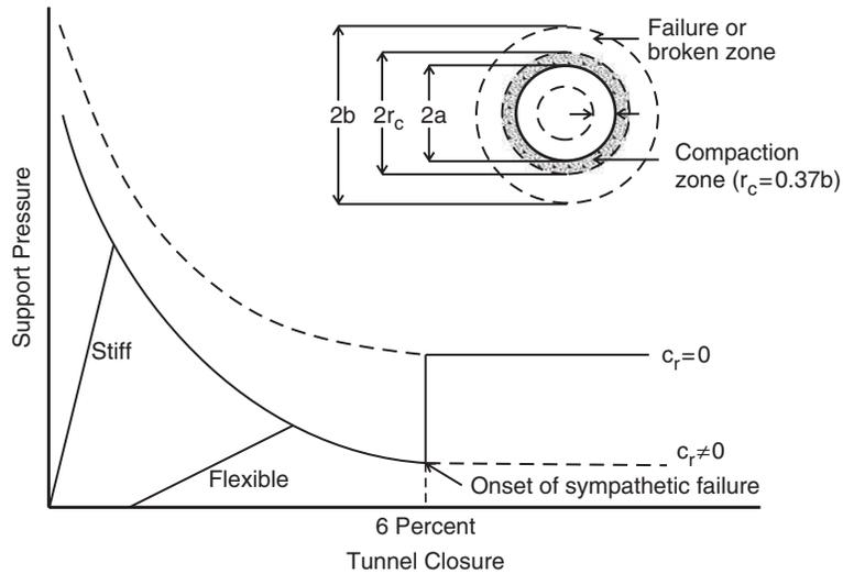
Fig. 19.5 Effect of sympathetic failure of rock mass on theoretical ground response curve of squeezing ground condition. Support reaction curve of stiff and delayed flexible supports are superposed.
