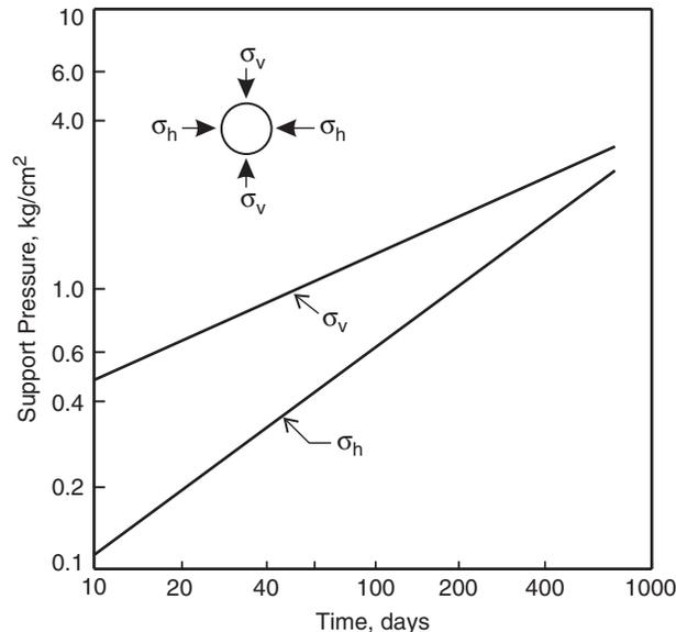
Fig. 18.3 Observed support pressure vs. time in black clays, Yamuna project (3.0 m diam. tunnel).
