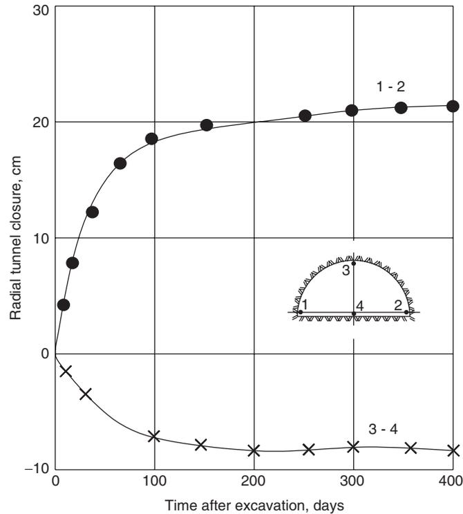
Fig. 20.13 Radial tunnel closure vs. time in red shales at Chhibro.
