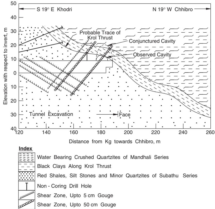
Fig. 20.3 Geological features causing flooding of tunnel at Kalawar (Shome et al., 1973).
