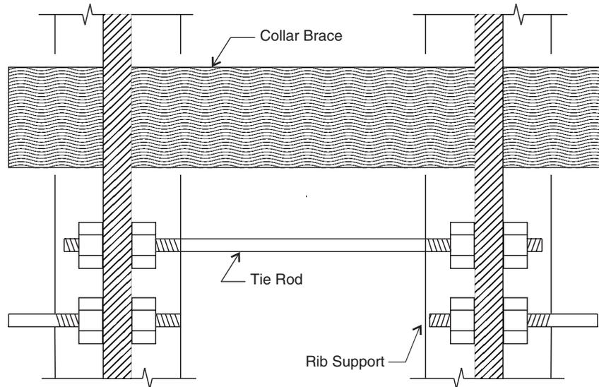
Fig. 28.15 Collar brace and tie rod.
