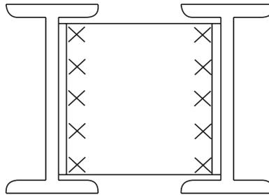
Fig. 28.11 Double beam wall plate.
