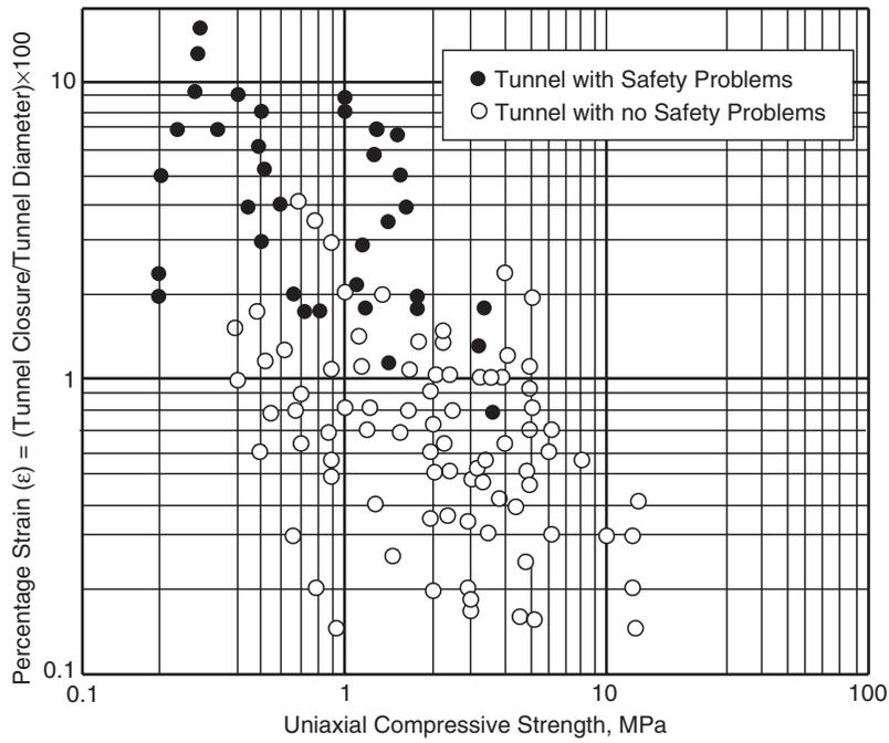
Fig. 19.6 Field observations by Cheru et al. (1998) from second Freeway, Pinglin and New Tienlun Headrace Tunnels in Taiwan.
