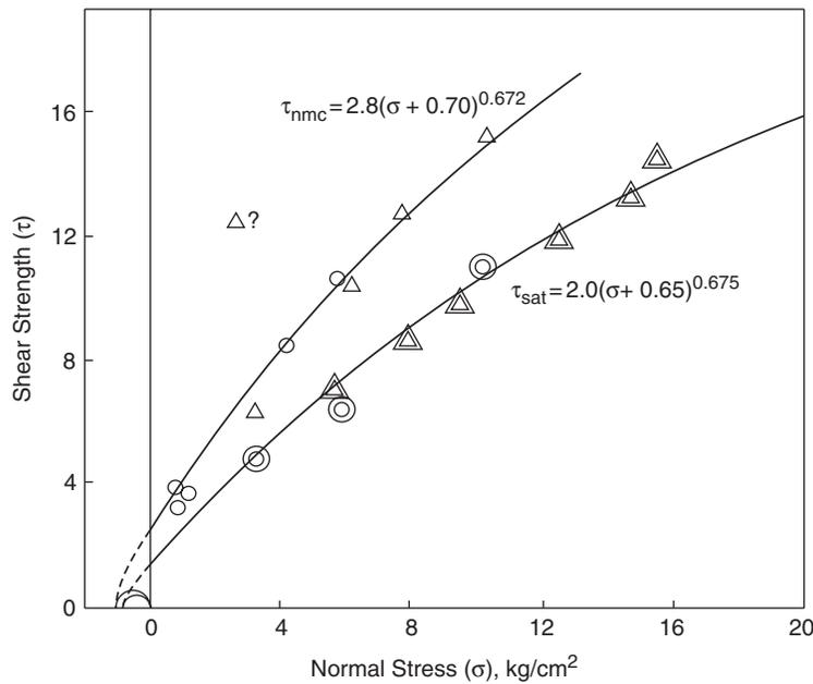
Fig. 8.3 Estimation of tensile strength of rock mass from Mohr's envelope (Mehrotra, 1992).
