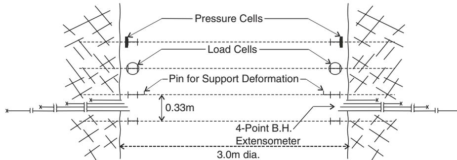
Fig. 14.11 Layout plan of a typical instrumentation zone.
