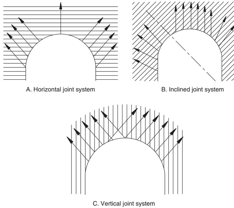
Fig. 12.12 Roof bolting in strata having various dip angles.
