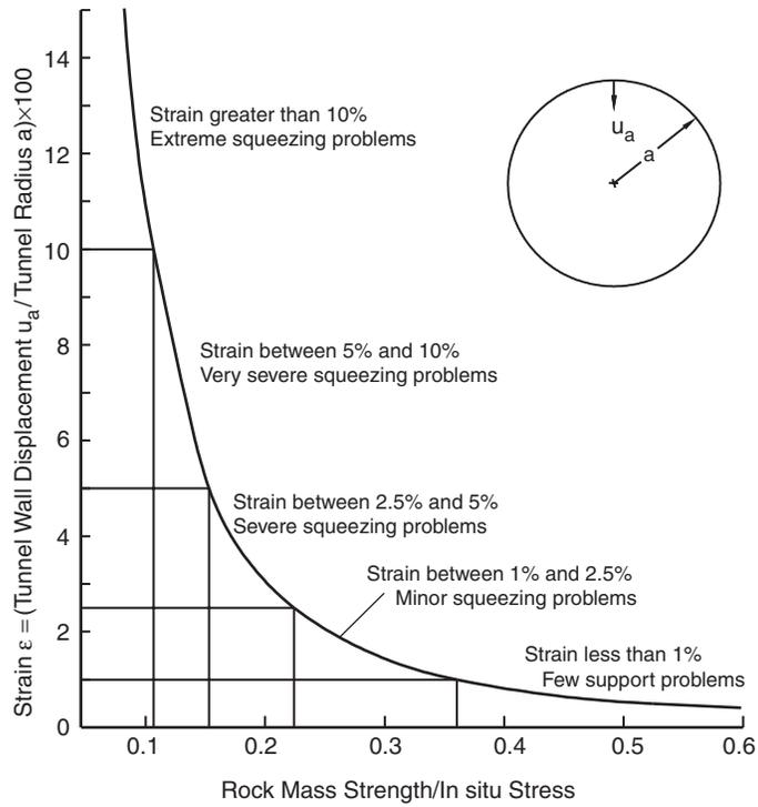
Fig. 19.7 Tunnelling problems associated with different levels of strain (Hoek, 2001).
