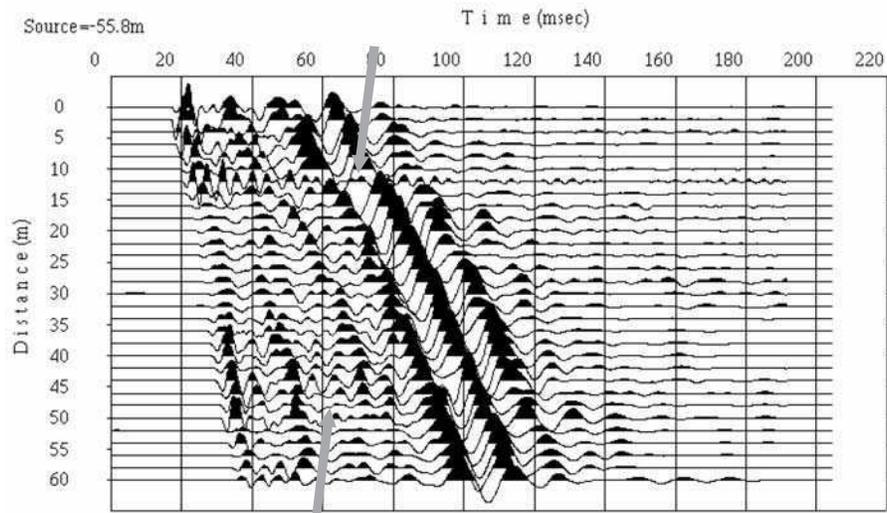
Fig. 2.11 A raw shot gather data of the in-tunnel seismic reflection method. A source was placed 55.8m away from a receiver array (© in Fig. 2.10). Big arrows indicate reflected waves from a reflector ahead of the tunnel face.
