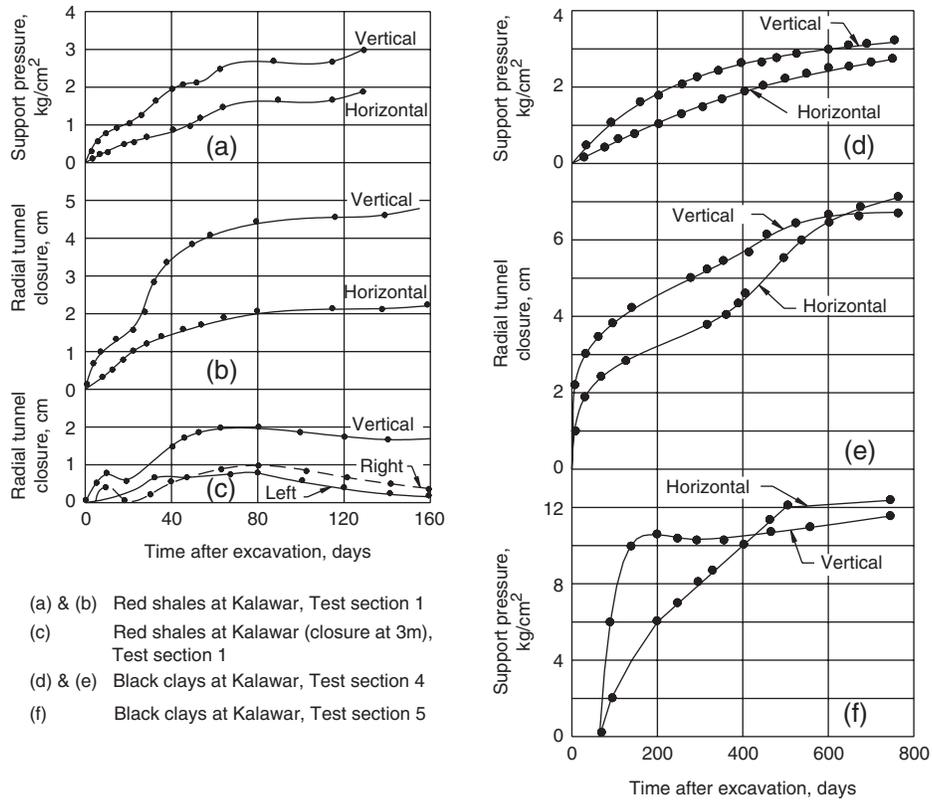
Fig. 20.10 Monitoring of support pressure and radial tunnel closure in red shales and black clays in different instrumentation test sections at Kalawar.
