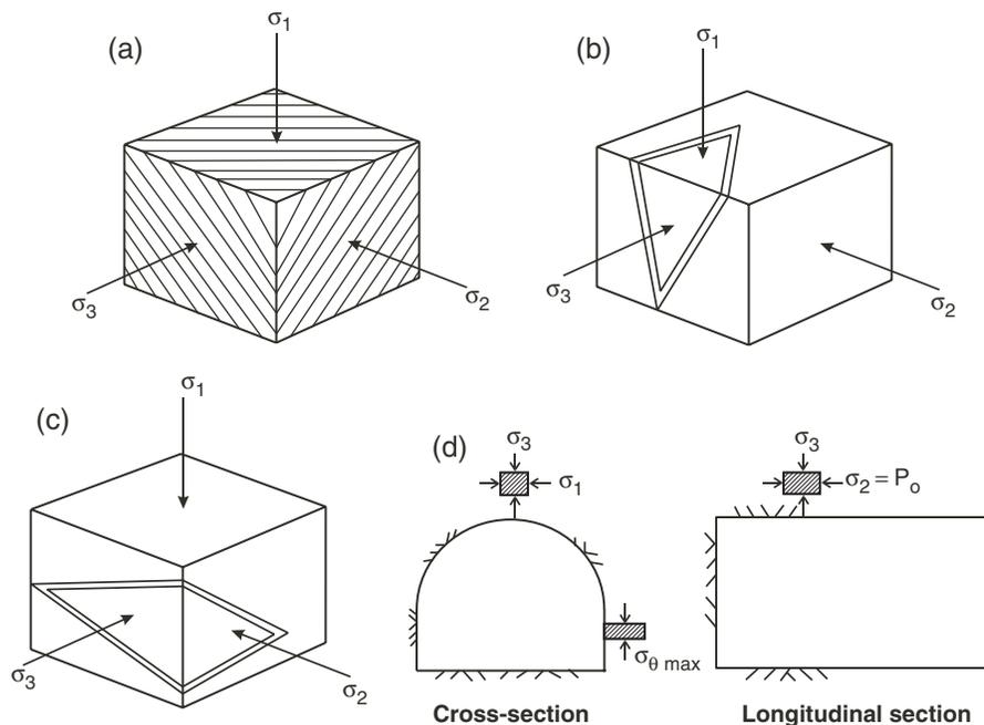
Fig. 8.1 (a) Anisotropic rock material with one joint set (slate, schist, etc.), (b) mode of failure in rock mass with 2 joint sets, (c)  $p_{\text{horizontal}} \gg p_{\text{vertical}}$  and (d) direction of  $\sigma_1$ ,  $\sigma_2$  and  $\sigma_3$  in the tunnel.
