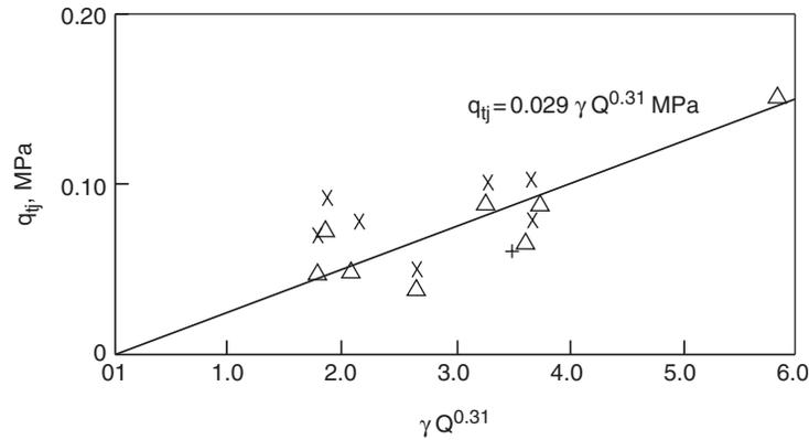
Fig. 8.4 Plot between  $q_{tj}$  and  $\gamma \cdot Q^{0.31}$ .
