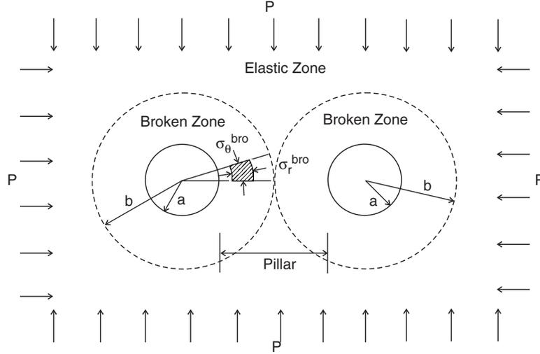
Fig. AI.4 Stresses on the pillar between two adjacent tunnels in squeezing ground condition.
