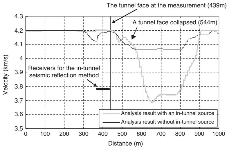
Fig. 2.14 Seismic velocity along a tunnel route. A thick line indicates result of an analysis with an in-tunnel source. A thin line indicates result of an analysis without in-tunnel sources.
