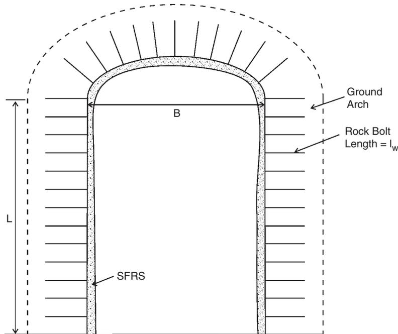
Fig. 28.18 Design of wall reinforcement of caverns.
