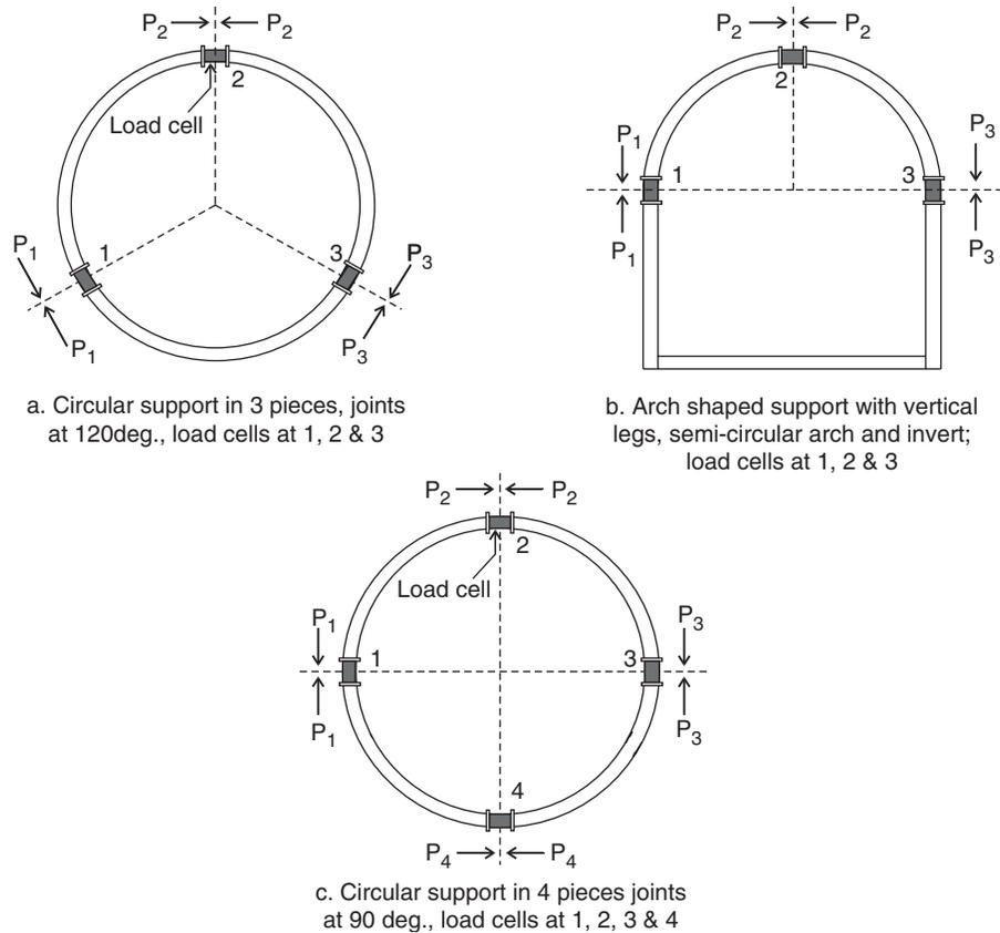
Fig. 14.3 Typical installation arrangements of load cells.
