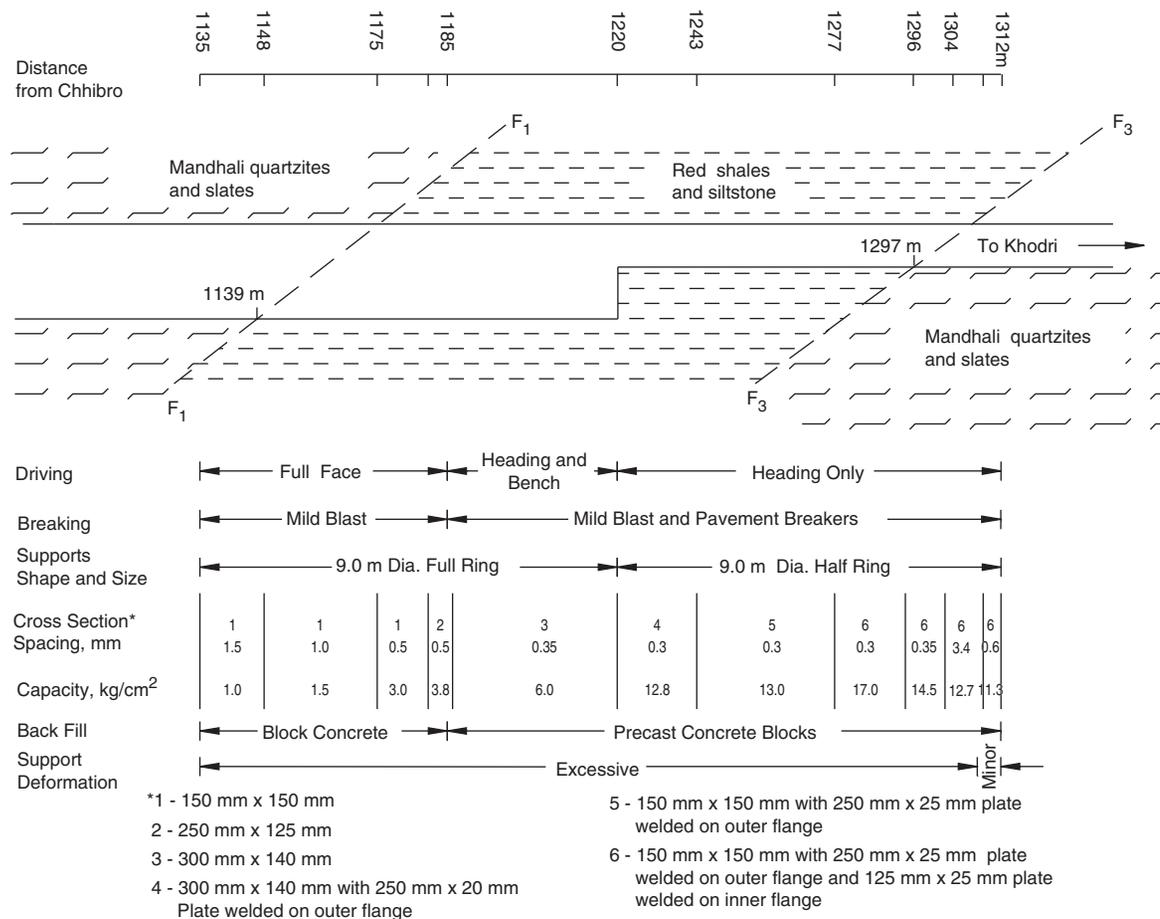
Fig. 20.11 Geological plan and construction details of head race tunnel through intra-thrust zone at Chhibro.
