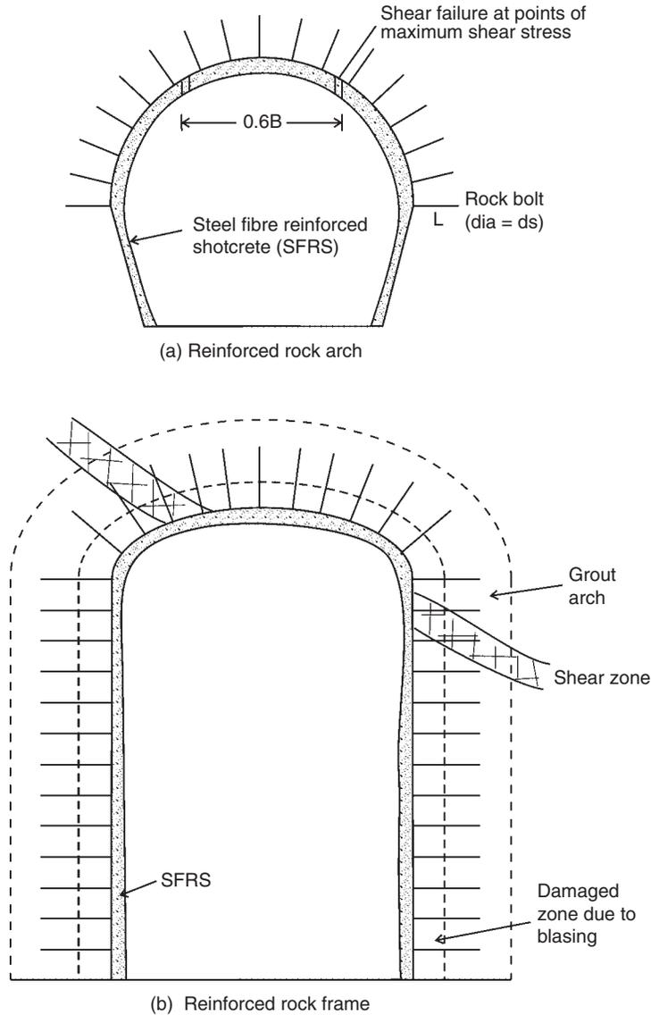
Fig. AII.1 Design of support system for underground openings.
