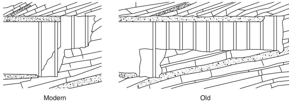
Fig. 9.12 Behavior of the rock will be influenced by the delay of ring closure, advanced crown, increase delay, bending effect on the crown and increasing loads on the rock foundation.
