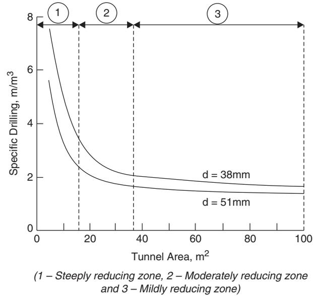
Fig. 11.8 Specific drilling vs. tunnel area (Olofsson, 1988) [ $d$  = blast hole diameter].
