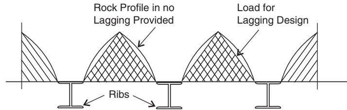
Fig. 28.16 Loading diagram for lagging.
