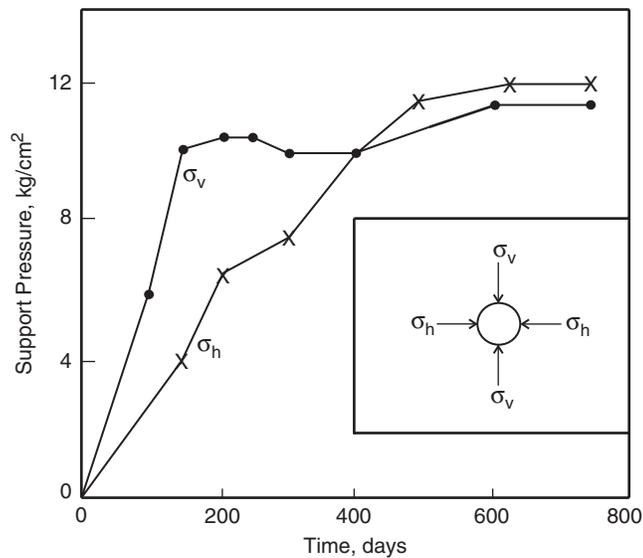
Fig. 18.2 Observed support pressure vs. time in black clays, Yamuna project (9.0 m diam. tunnel).
