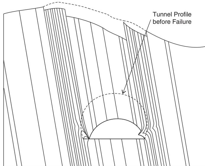
Fig. 19.2 Squeezing failures occur first at the sidewalls for a tunnel (the bedding spacing is 0.5 m and dip angle is  $80^\circ$ ) [Hsu et al., 2004].
