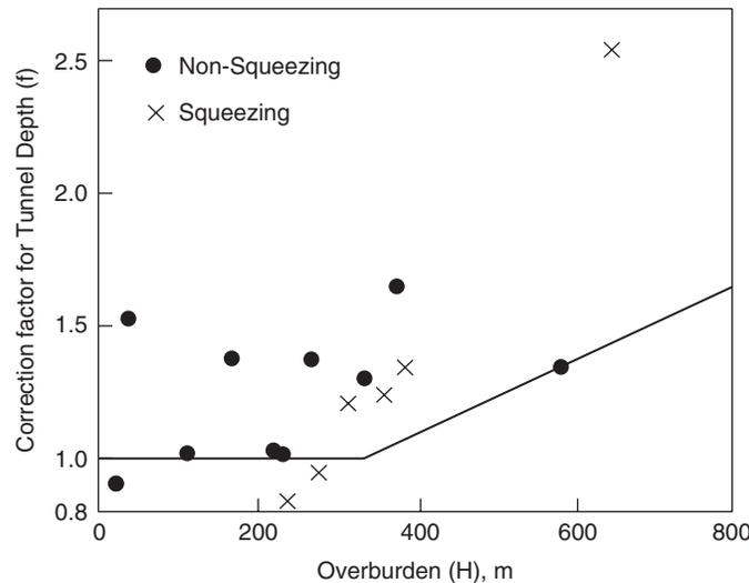
Fig. 5.3 Correction factor  $f$  for tunnel depth or overburden (Singh et al., 1992).
