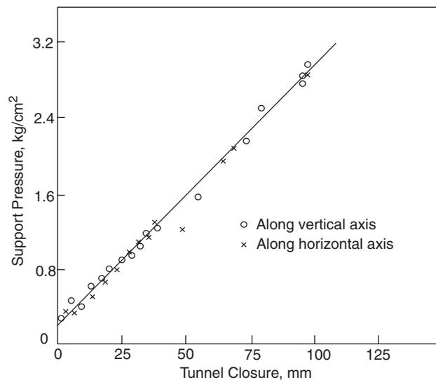
Fig. 14.7 Support pressure as a function of tunnel closure (observed by installing load cells in a support).
