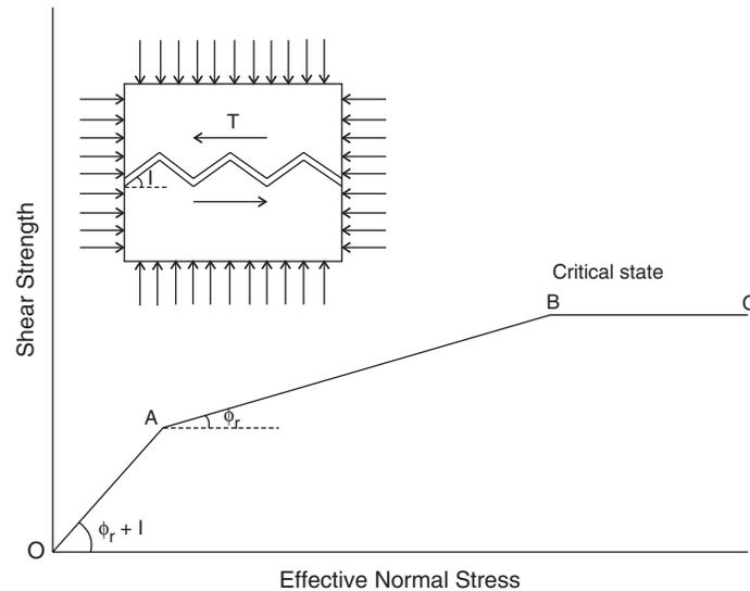
Fig. 7.5 Shear strength of discontinuities at very high confining pressure (OA – sliding above asperities, AB – shearing of rock asperities and BC – critical state of rock material at very high confining stress).
