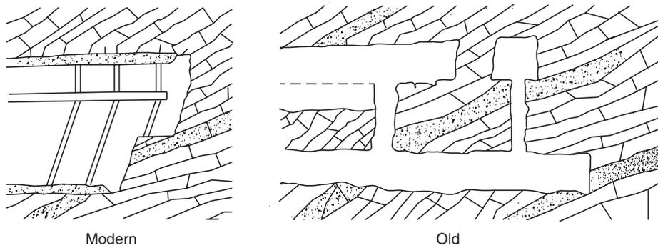
Fig. 9.14 Procedure of construction is important for safety of the structure. Variation of duration of a round, timing of support and ring closure, length of the crown and lining resistance are used to help the self-stabilization of the rock and the support.
