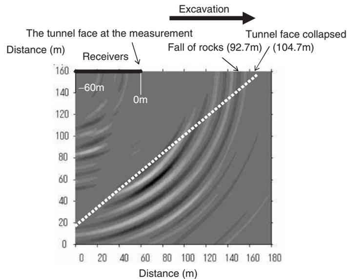
Fig. 2.15 A reflector image by the migration with the migration velocity of 4.5 km/s obtained from the seismic refraction analysis with a source at the tunnel face. A white broken line indicates the reflector that a stacking performance is maximum if velocity is 4.1 km/s. A tunnel face collapsed on the extension of clear reflector.
