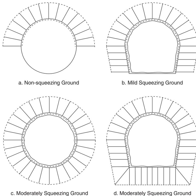
Fig. 28.19 Design philosophy of rock reinforcement in tunnelling.
