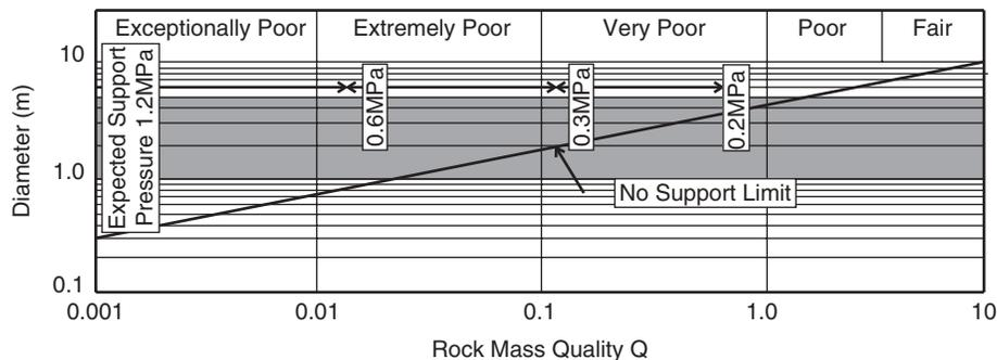
Fig. 24.3 Guide to estimate support pressures in vertical bored excavations (Golder Associates, 1976).
