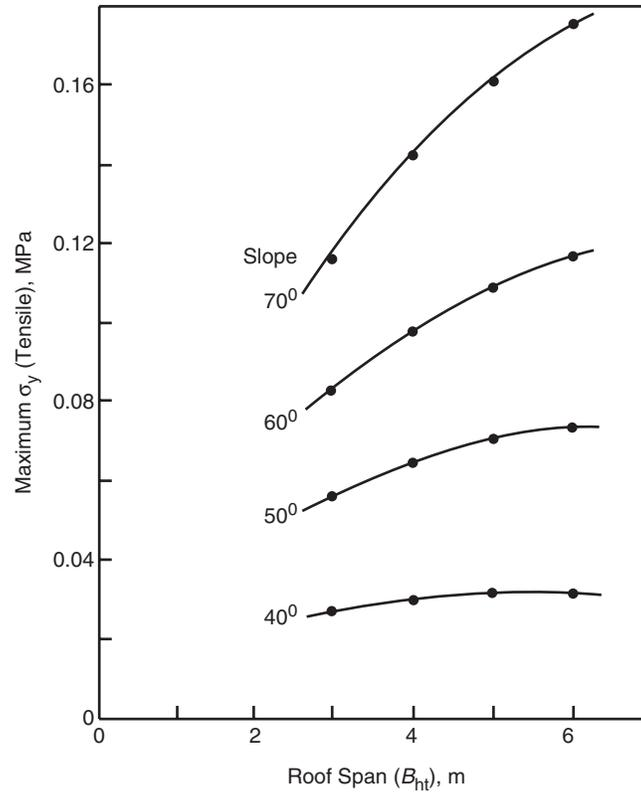
Fig. 25.4 Variation of maximum vertical tensile stress in roof with slope and span.
