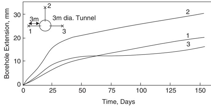
Fig. 14.8 Variation of borehole extension with time.
