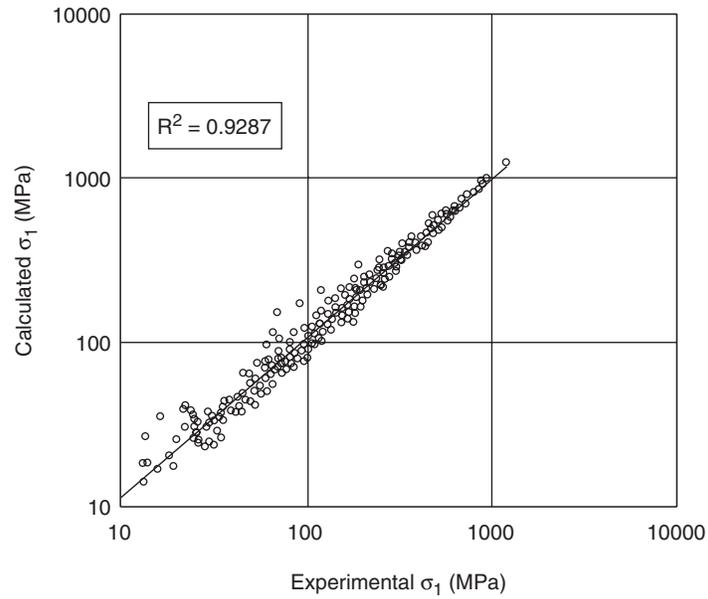
Fig. 29.3 Comparison of experimental  $\sigma_1$  values with those predicted using present criterion without using triaxial test data (Singh & Singh, 2005).
