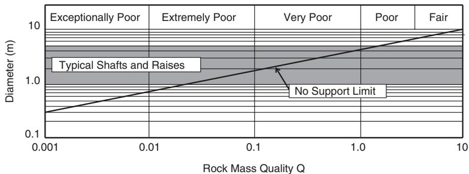
Fig. 24.2 No-support limit for vertical excavations adopted for wall conditions from Barton et al. (1974).
