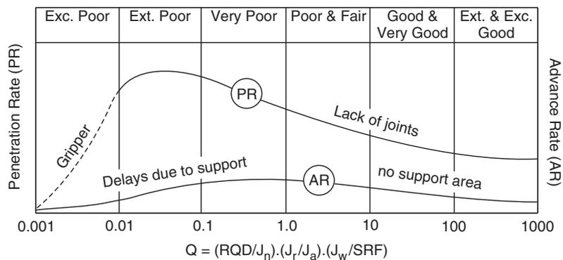
Fig. 16.1 A conceptual relation between  $Q$ , PR and AR.
