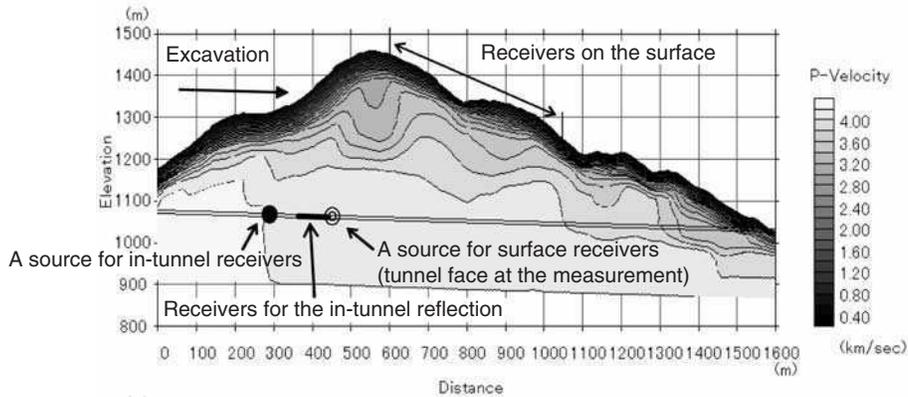
Fig. 2.10 A velocity model obtained from a refraction method carried out before construction and source and receiver location for data acquisition during the construction. A black thick line indicates receivers for the in-tunnel reflection method. ● Indicates a source for the in-tunnel reflection method. ⊙ Indicates a source for surface receivers.
