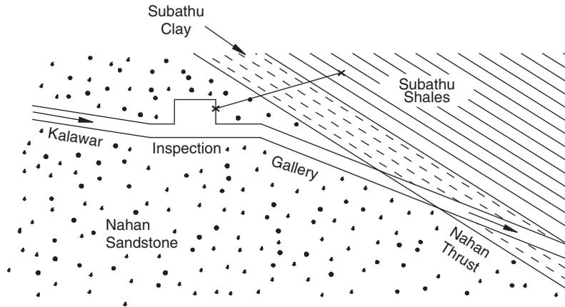
Fig. 20.5 Schematic arrangement for measuring displacement across the Nahan thrust by single-point borehole extensometer.
