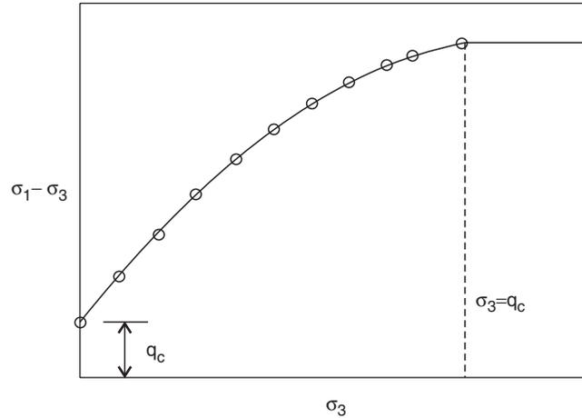
Fig. 29.1 Parabolic strength criterion.
