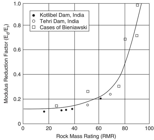
Fig. 4.2 Relationship between RMR and modulus reduction factor (Singh, 1979).
