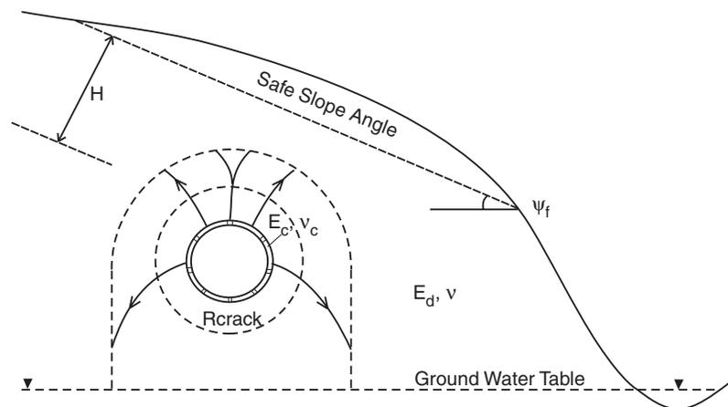
Fig. 23.1 Safe overburden above a pressure tunnel.
