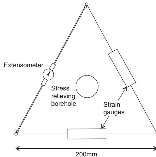
Fig. 14.2 Stress measurement at rock face by extensometers or strain gauges.
