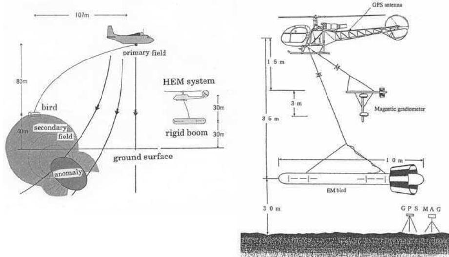
Fig. 2.4 Schematic map of helicopter-borne electromagnetic survey.
