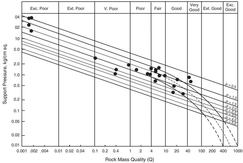
Fig. 5.2 Correlation between support pressure and rock mass quality Q (Barton et al., 1974).
