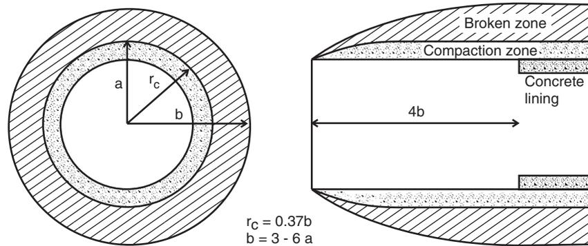
Fig. 19.3 Compaction zone within broken zone in the squeezing ground condition (Jethwa, 1981).
