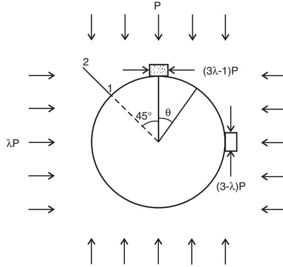
Fig. AI.1 Stress concentration around circular tunnel in non-hydrostatic state of in situ stress.
