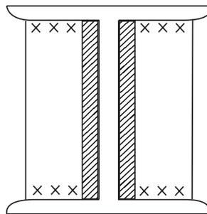
Fig. 28.12 Single beam wall plate.
