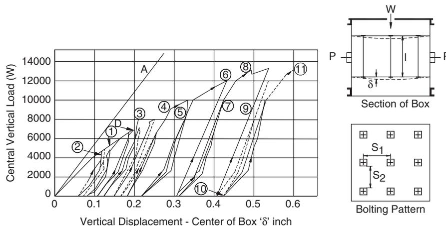
Fig. 12.10 Behavior of crushed rock model (Lang, 1961) [Rock size range was 1-1/2' to 2-1/4'; The mean ( $m$ ) was 1.875 inch ( $F = S_2/m = 4.3$ )].
