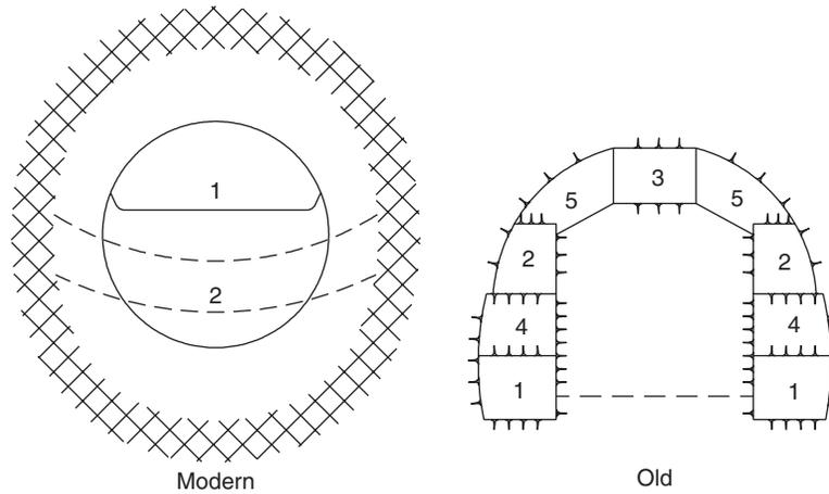
Fig. 9.13 Full-face heading helps to keep rock mass strength. Many partial headings reduce rock strength according to stress superposition.
