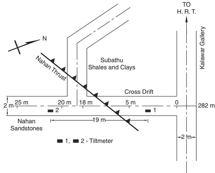
Fig. 20.4 Plan of tiltmeter bases for measuring tectonic movement along the Nahan thrust (Agrawal & Gaur, 1971).
