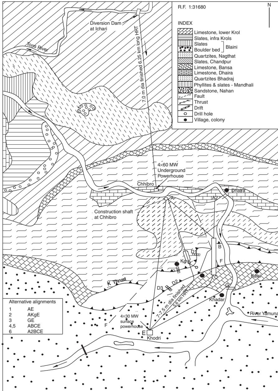
Fig. 20.1 Regional geology and alternative layout of the Yamuna hydroelectric scheme, stage II, part II.
