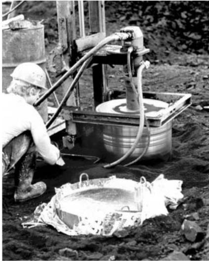
**Fig. 3.3.** Drilling of large core sample ( $\varnothing$  60 cm)
