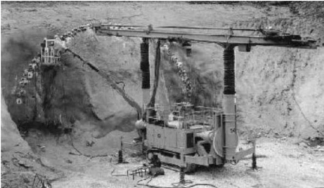
**Fig. 5.25.** Special forepoling rig, *Rotex*
