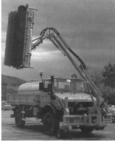
**Fig. 2.14.** Truck for tunnel washing<sup>46</sup>
