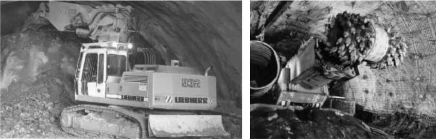
Fig. 4.12. Excavator<sup>7</sup>(left); Roadheader<sup>8</sup>(right)
