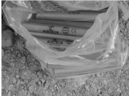
**Fig. 4.20.** Explosive cartridges
