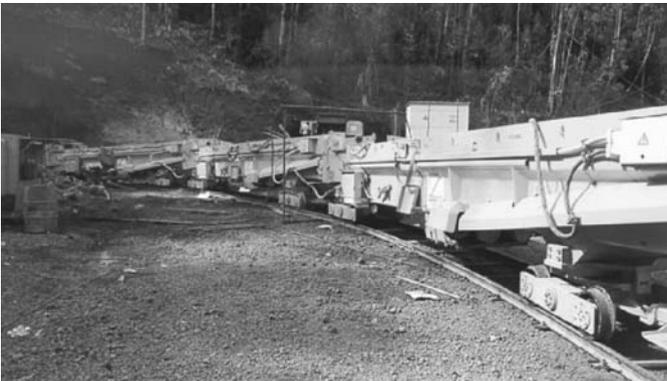
**Fig. 4.68.** Mucking with continuous conveyor<sup>63</sup>
