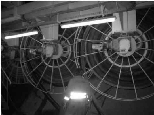
**Fig. 12.3.** Rolled cables for TBM power supply
