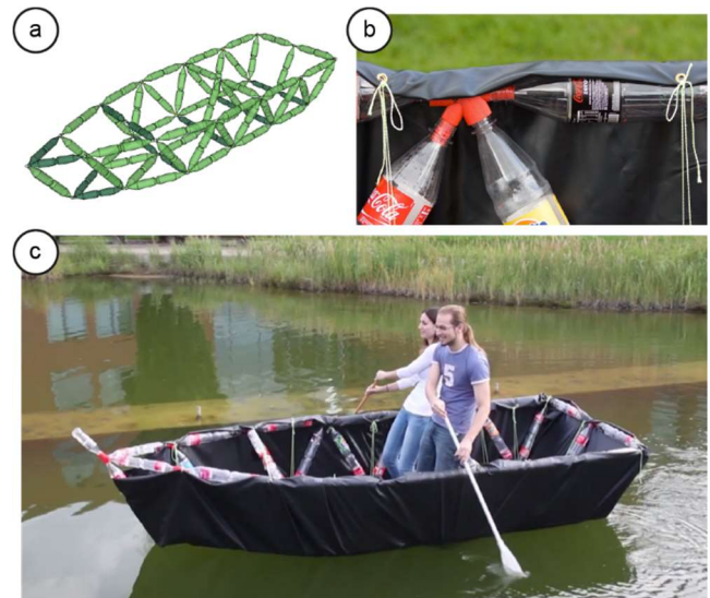
Figure 7: A functional boat created using TrussFab. (a) Using the editor, users can design their structures efficiently. (b) The bottle-frame is simply covered by tarp. (c) The fabricated boat seats two.
