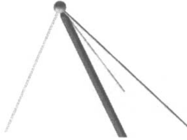
Figure 3.2 Necessary condition of spatial stability for a node
