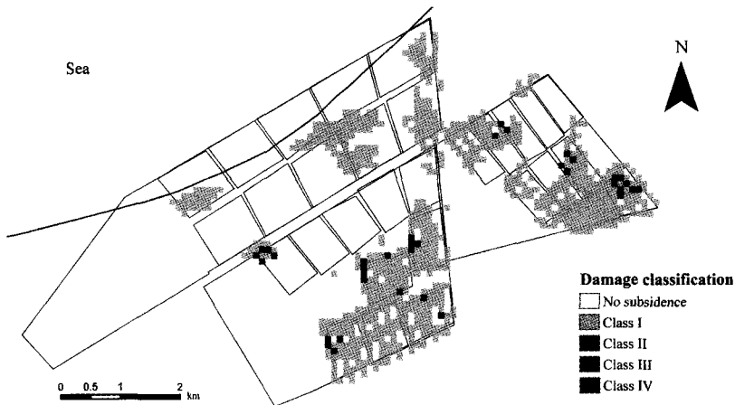
Fig. 1. Damage classification based on fuzzy model after mining.
