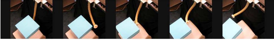
Figure 2.8: The continuum arm pushing a box resting on a surface
