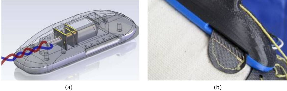
Figure 4.22: Twisted string actuators used to actuate the rolling flexure joints
