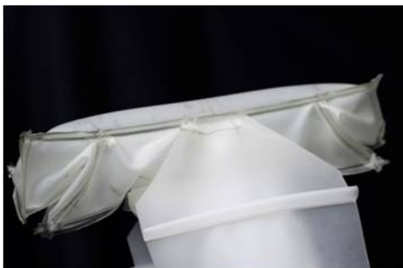
(a) The inflatable hand in its open state when volume with shape S_1 is inflated
