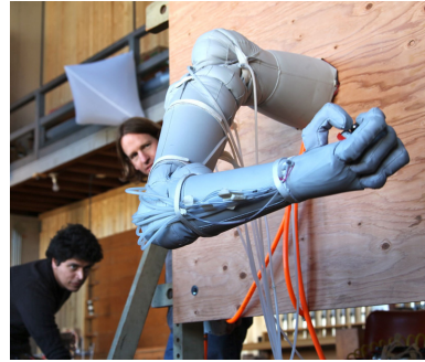
(b) Fabric-based inflatable arm with integrated compressive pneumatic actuators (work at Otherlab)
