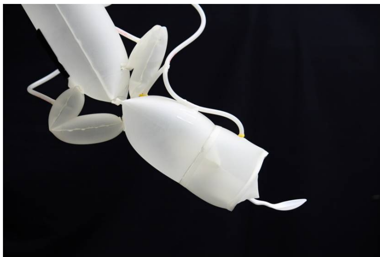
(b) Spoon affixed at end of the inflatable arm
