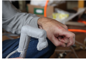
(b) Finger in closed state. In this state, the volume which has the shape of a closed finger is pressurized while the other volume is deflated.
