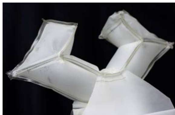
(b) The inflatable hand in its closed state when volume with shape S_2 is inflated
