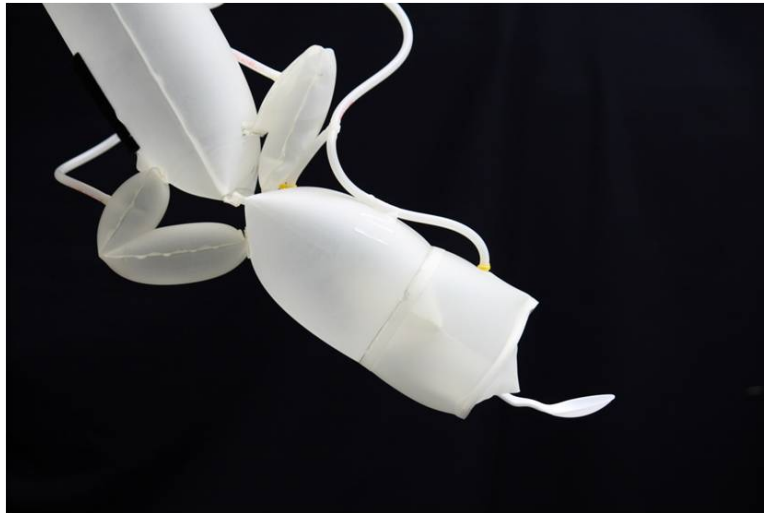
(b) Physical realization of the wrist and the variable stiffness actuator (IVSA)
