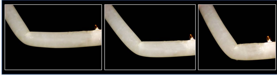
Figure 2.22: Variation in location of buckling site along an inflatable link
