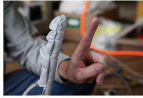
(a) Finger in open state. In this state, the volume which has the shape of an open finger is pressurized while the other volume is deflated.
