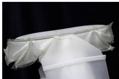
(b) Inflatable hand - open state
