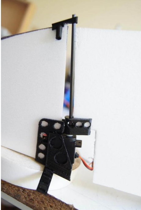
Figure 6 fin control setup of printed parts
