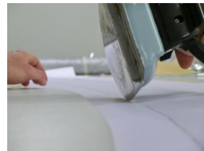
Figure 14 welding with an iron
