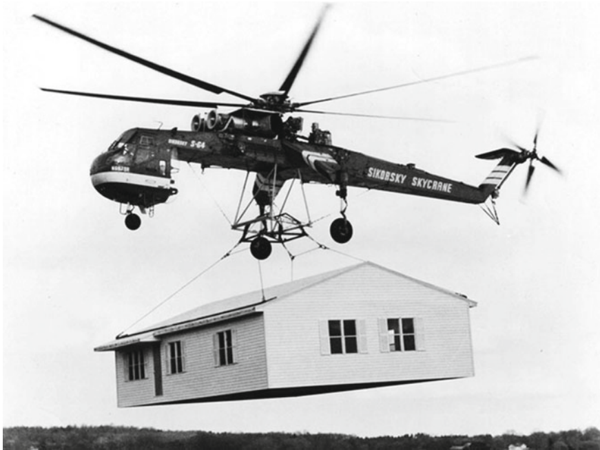
Fig. 3 A Sikorsky Skycrane carrying an accommodation
