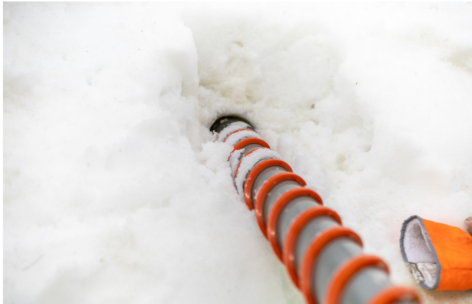
Image 27. Measuring snow density using an ice drill (Pernu 2022)
