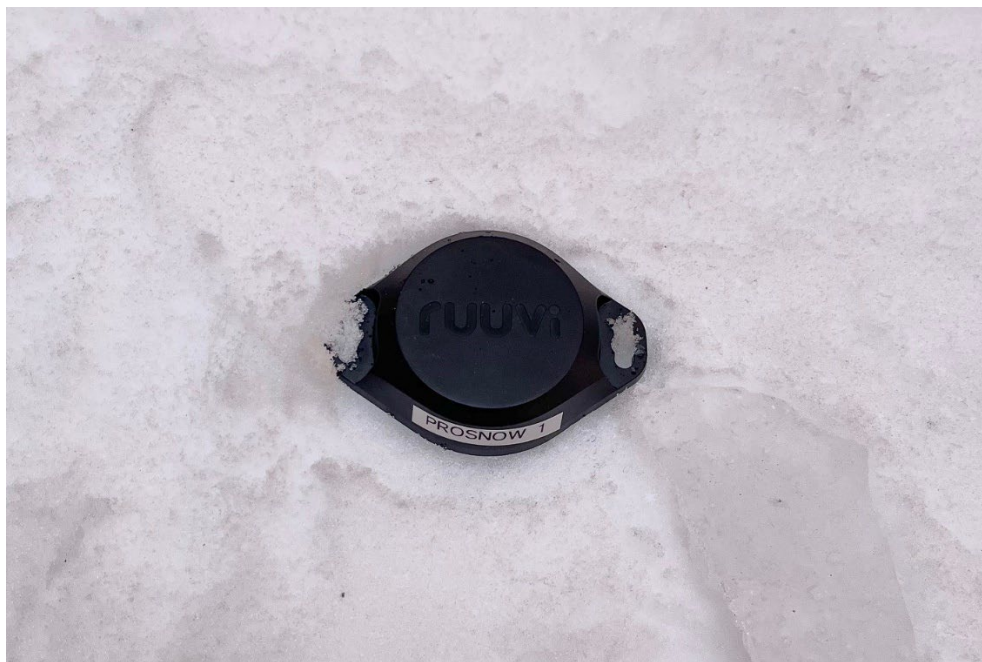
Image 26. A wireless temperature sensor for installation in a snow structure (Pernu 2025)
