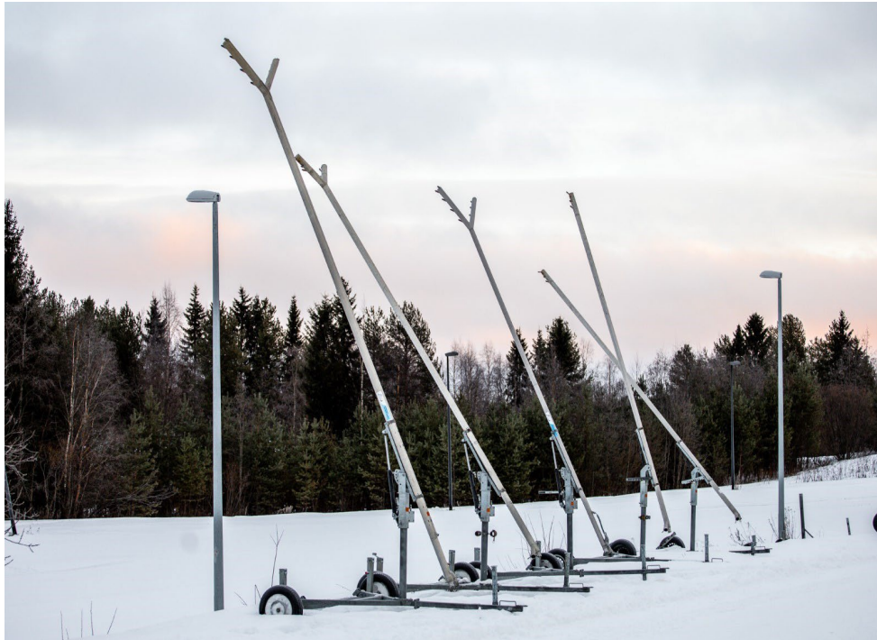
Image 19. A high-pressure lance suitable for direct blowing in Ounasvaara (Pernu 2025)
