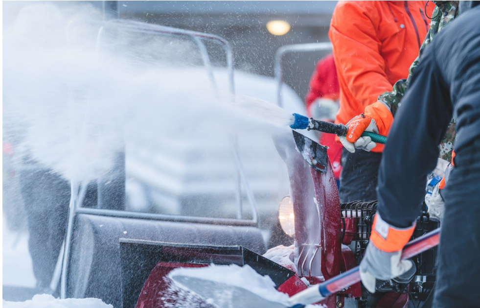
Image 18. Spraying water during the snow blowing phase (Pernu 2022)
