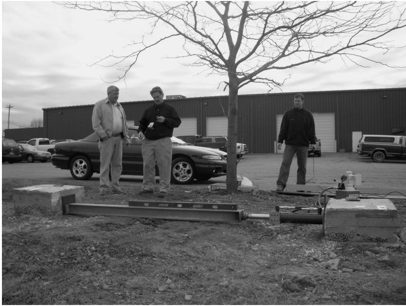
Figure 10.12 Lateral load test on concrete pile caps formed over helical piles (Courtesy of Magnum Piering, Inc.)
