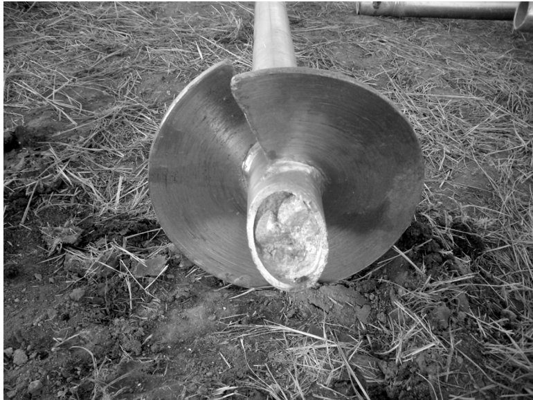
Figure 4.12 Plugged end of a typical helical pile
