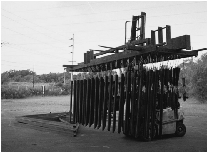
Figure 11.8 Helical piles ready for galvanizing
