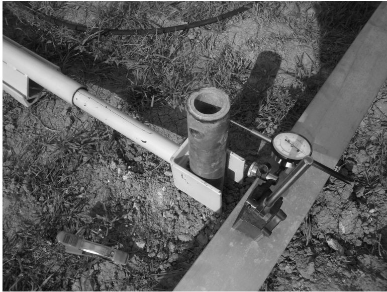
Figure 10.11 Dial gage used to measure lateral displacements
