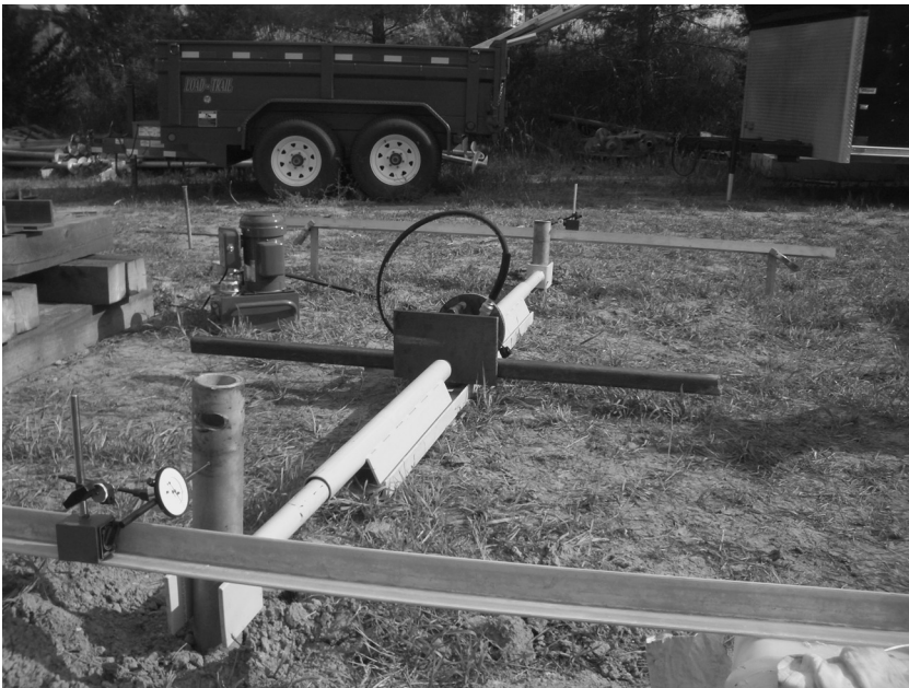
Figure 10.10 Lateral load testing on helical piles by pushing apart (Courtesy of CTL|Thompson, Inc.)
