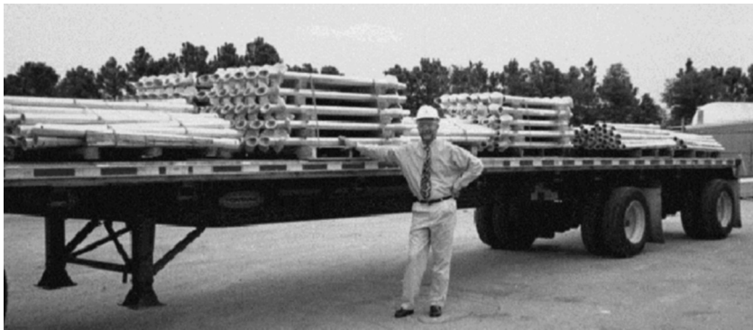
Figure 11.9 Galvanized piles ready for shipment
