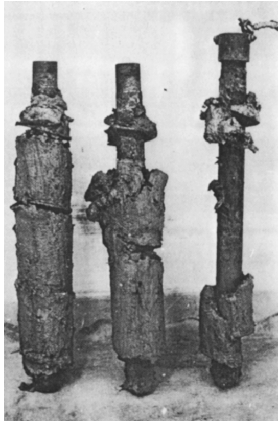
Figure 5.1 Model helical anchors with different inter-helix spacing ratios (Narasimha Rao et al. 1989)
