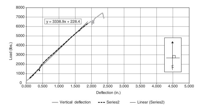
Figure 7-6. Typical response for an axially loaded anchor.
