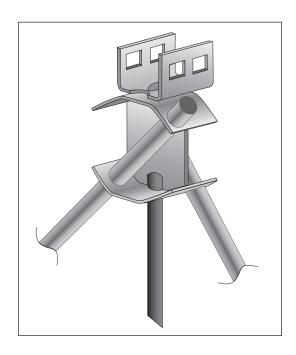
Figure 7-1. Cross drive anchor. (Courtesy of Tie Down Engineering)
