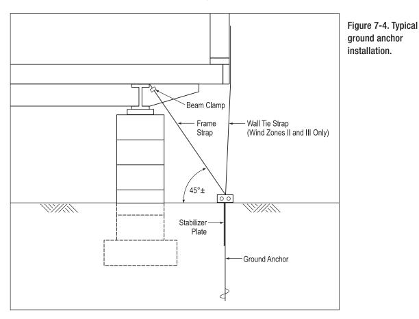
When fastened as vertical wall ties and loaded axially, ground anchors may be used without stabilizer plates. When ground anchors are used with some proprietary foundation systems, anchors can be installed 45 degrees to the horizontal and loaded axially (Figure 7-5).
