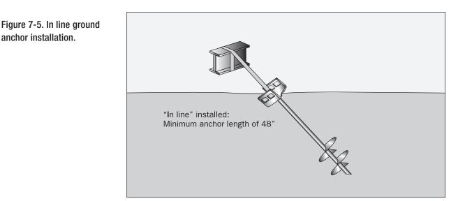
Failure occurs when the stresses exceed the soil shear strength. The geometry of the failure surface varies based on the critical depth of the anchor. Ground anchors with an embedment depth less than the critical depth to anchor base width ratio  $((D/B)_{cr})$  respond as a shallow foundation. Ground anchors with a depth greater than  $(D/B)_{cr}$  respond as a deep foundation.
