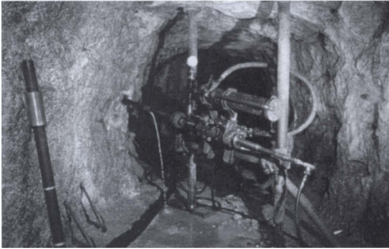
Figure 4.2 In situ stress determination in the Carmenellis granite.
