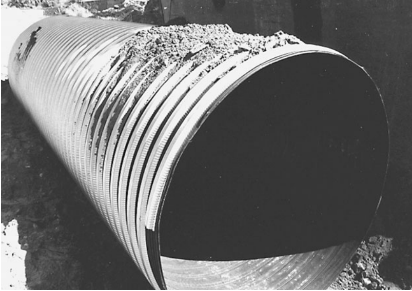
Figure 7.45 Test pipe being placed in test cell.
