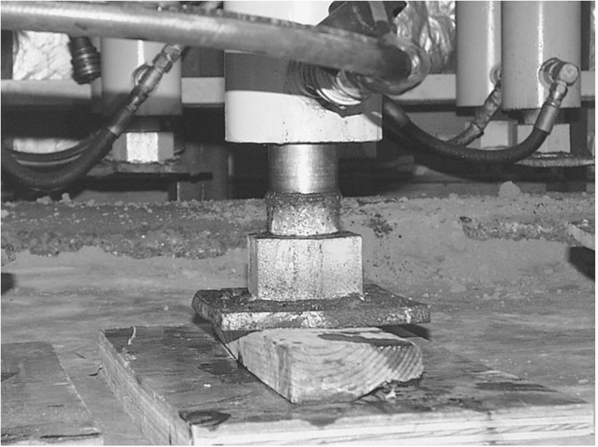
Figure 6.31 Photograph showing 16,000-lb load being applied to a 10-in \times 20-in plate over one-half of the pipe.
