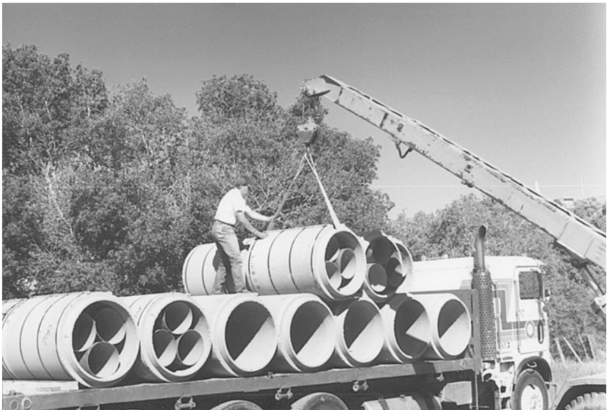
Figure 8.3 Broken rigid pipe after breaking in three-edge-bearing device. Broken pipes have paper sonotubes inside and are steel-banded on the outside to hold broken segments together.
