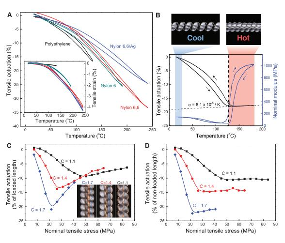
(C) when normalized to the initial nonloaded muscle length, indicating that the absolute displacement during actuation remains nearly constant at loads above those at which coils contact.
