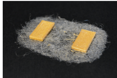
Figure 2: A simple hinge fabricated with our 3D printer using rigid plastic printing and melt electrospinning on the same extruder.
