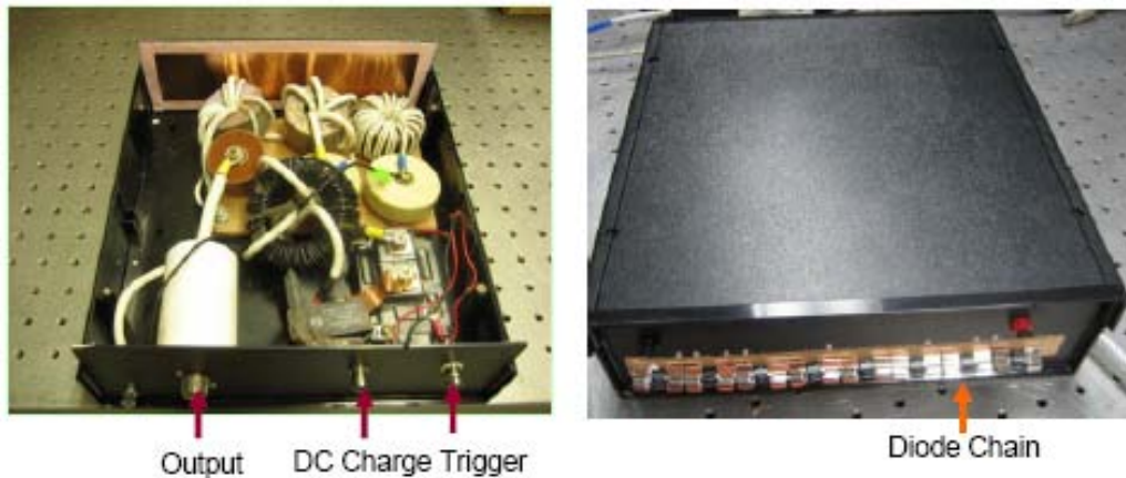
Figure 4.12 Prototype of the pulse generator, a “plug in” diode testing interface is designed as shown in the right hand graph.
