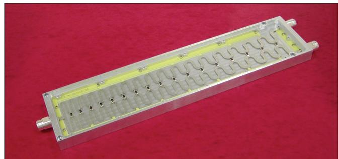
Figure 3. Ultrawideband 70 MHz to 2700 MHz Wilkinson divider/combiner using 17 sections with an air dielectric for minimum loss.
