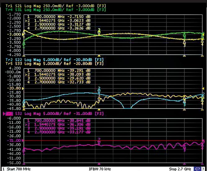
Figure 6. Hybrid coupler's typical characteristics for coupling (top), return loss (center) and isolation (bottom).
