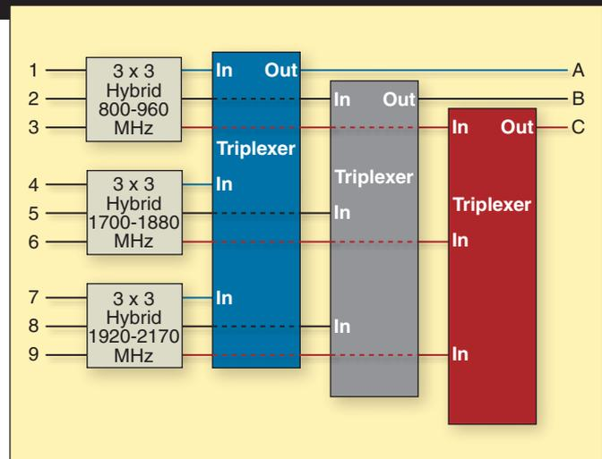
Figure 10. Lossless combining of nine inputs to three distributed antenna feeds, as might be used in an in-building system.
