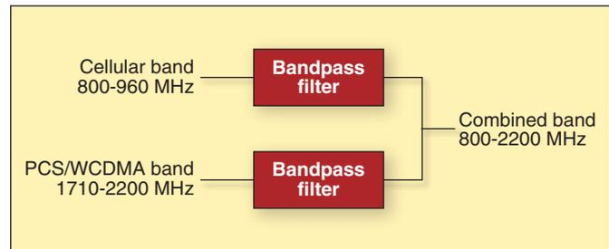
Figure 1. A typical two-input diplexer filter system.
