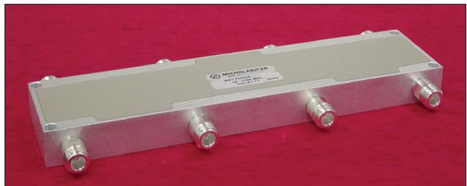
Figure 7. Simple four-input, two-output multiband 700 MHz to 2700 MHz combining matrix using three hybrid couplers and two external loads.
