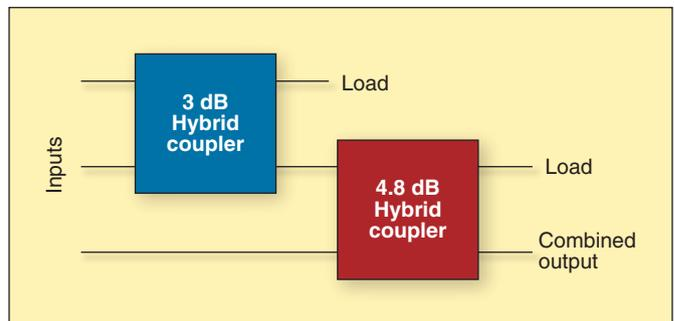
Figure 8. Schematic of a 3:1 hybrid combiner with 4.8 dB loss in each signal path.
